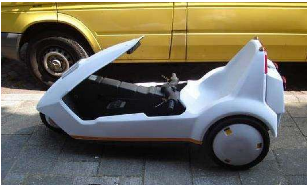
The Sinclair C5 pedal-assisted battery vehicle.
