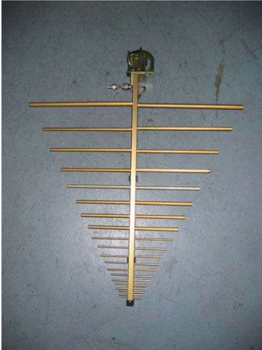
Log-periodic dipole array
