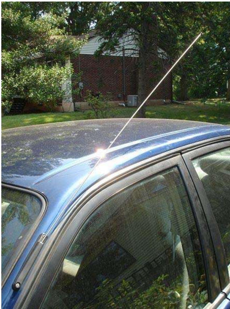
Whip antenna on car
