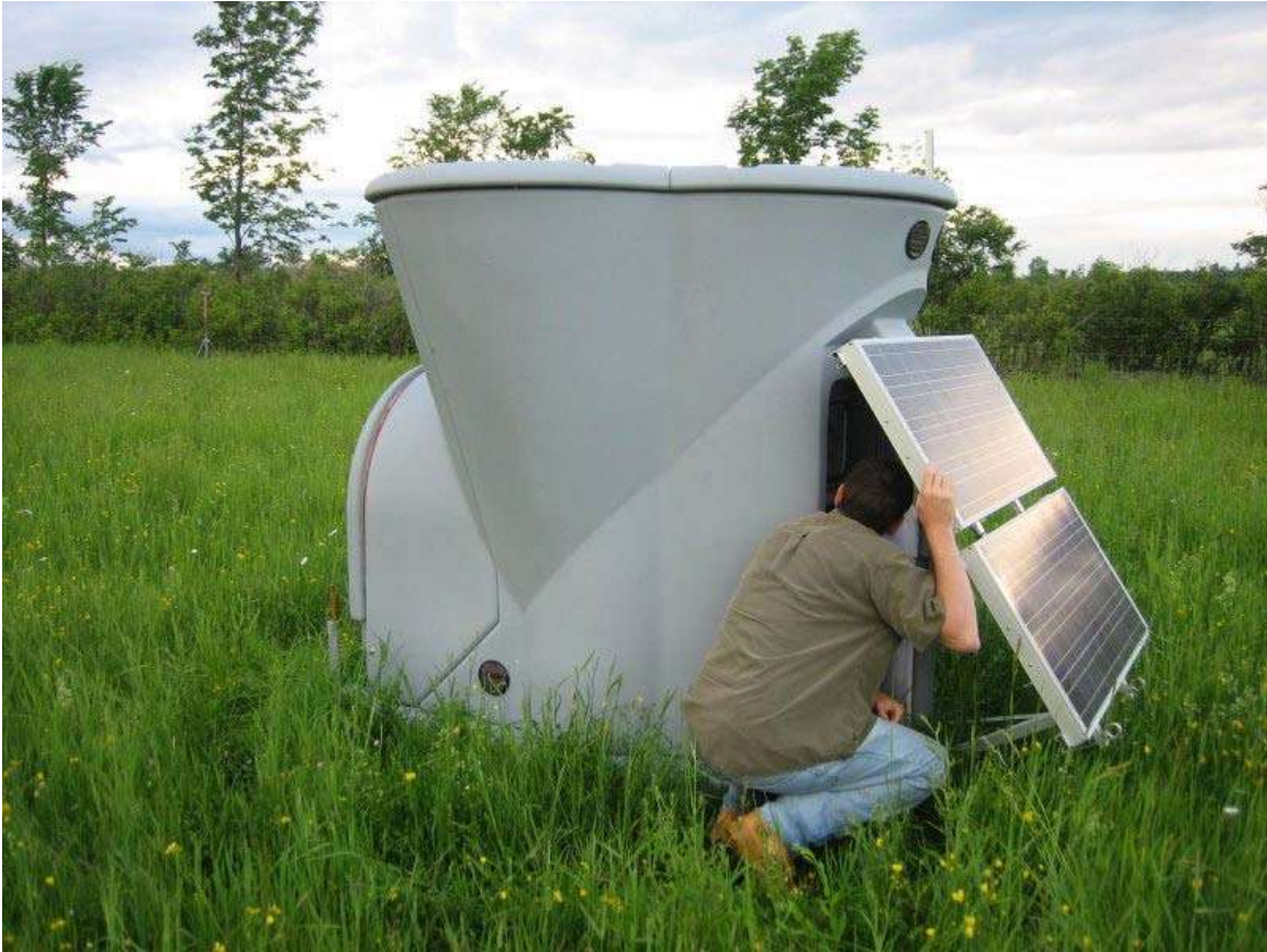
The TRITON transportable SODAR system used to measure wind profiles from Second Wind.
