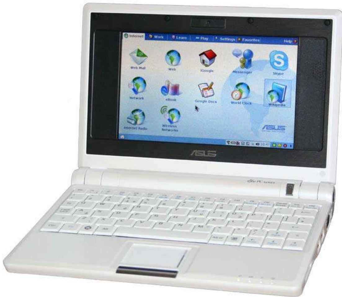
An ASUS Eee PC 700, the first mass-produced netbook, used a 7 inch screen.
