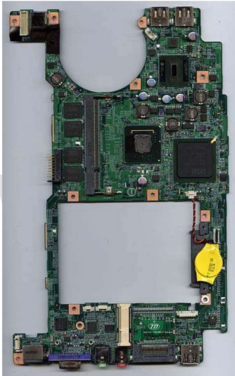
An MSI Wind netbook motherboard featuring the Intel Atom processor
