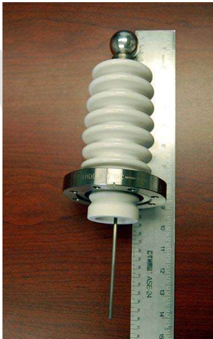
A 60 kV high voltage electrical feedthrough on a 4-1/2 inch (or DN63) conflat flange
