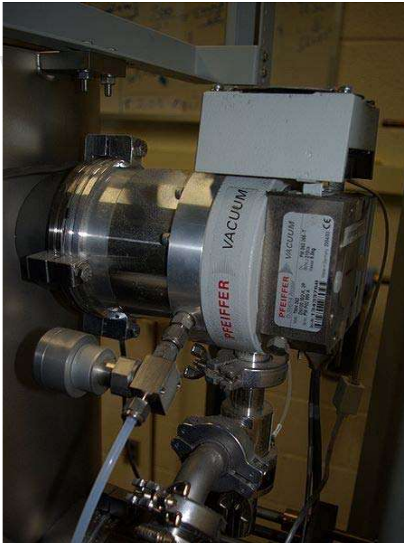
A turbopump by Pfeiffer attached to a thin film deposition system for organic electronics research
