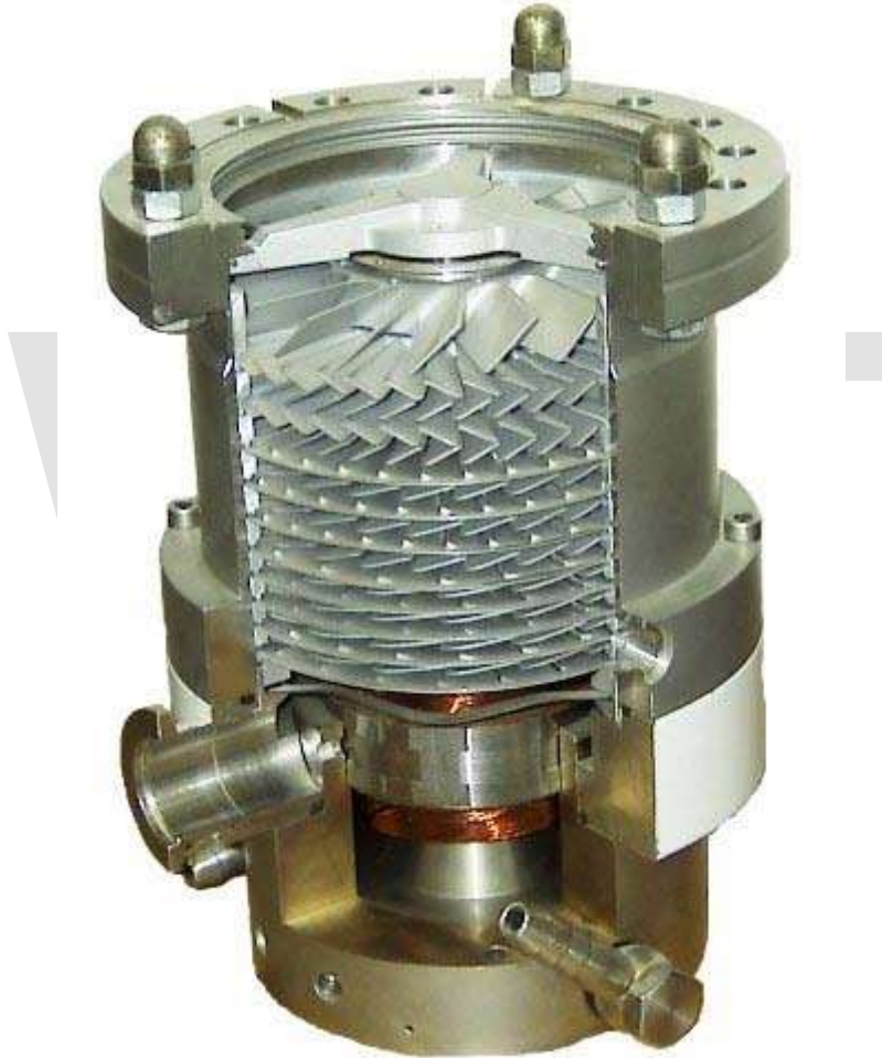
Interior view of a turbomolecular pump
