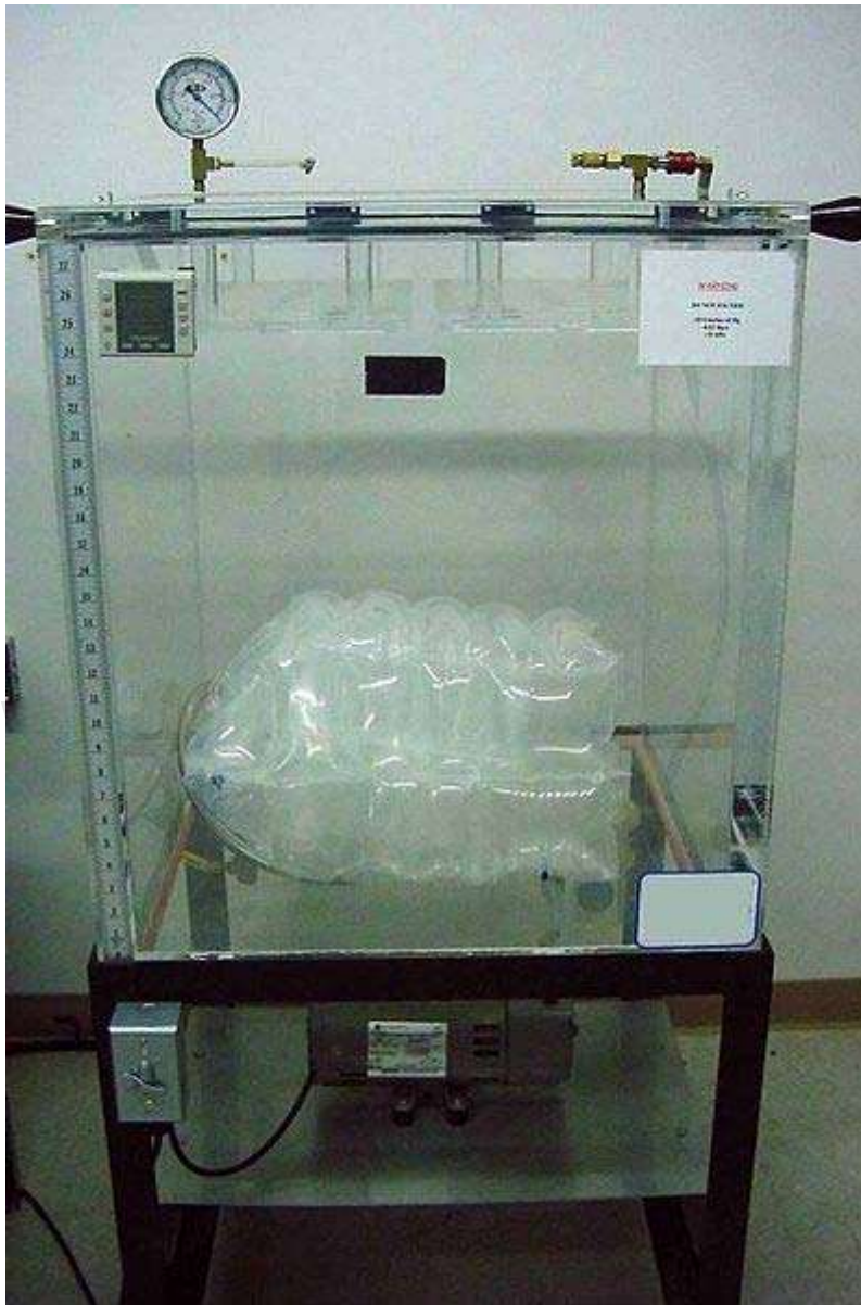
Vacuum chamber for testing leaks in packaging
