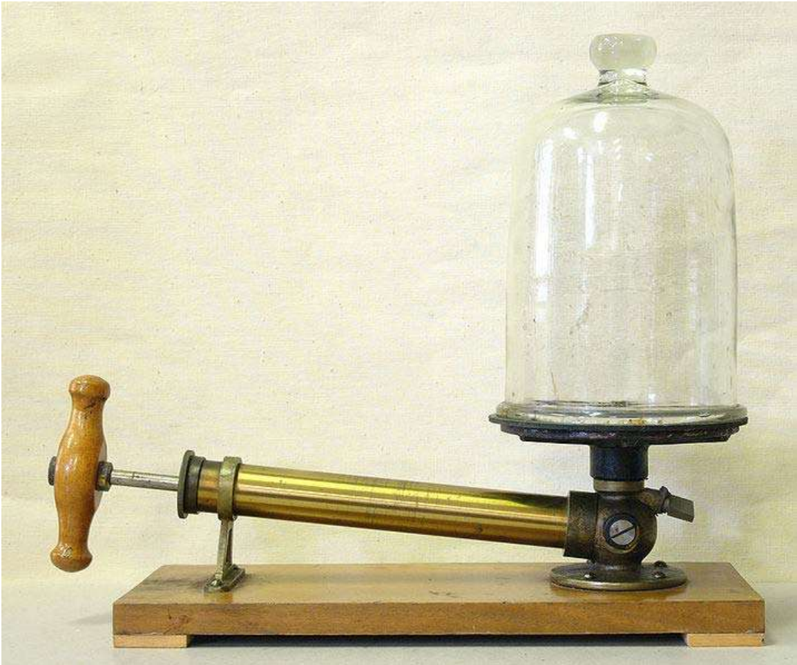
Pump to demonstrate vacuum
