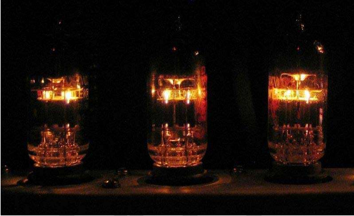
Russian 12AX7 tubes inside a modern guitar amplifier
