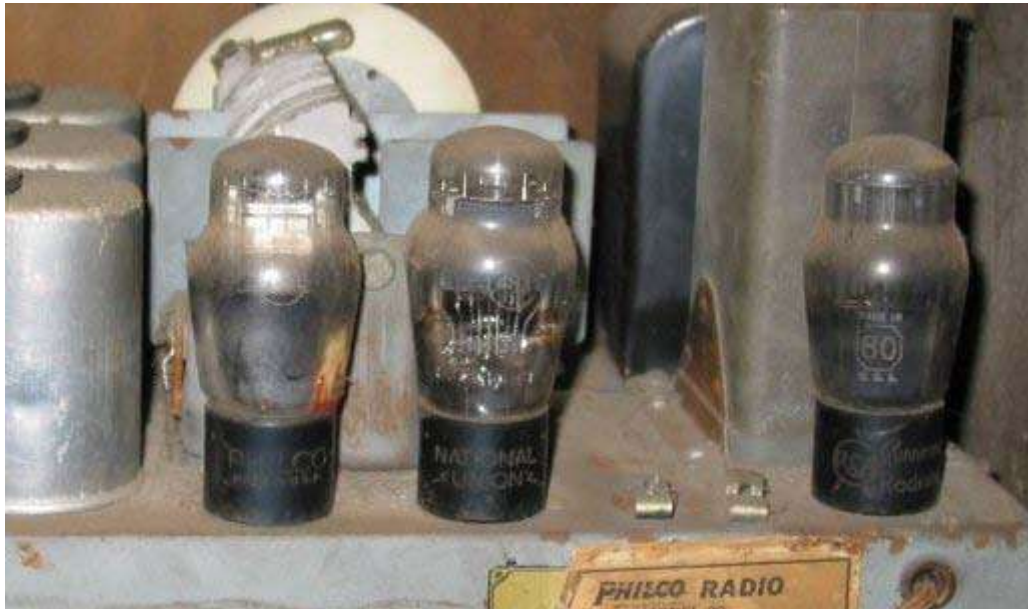
Vacuum tubes in an Australian radio of the late 1930s
