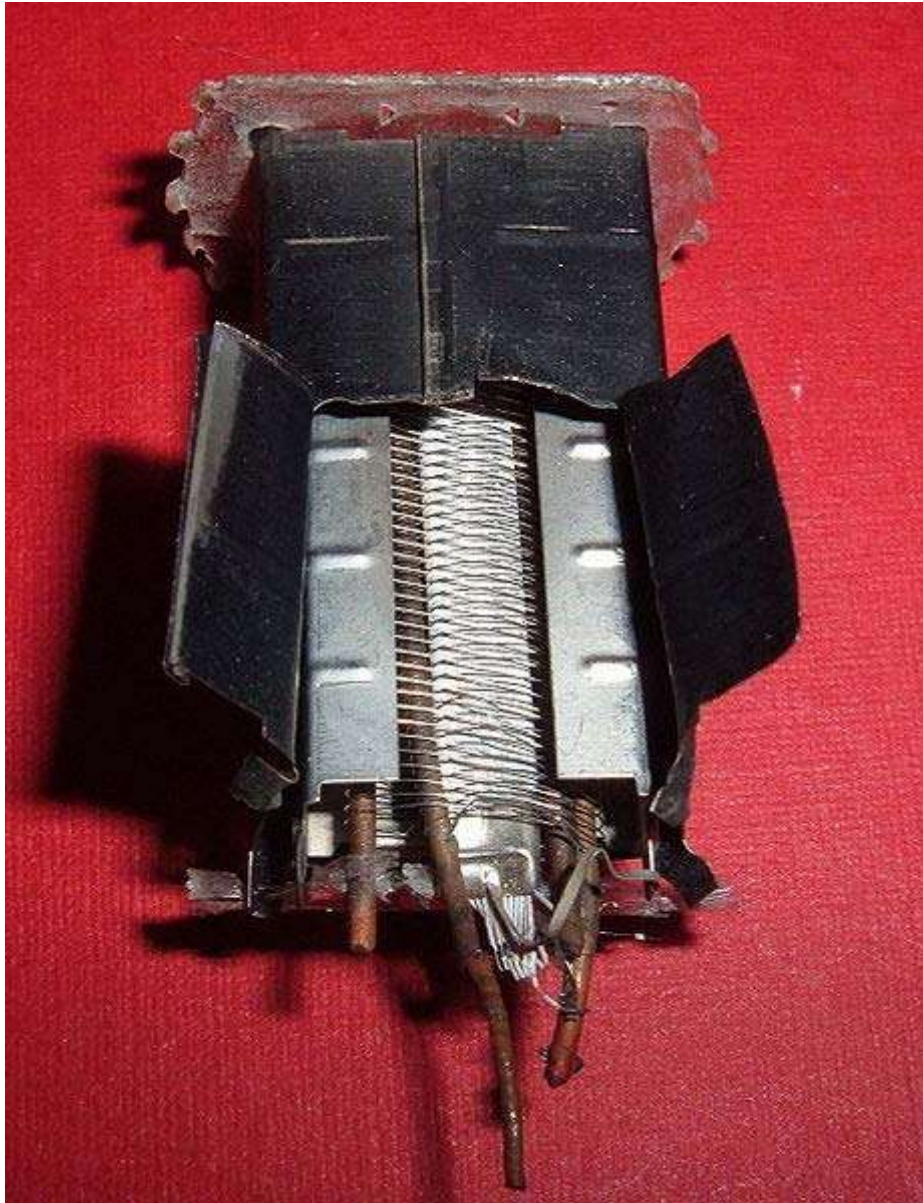
Inside of a vacuum tube with plate cut open
