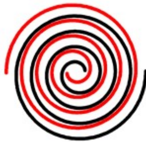
Mechanism of a scroll pump
