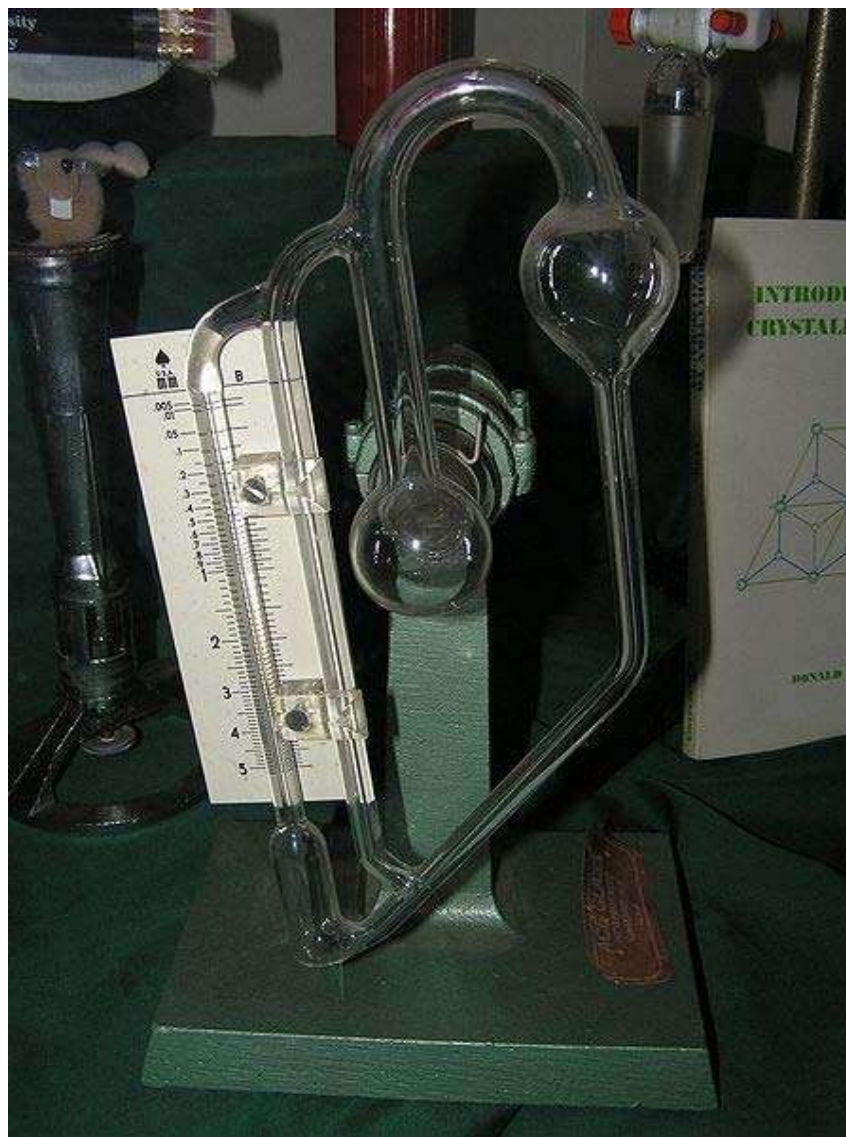
A McLeod gauge, drained of mercury
