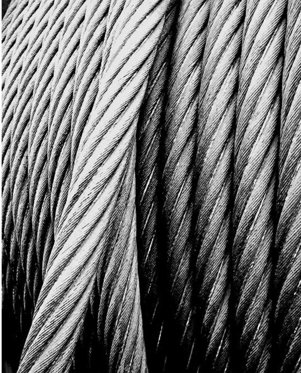
The steel cable of a colliery winding tower
