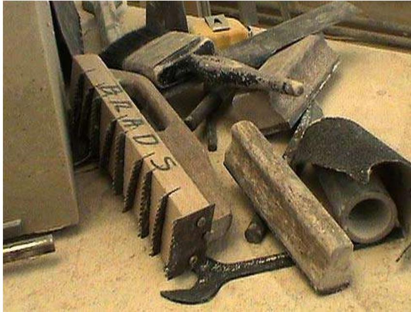
The foreground tool with serrated blades is a cockscomb, cock's comb or stonemason's drag, used on soft limestone
