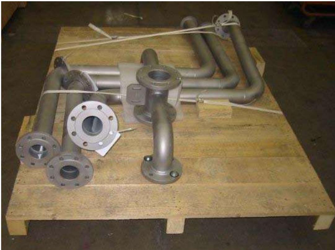
Pipes and fittings made of stainless steel
