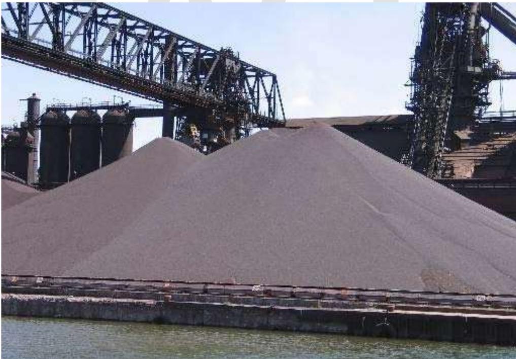
Iron ore pellets for the production of steel
