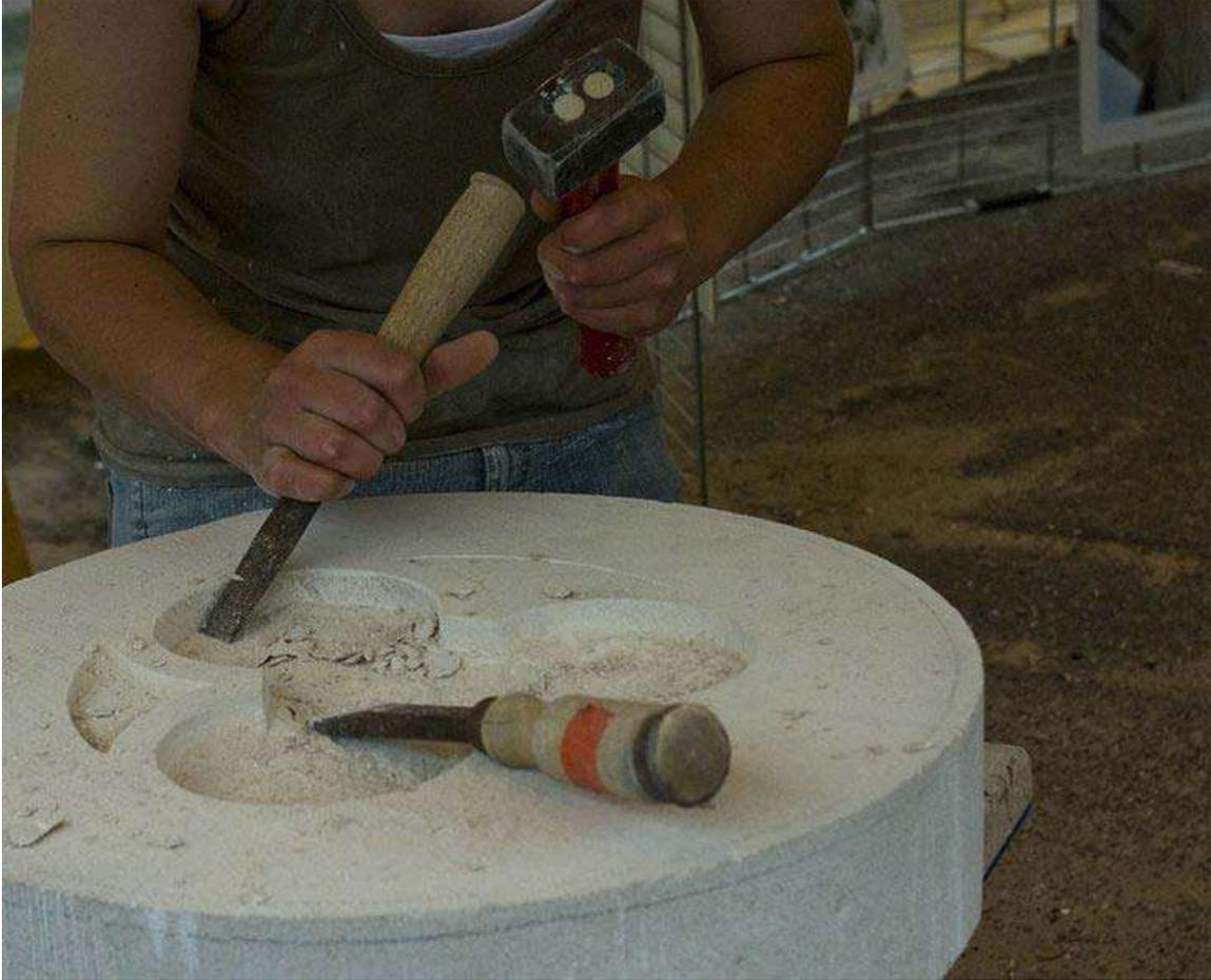
Typical French chisels with wooden hilt, used for soft limestone
