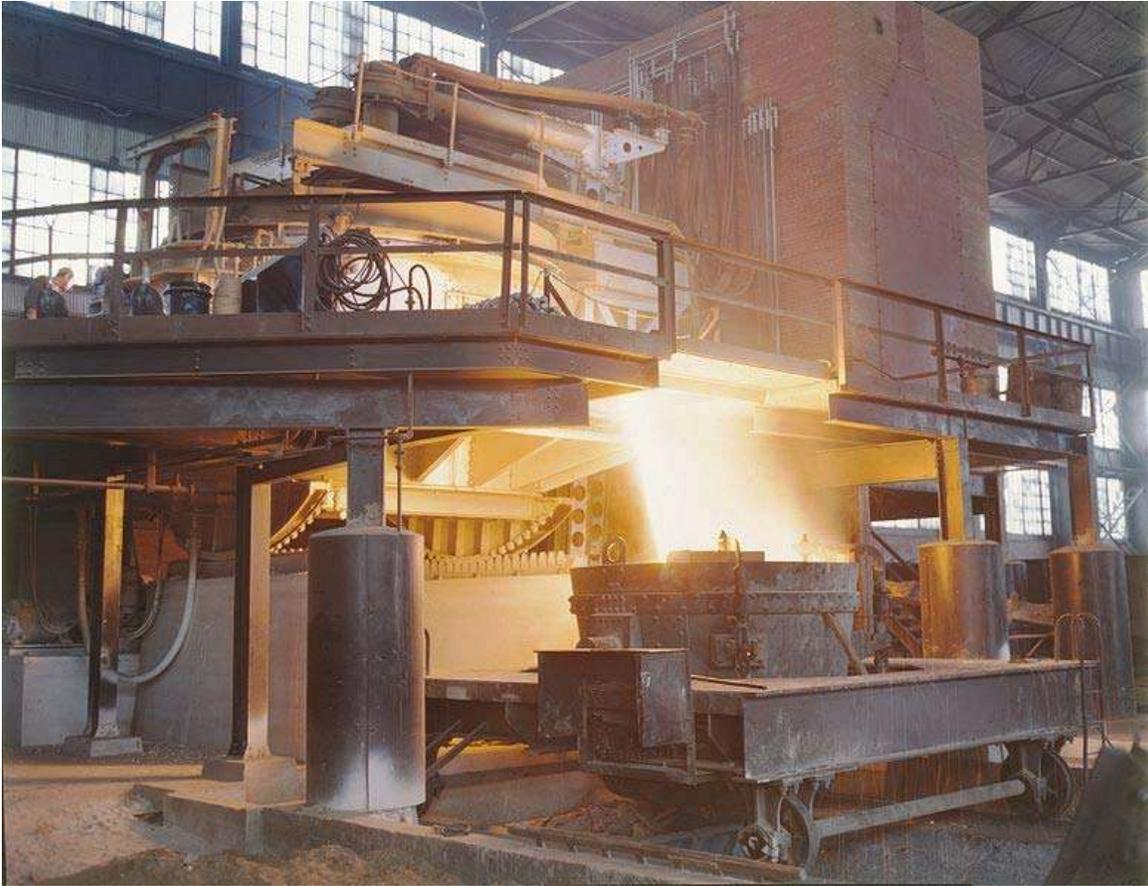
White-hot steel pouring out of an electric arc furnace
