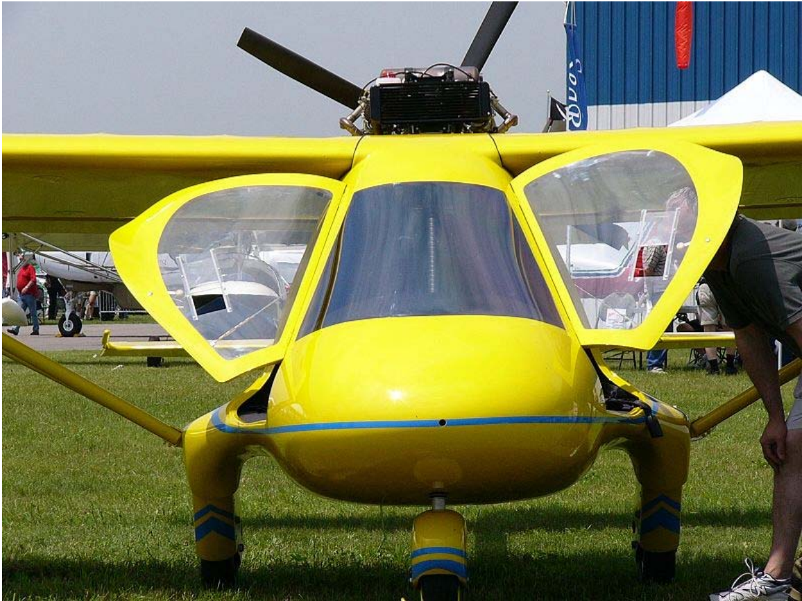
Interplane Skyboy - front view showing the unusual main landing gear
