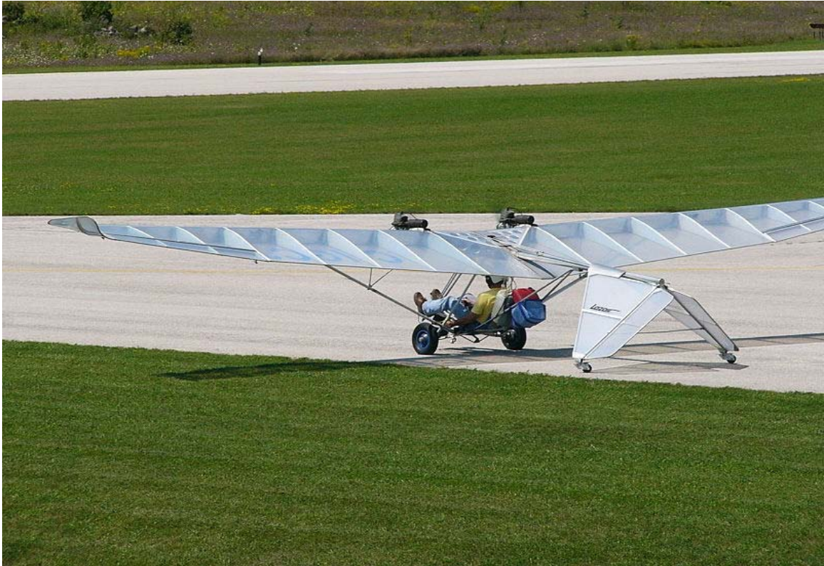
Canadian Lazair ultralight covered in clear Mylar
