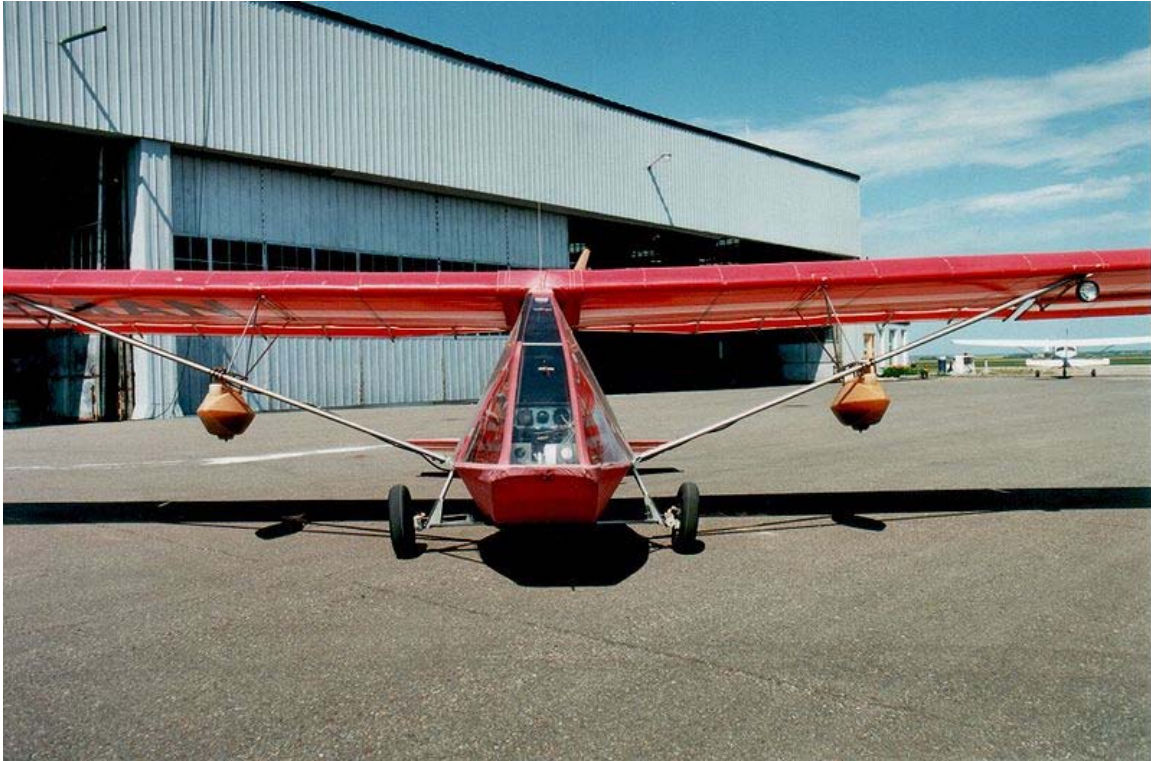
Birdman Chinook 2S showing the pentagonal cockpit cross-section
