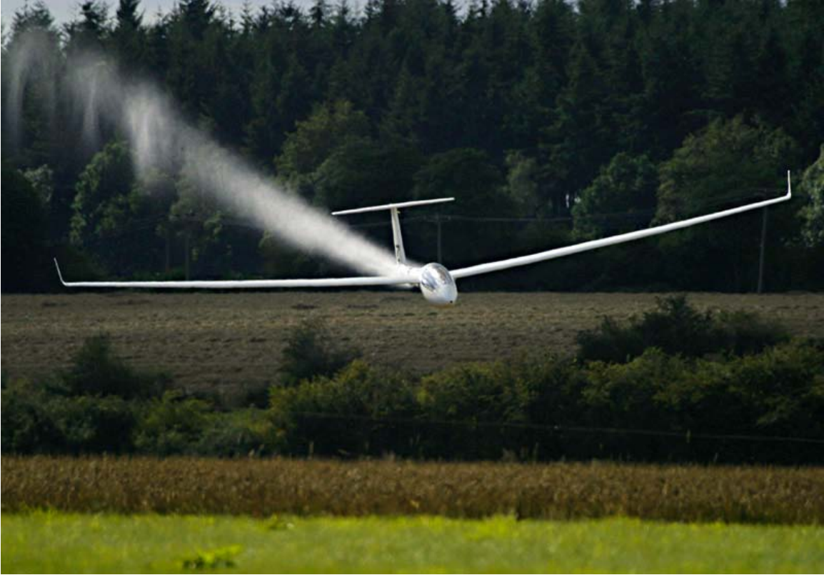
A glider releasing its water ballast
