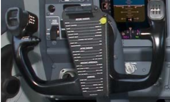
The "W" shaped control yoke of a Boeing 737.
