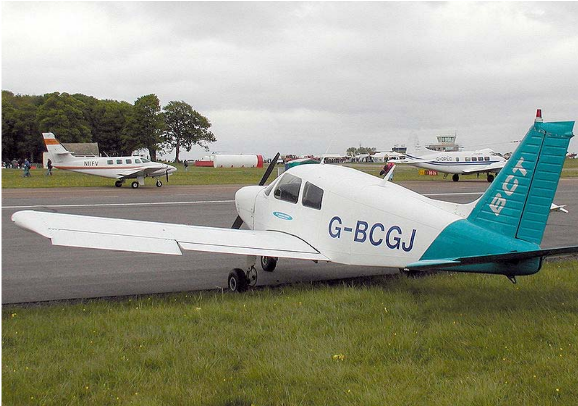
Piper Cherokee with stabilator (and anti-servo tab) deflected upwards
