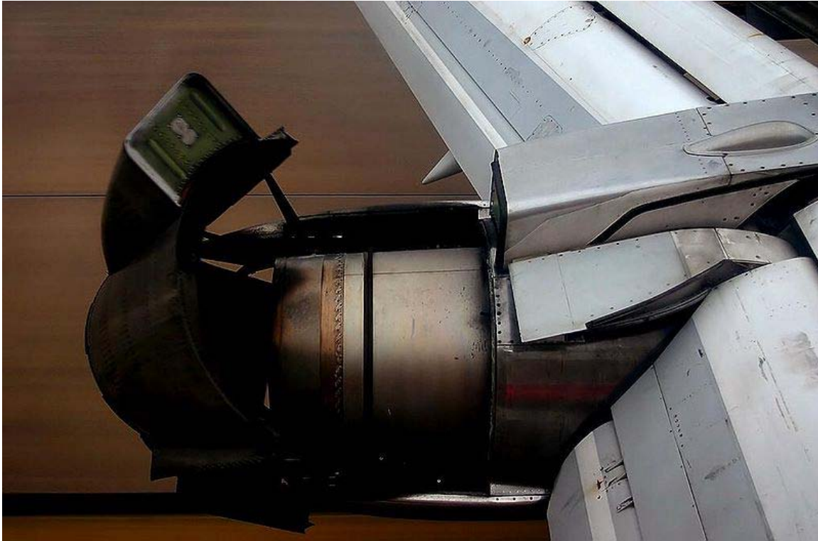
Thrust reverser deployed on the Pratt & Whitney JT8D-7 turbofan engine of an Aloha Airlines Boeing 737-200 landing at Honolulu, HI
