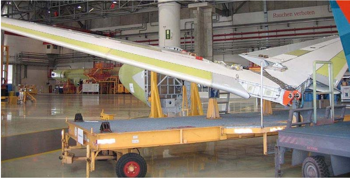
Pre-installed elevators for a small Airbus. The elevator is the silver surface on the right hand side of the picture, immediately below the red pipes on the factory wall
