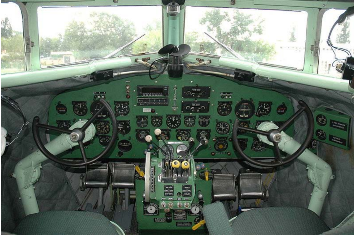
Circular, steering-wheel type yoke in a 1940's Lisunov Li-2
