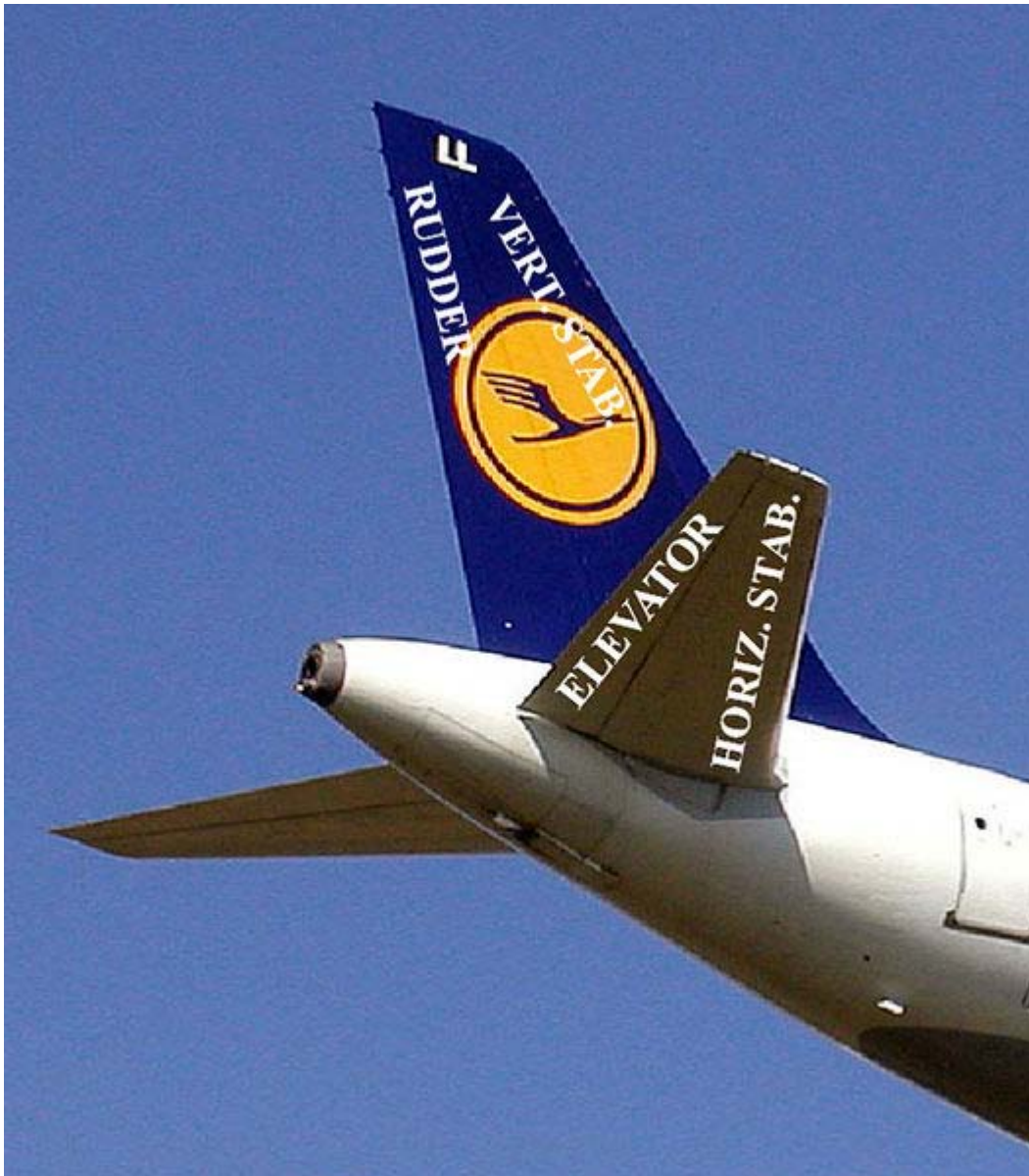
The tail of a Lufthansa Airbus A319 in flight, showing the elevator (Stab. means Stabiliser)
