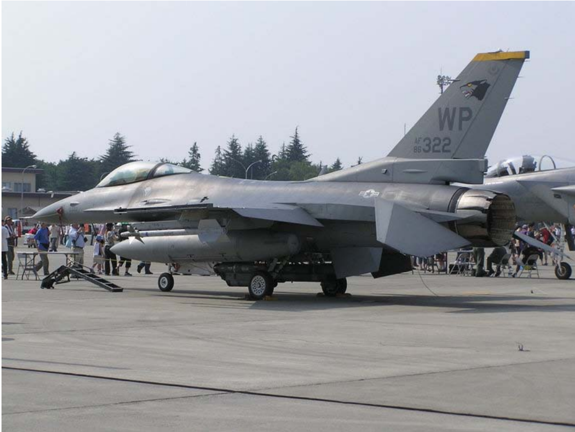
F-16 Falcon fighter jet parked at an airshow, with stabilators deflected downwards
