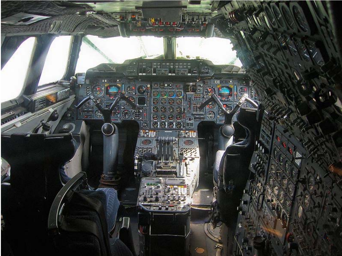
The cockpit of Concorde, which has an "M" shaped yoke mounted on a control column
