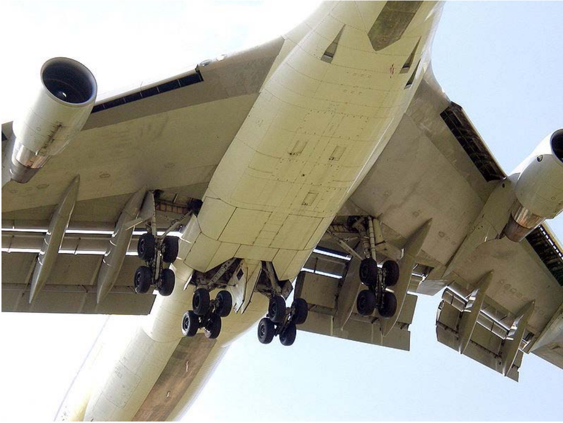
Triple-slotted trailing-edge flaps and leading edge Krueger (unslotted and slotted) flaps fully extended on a Boeing 747 for landing.
