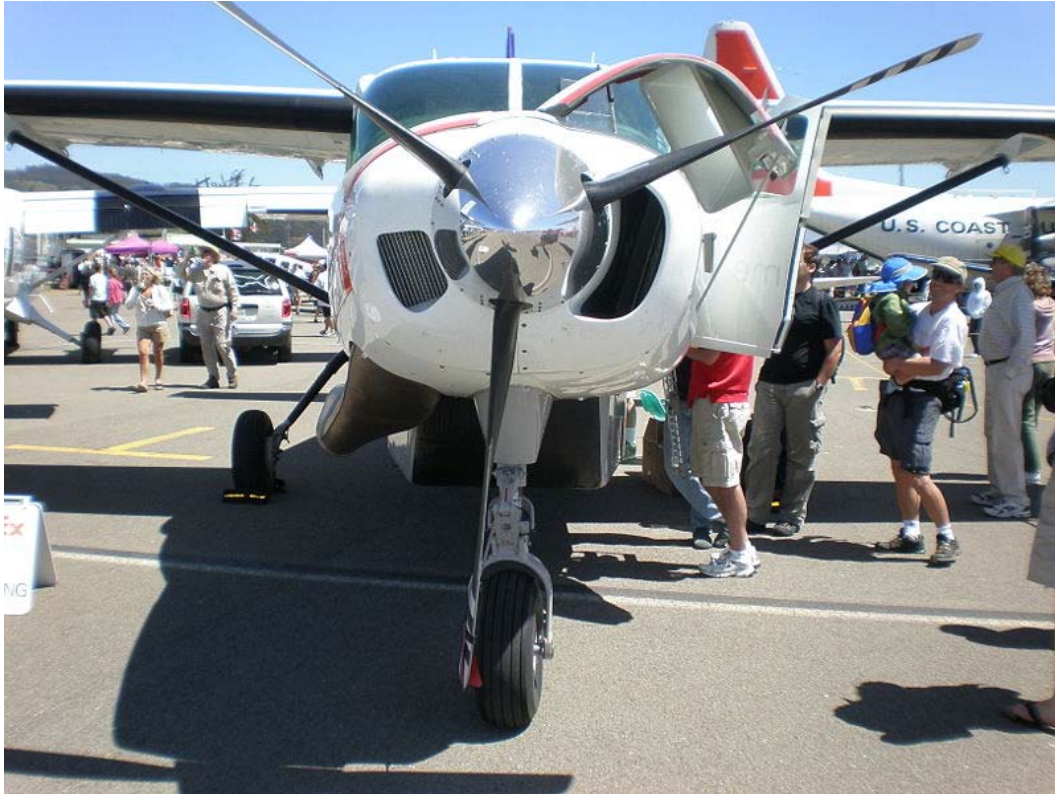
Controllable pitch propeller on the single-turboprop of a FedEx Cessna 208B Grand Caravan
