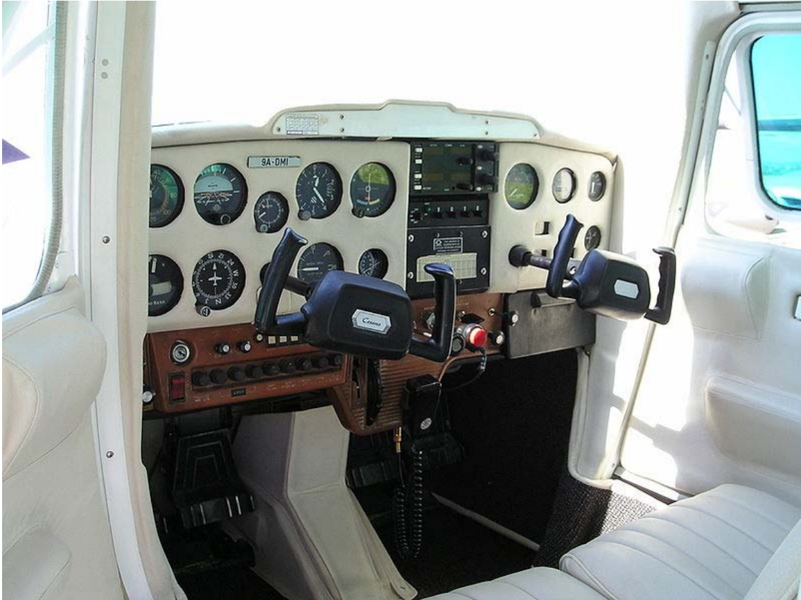
"W"/"U" style yoke in a Cessna 152 light aircraft, mounted on a horizontal tube protruding from the instrumental panel.
