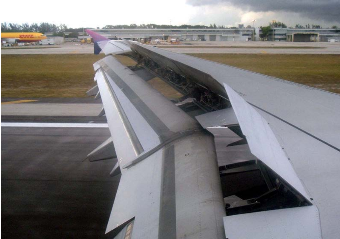
A close look at the spoiler (the parts of the wing that are raised up) during the landing of an Airbus A321.
