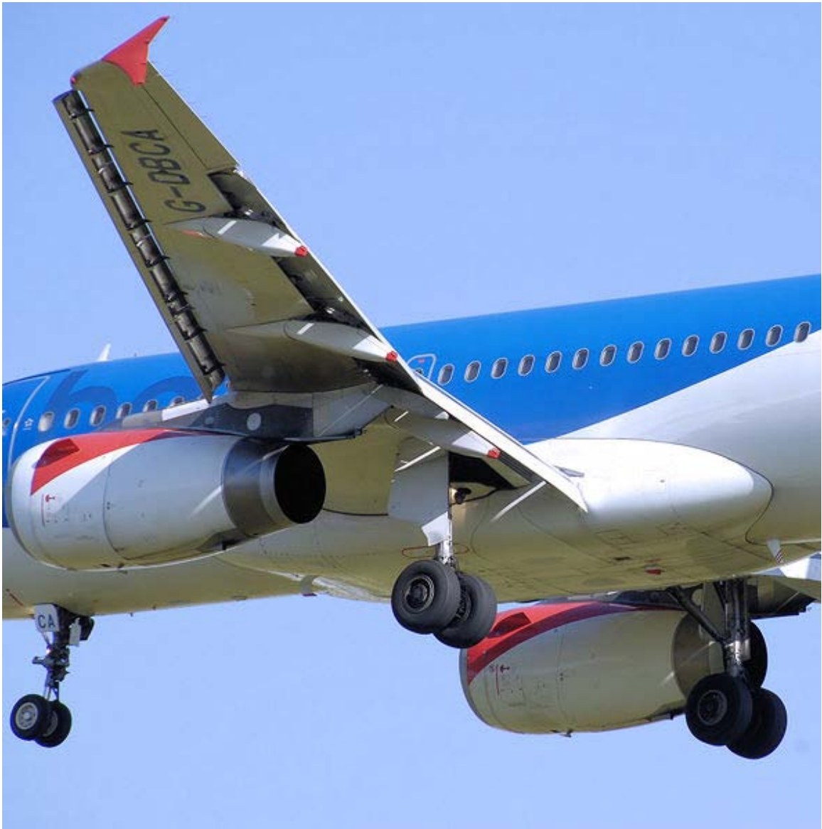
The wing of a landing bmi Airbus A319-100. The slats at the leading edge and the flaps at the trailing edge are extended.
