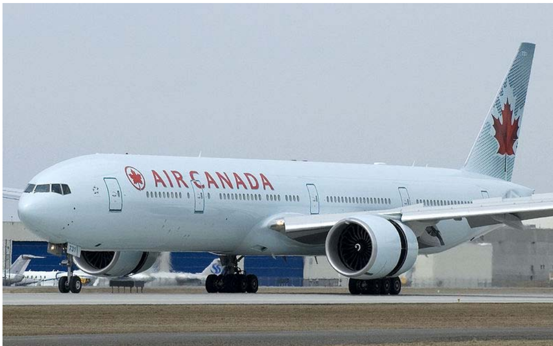
An Air Canada Boeing 777 with thrust reversers deployed, visible as a gap in the engine nacelle
