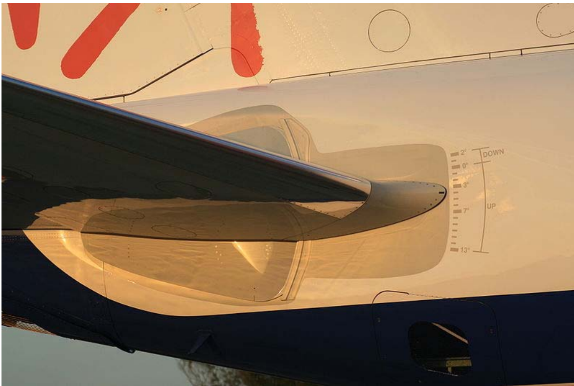
Adjustable stabilizer on an Embraer ERJ-170, with markings showing the degree of nose-up and nose-down trim available
