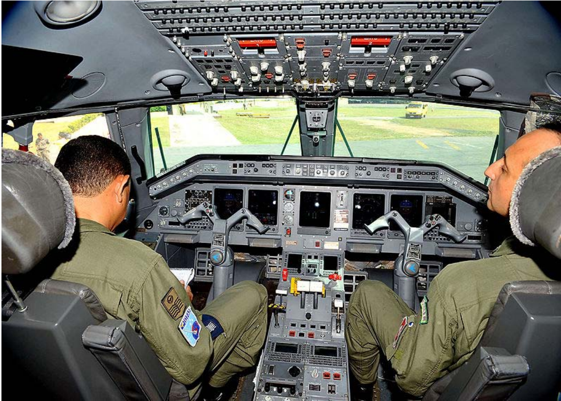
The cockpit of an Embraer ERJ with an "M" shaped yoke
