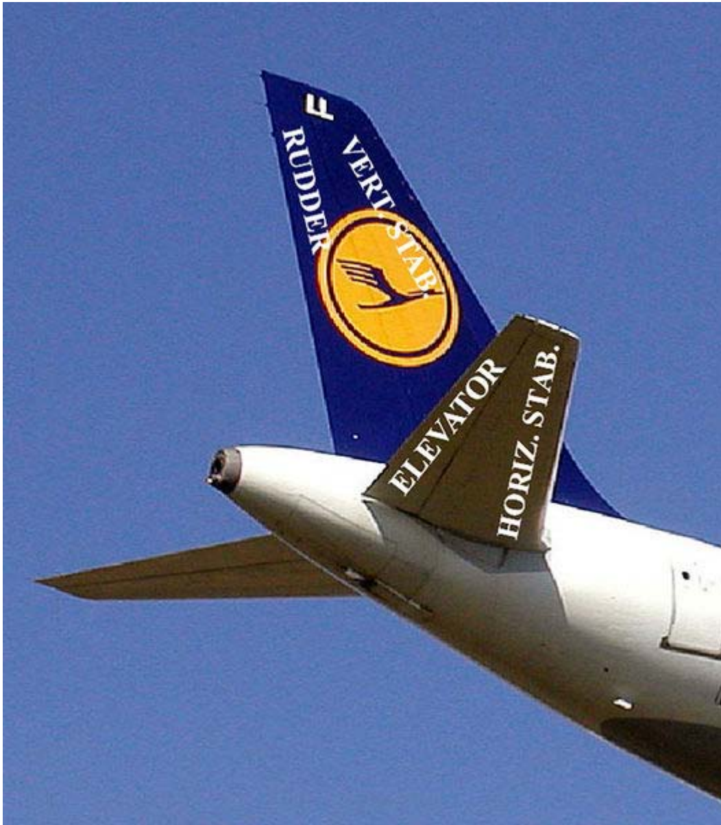
The tail of a Lufthansa airliner (Airbus A319) in flight, showing the horizontal and vertical stabilizer
