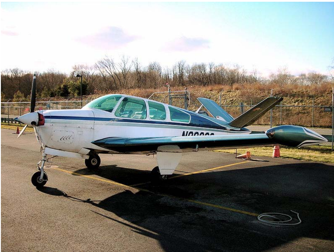
The Beechcraft Bonanza, the most common example of V-Tail empennage configuration
