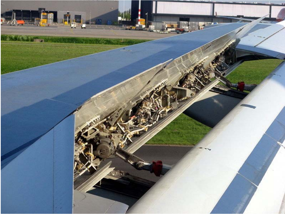
A close look at the inner workings of the spoiler during the landing of an Airbus A320
