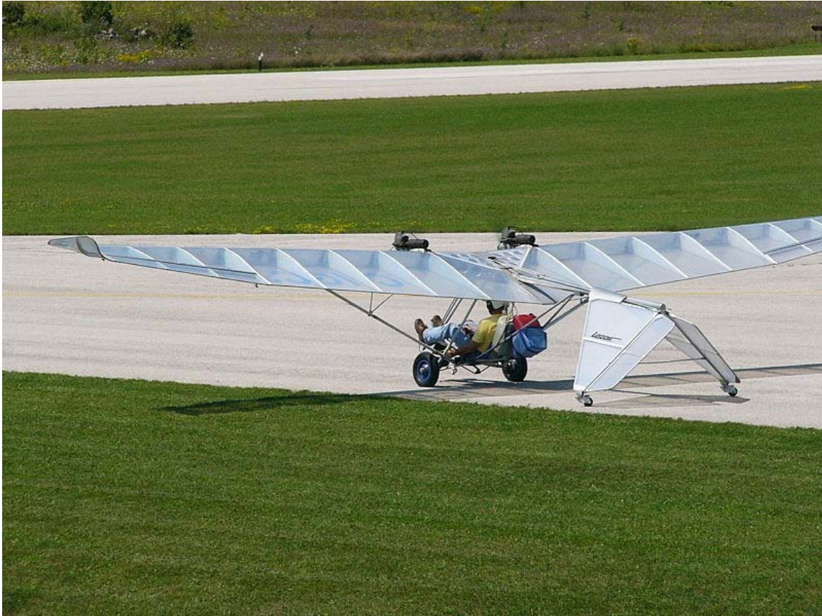
An Ultraflight Lazair showing its inverted V-tail covered with translucent Tedlar
