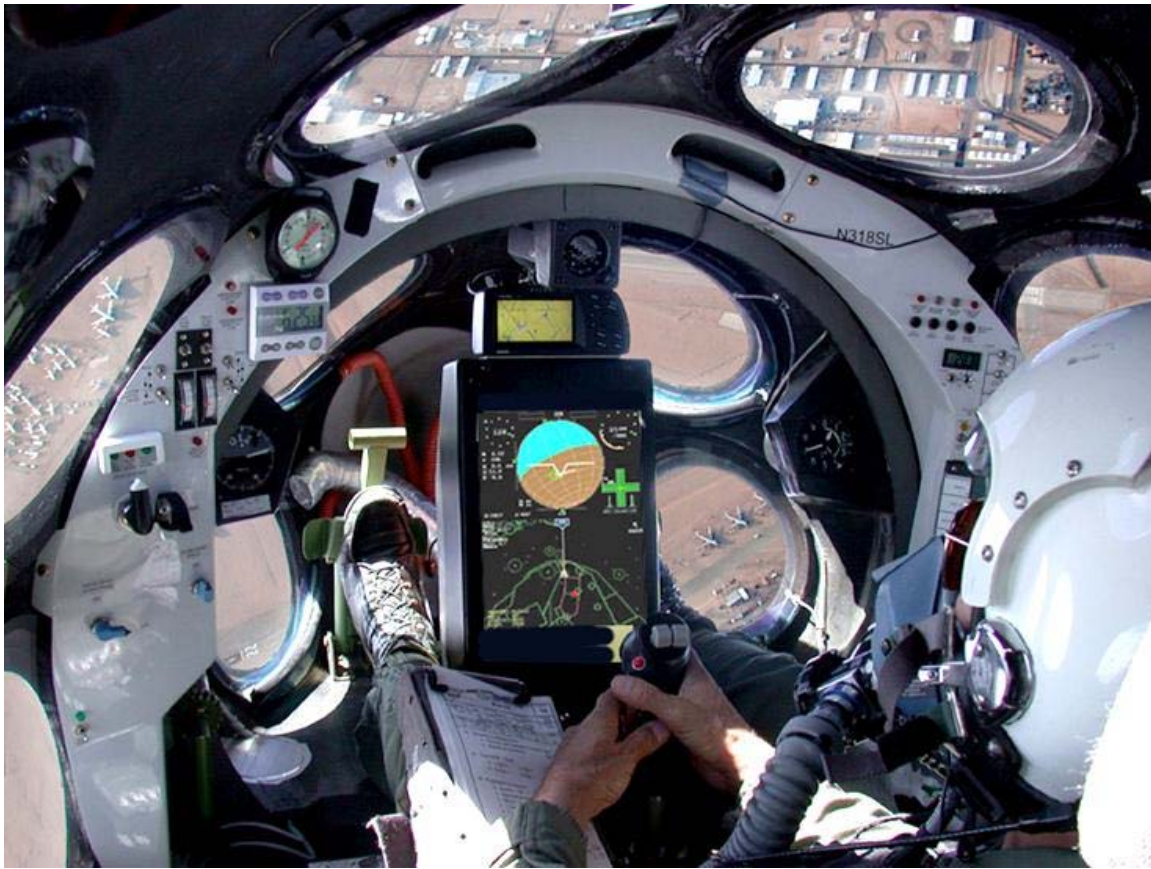
Cockpit of WhiteKnight in flight, EFIS display edited to look like SpaceShipOne
