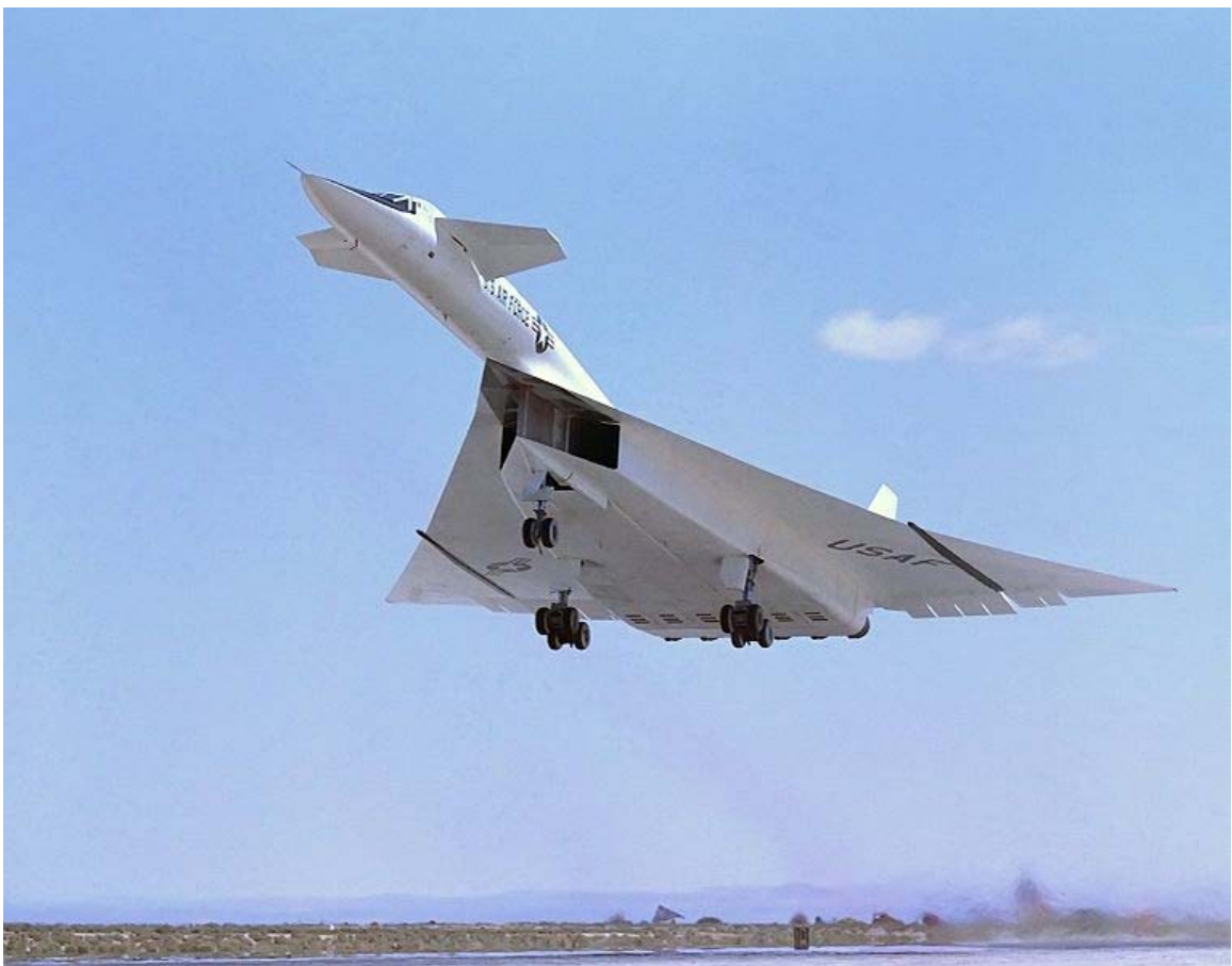
Canards (just behind the flight deck) on the XB-70 Valkyrie experimental bomber aircraft
