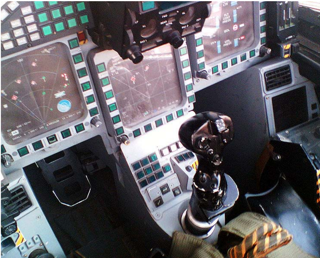
MHDDs and Pedestal Panel with centre stick in the Typhoon cockpit
