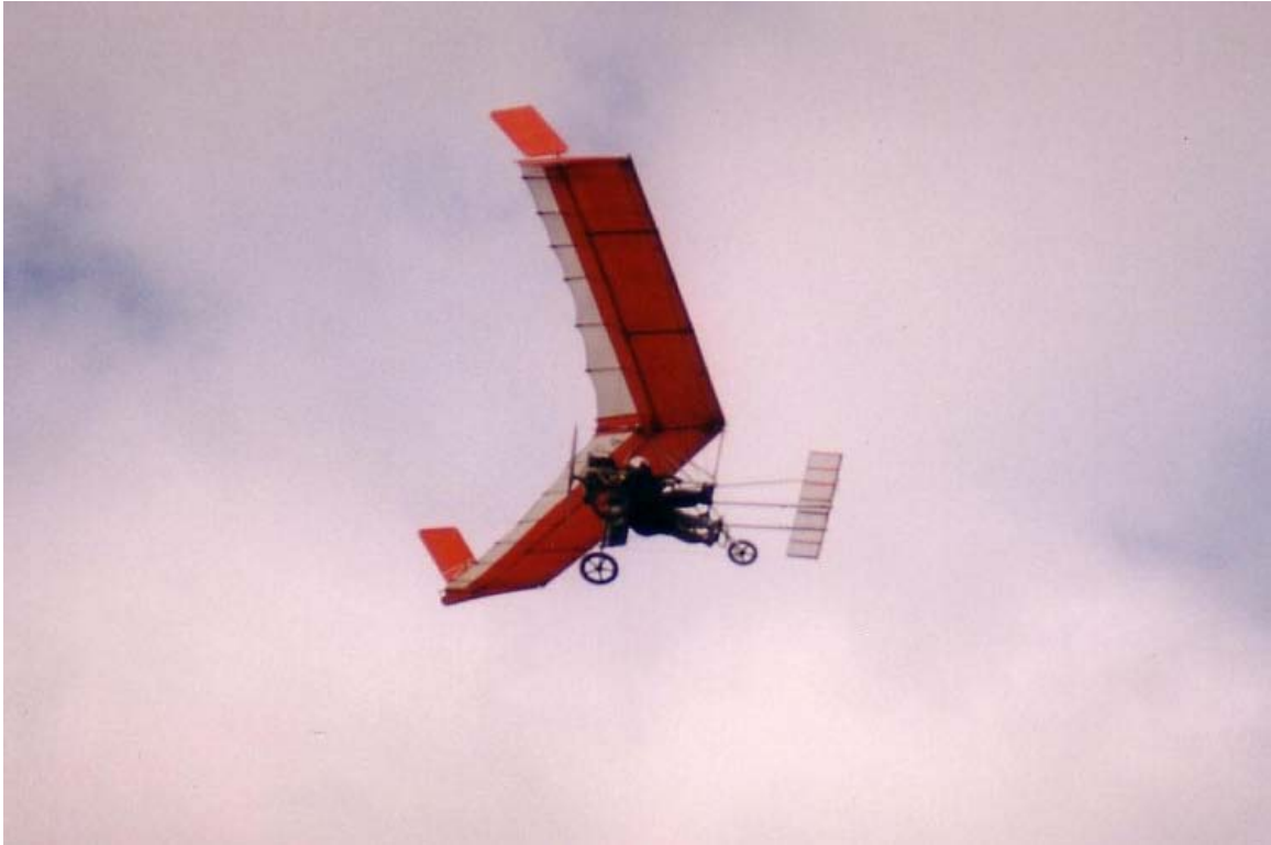
A Pterodactyl Ascender II+2 showing its canard control surface
