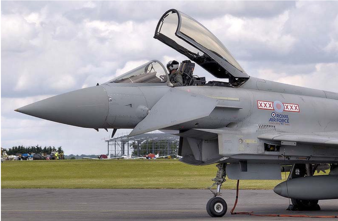
Close up view of an RAF Typhoon F2, showing the deflected canard control surface immediately below the pilot
