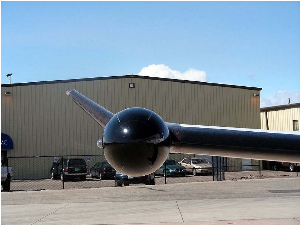
Weather radar on the wing of Pilatus PC-12
