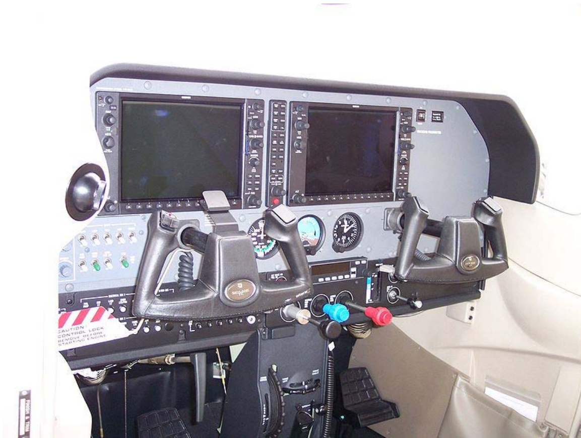
Garmin G1000 displays in a Cessna 182
