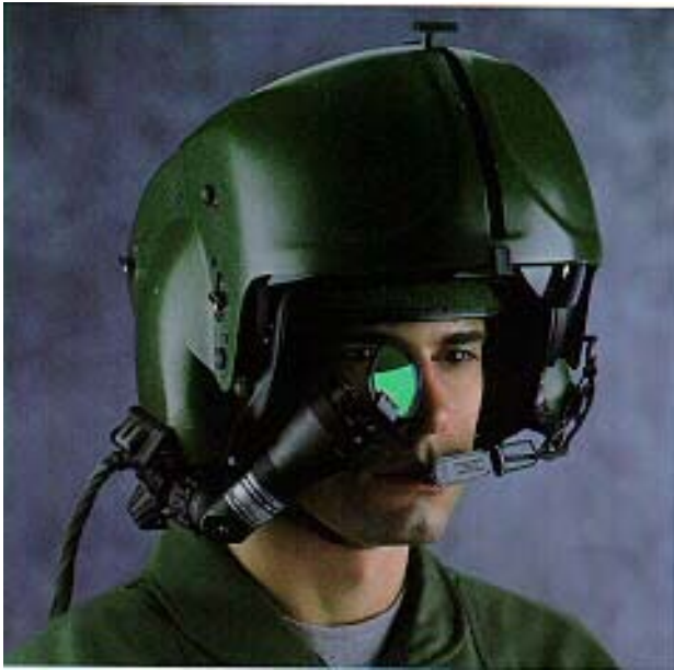
The Integrated Helmet and Display Sight System (IHADSS)
