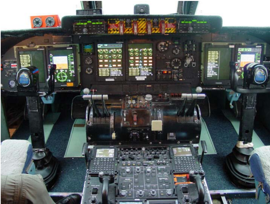
New instrument panel for C-5 as part of AMP program
