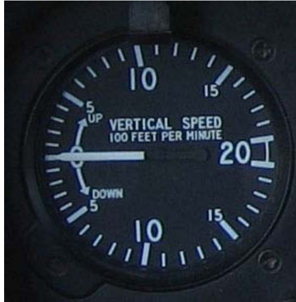
The vertical speed indicator from a Robinson R22
