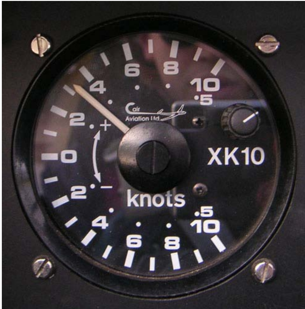
Panel mounted variometer for gliders
