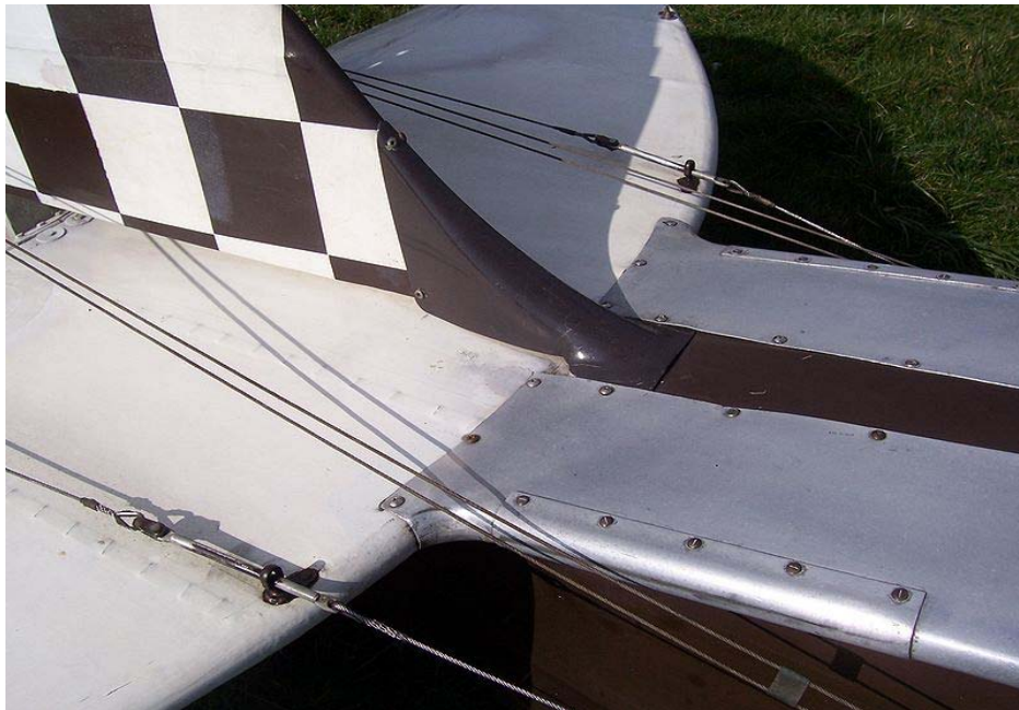
de Havilland Tiger Moth elevator and rudder cables
