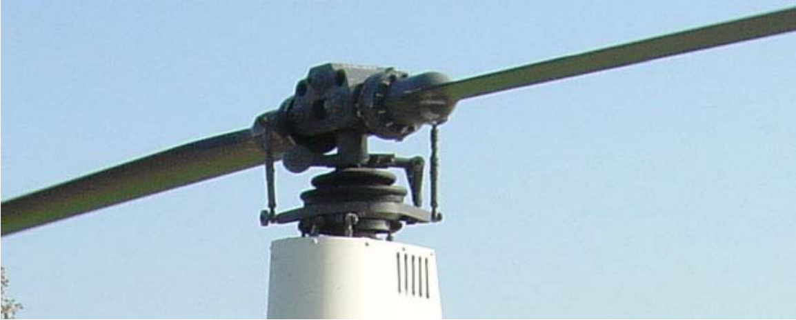
The simple rotor of a Robinson R22
