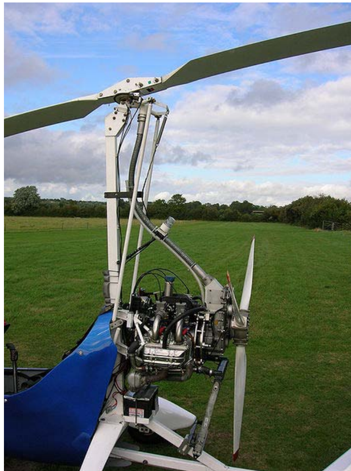
The rotor head, pre-rotator shaft and Subaru engine configuration on a VPM M-16 autogyro
