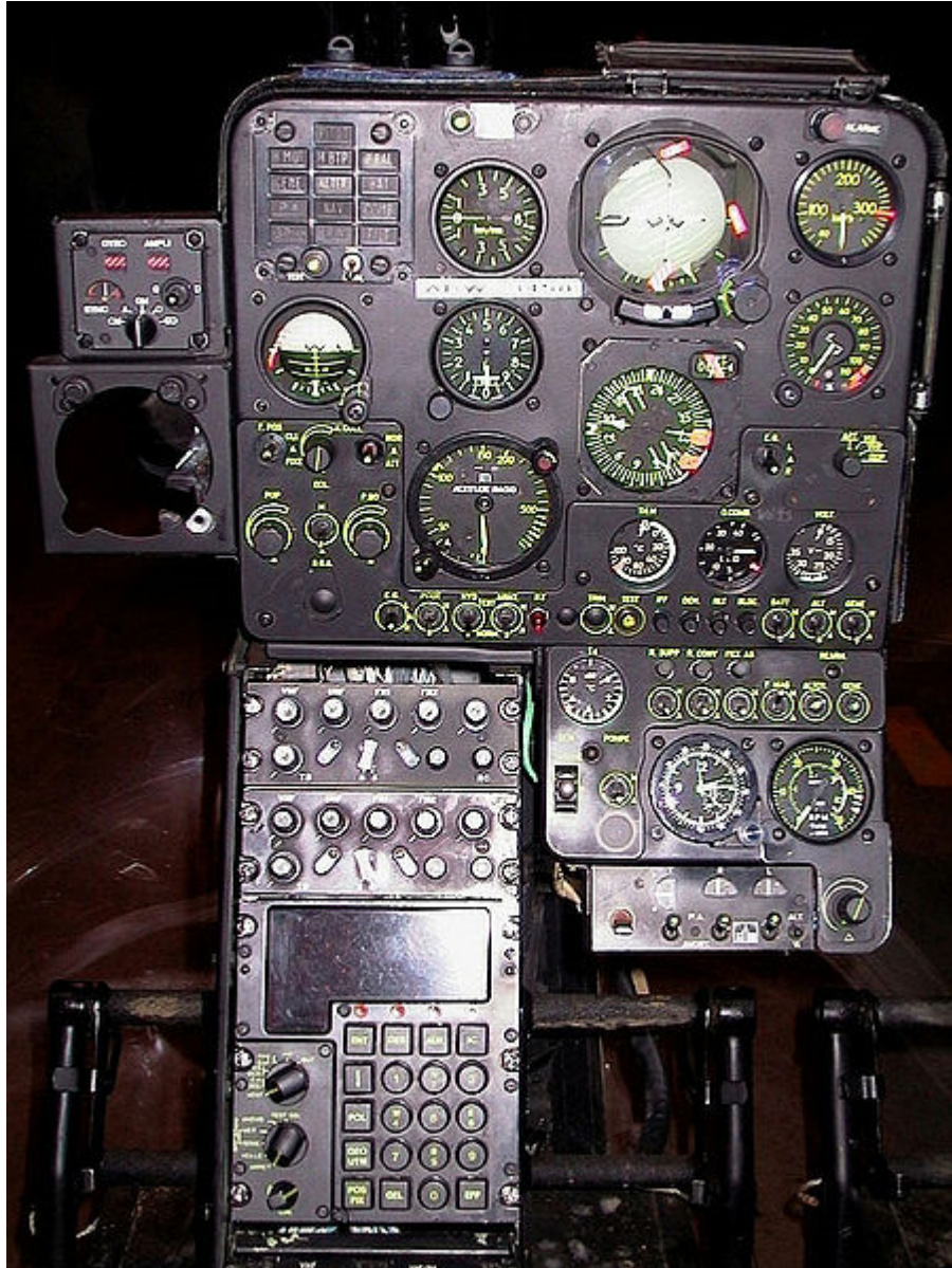
Control panel of a Gazelle SA 342M of the French Army's Light Aviation (ALAT)
