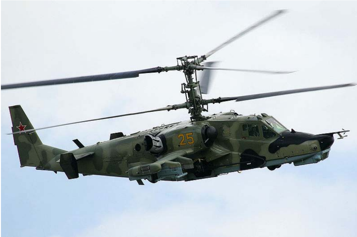
Kamov Ka-50 of the Russian Air Force, with coaxial rotors
