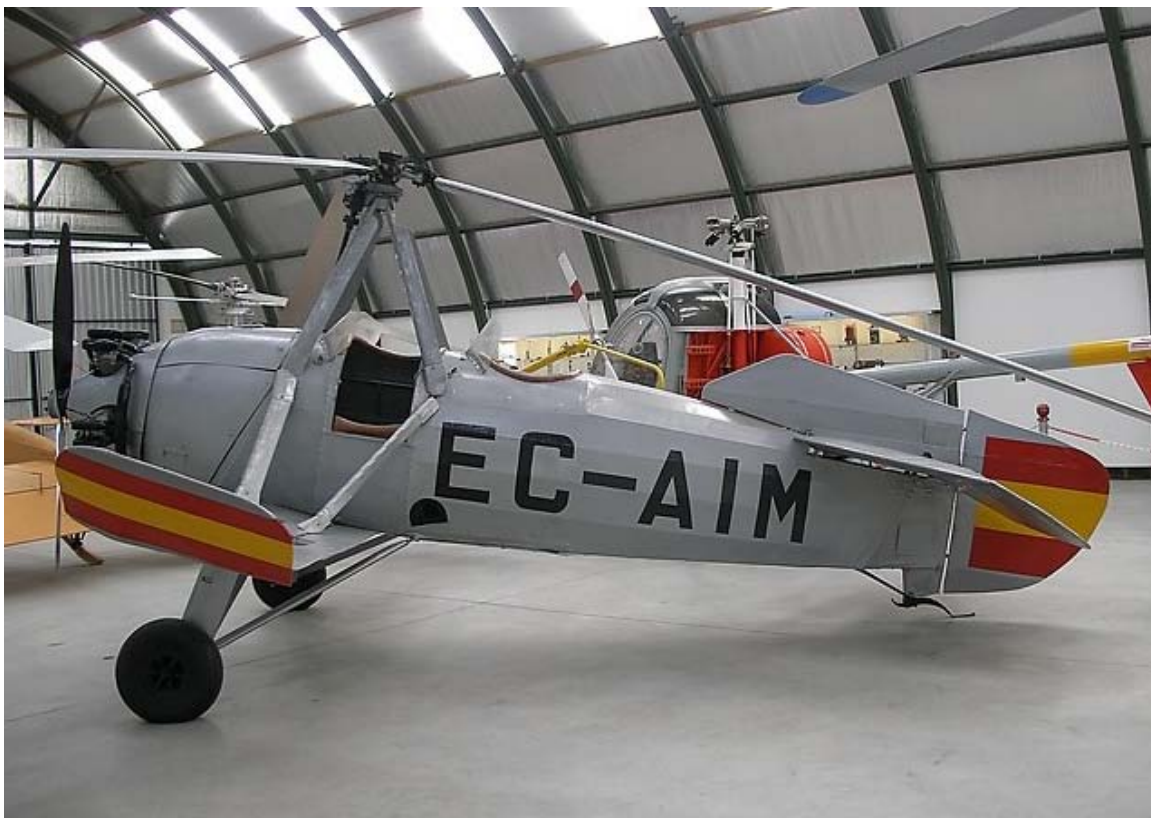
Avro-built Cierva C.19 Mk.IV Autogyro, built in 1932. Cuatro Vientos Airport Museum, Madrid, Spain.
