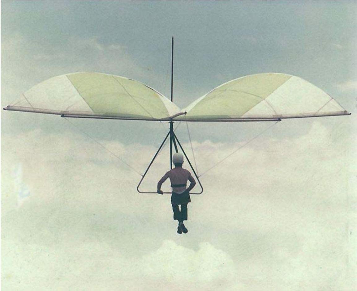
'Standard' flexible wing hang glider, based on variants of the Rogallo wing aircraft, 1975
