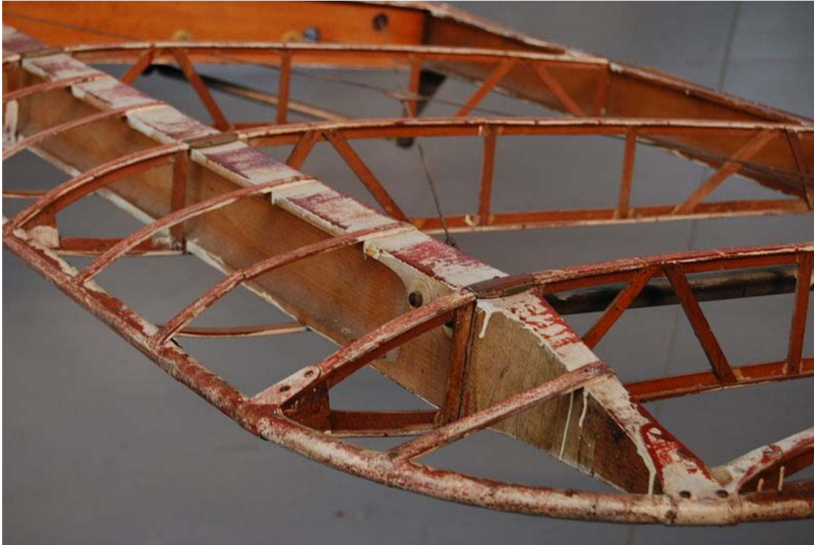
Wing ribs of a de Havilland DH.60 Moth
