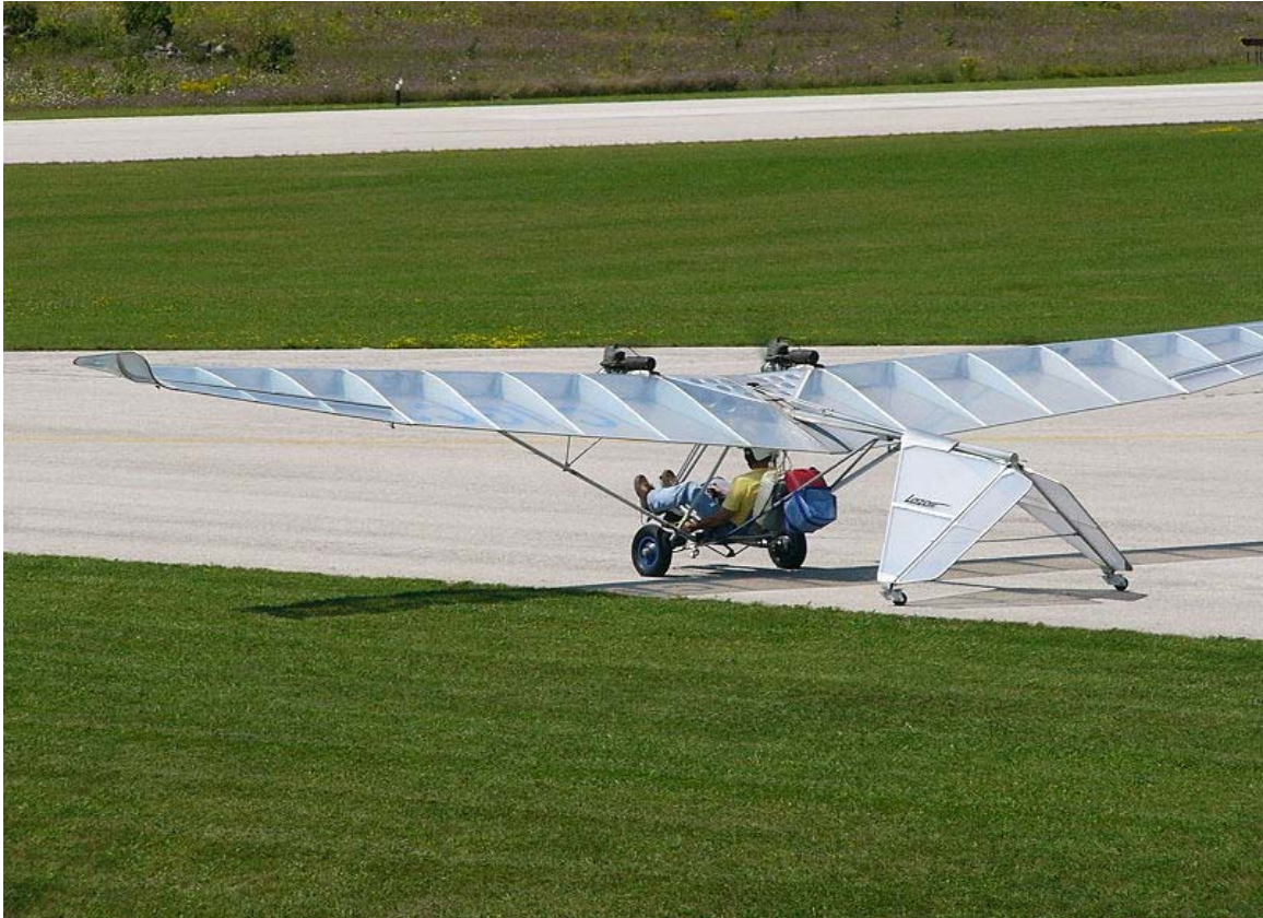
Canadian Lazair ultralight covered in clear Mylar
