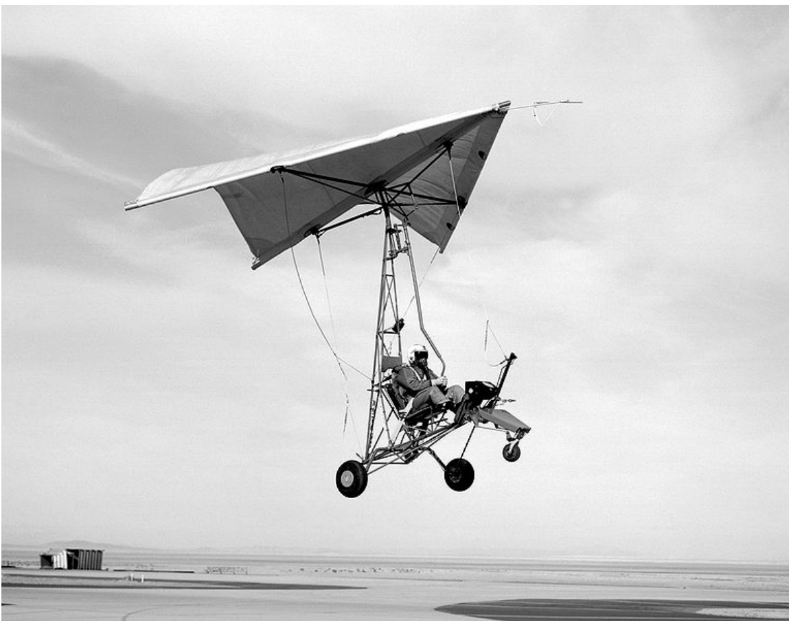
First towing tests of NASA's Paresev glider (Para Wing Research Vehicle), March 1962
