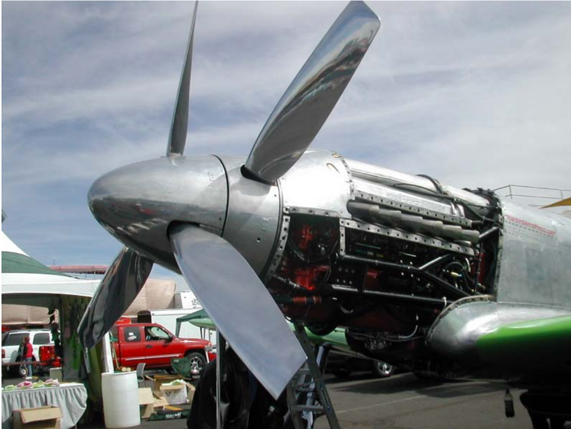
Contra-rotating propellers of a modified P-51 Mustang fitted with a Rolls-Royce Griffon.
