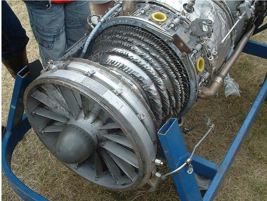
Inside of a jet engine after a bird strike
