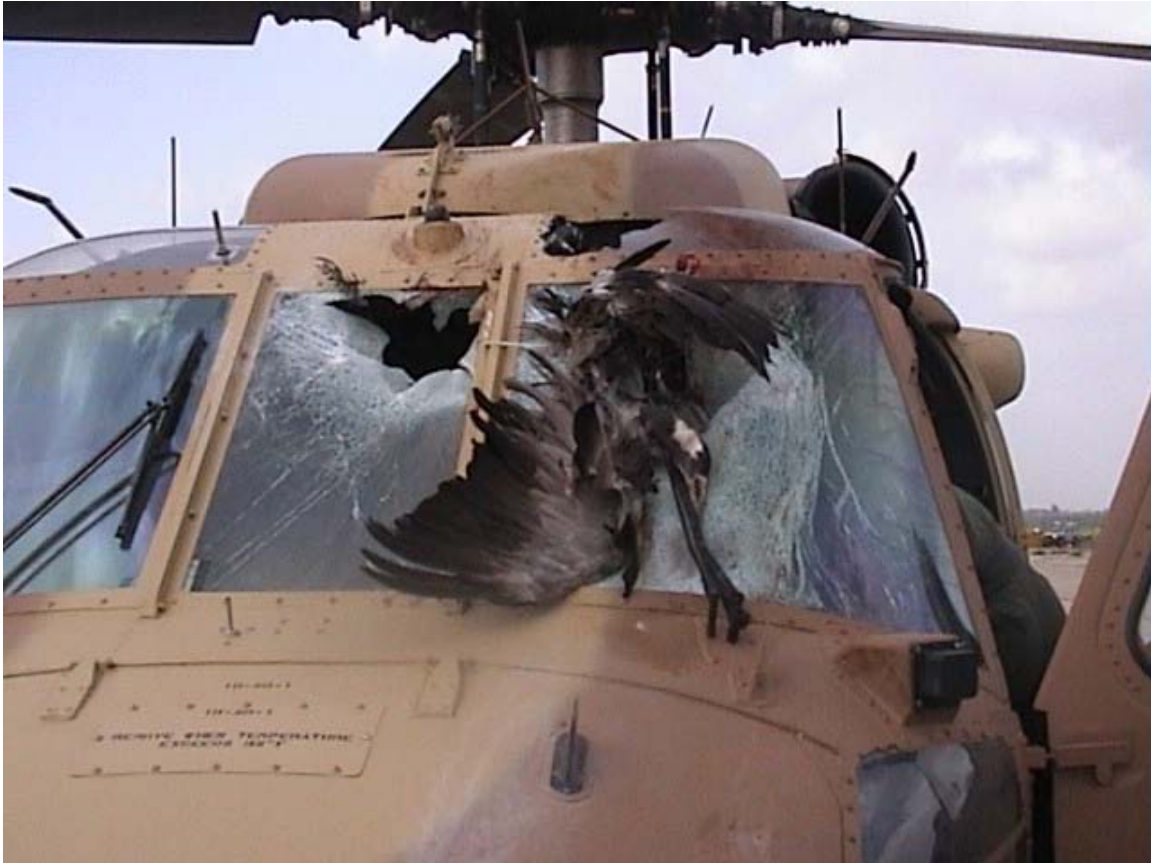
A UH-60 Black Hawk after a collision with a Common Crane, and resulting failure of the windshield.
