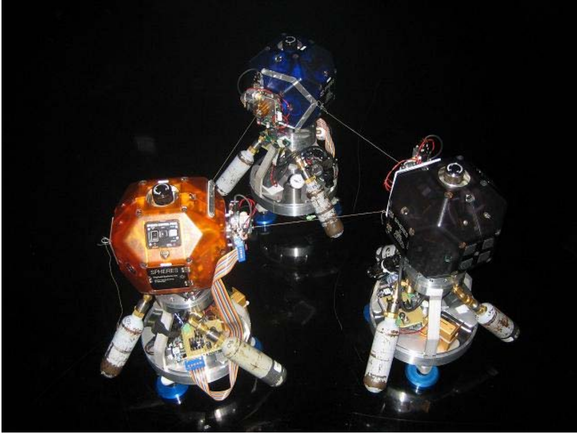
Tethered SPHERES nano-satellites developed by MIT
