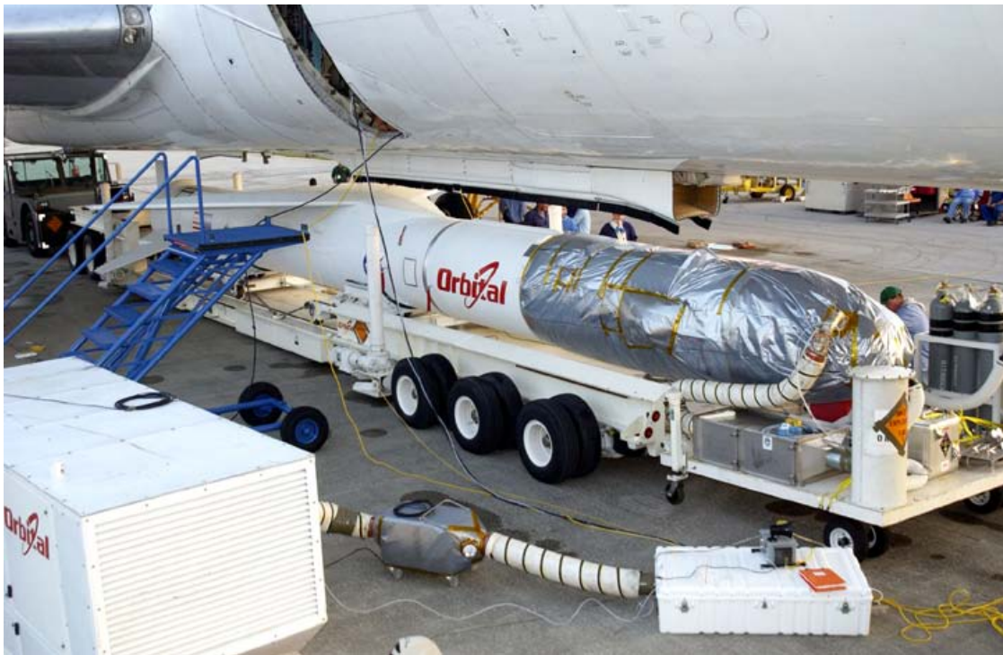
GALEX's Pegasus XL being attached to the L-1011 Stargazer
