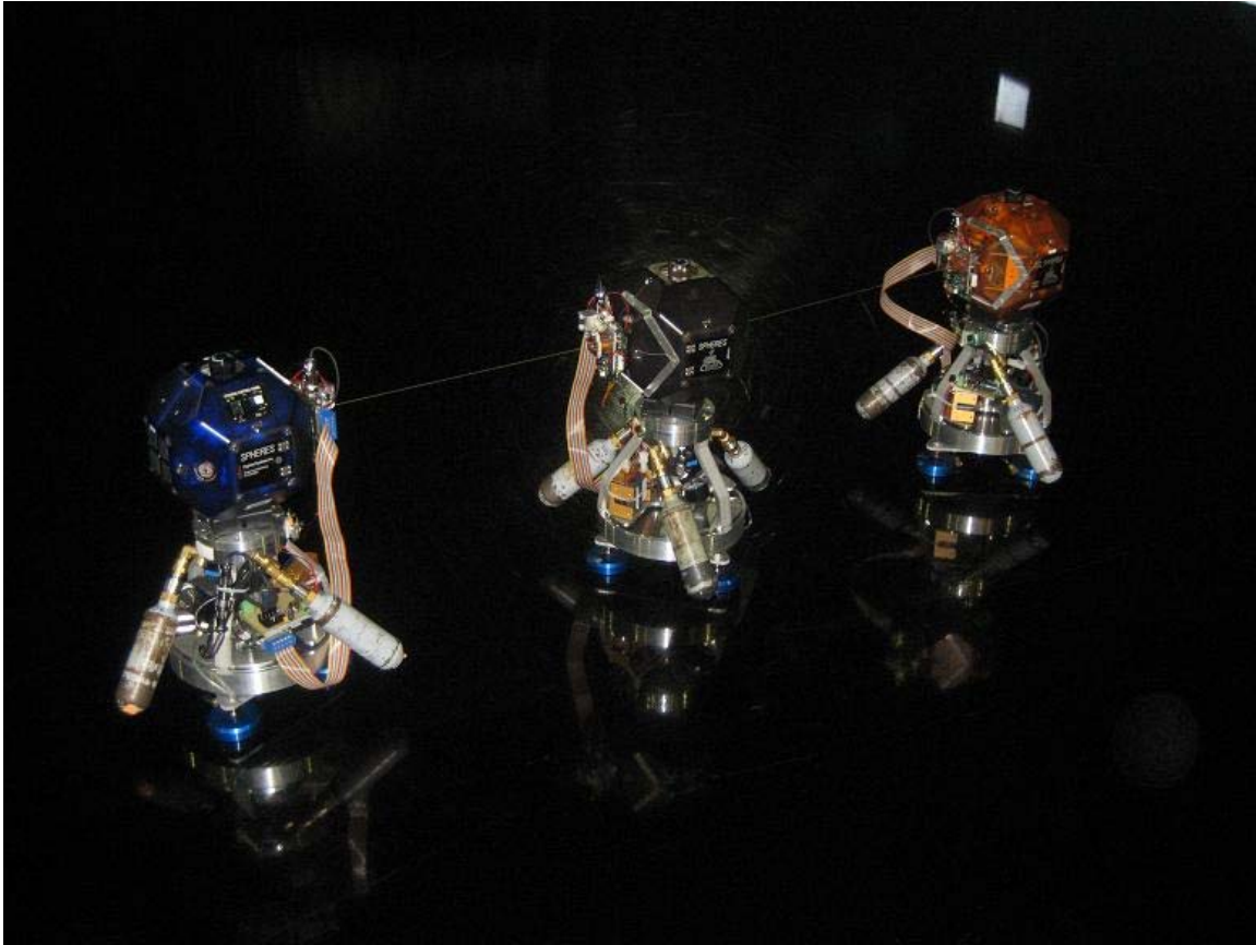
Tethered SPHERES nano-satellites developed by MIT
