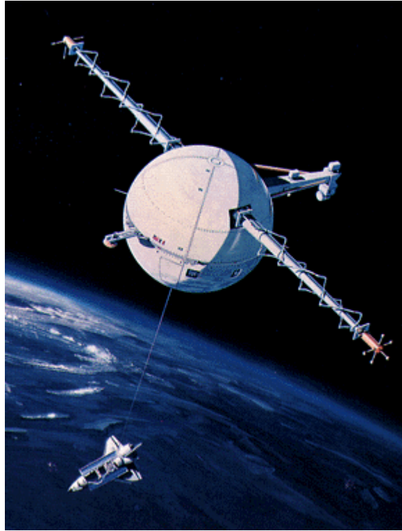
A NASA artist's rendering of a satellite tethered to the space shuttle.
