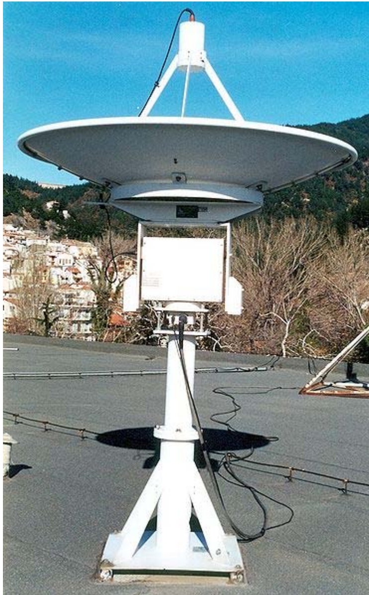
Computer controlled motorized parabolic dish antenna for tracking LEO weather satellites
