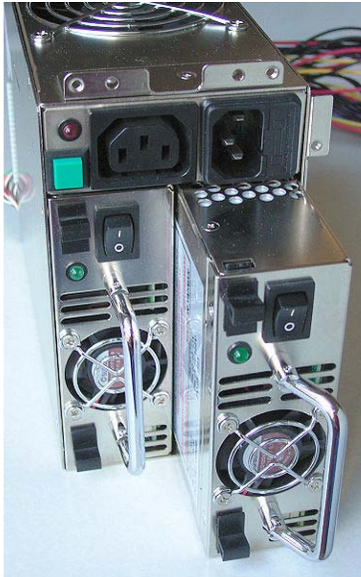
Redundant power supply
