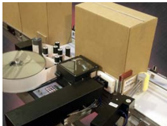
Label printer applicator applying a label to adjacent panels of a corrugated box.
