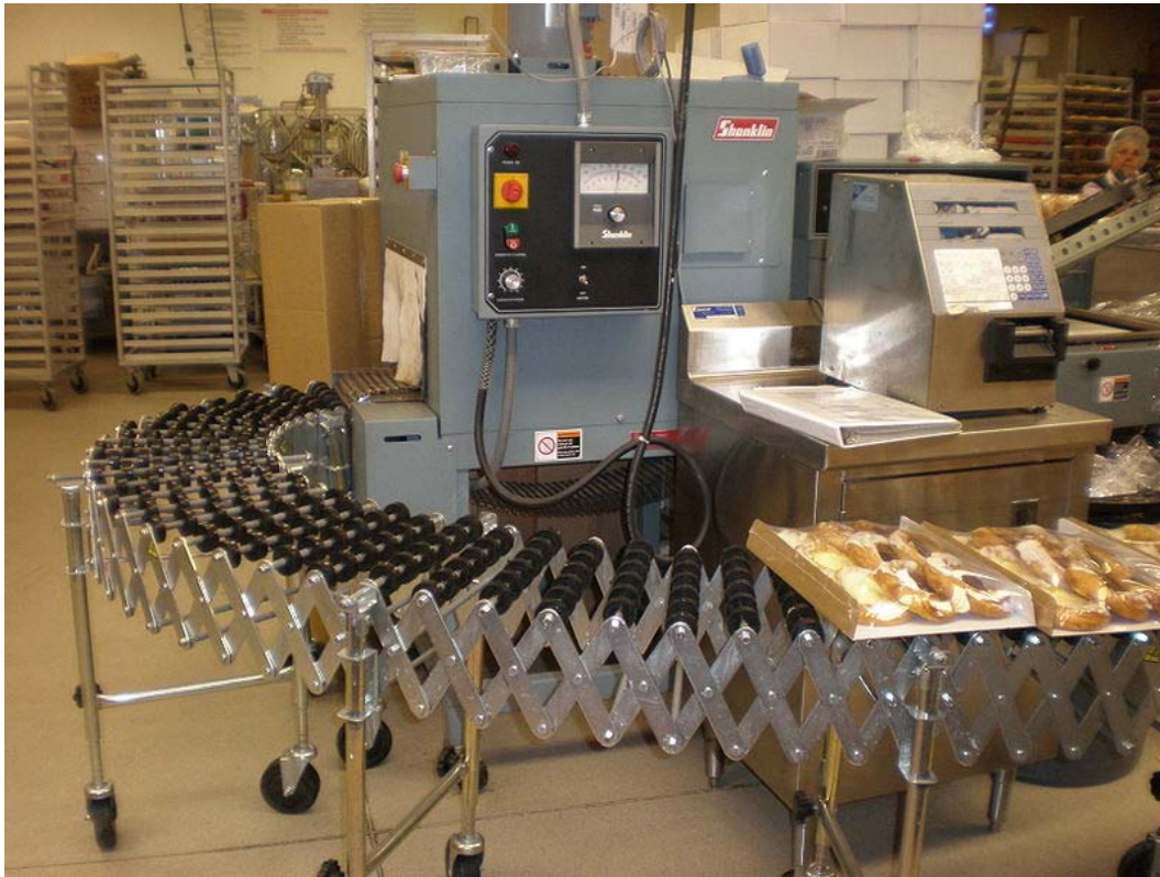
Bakery goods shrinkwrapped by shrink film, heat sealer and heat tunnel on roller conveyer
