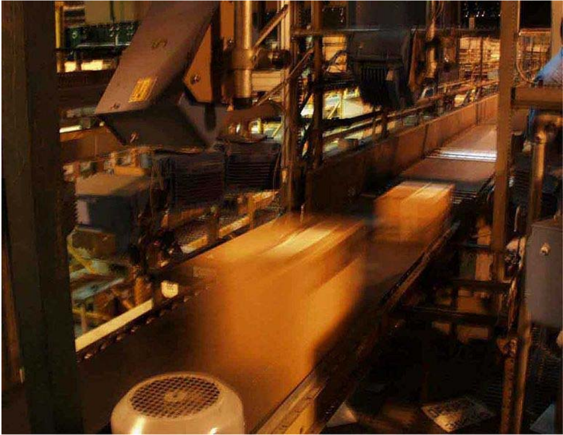
High speed conveyor with bar code scanner for sorting transport packages
