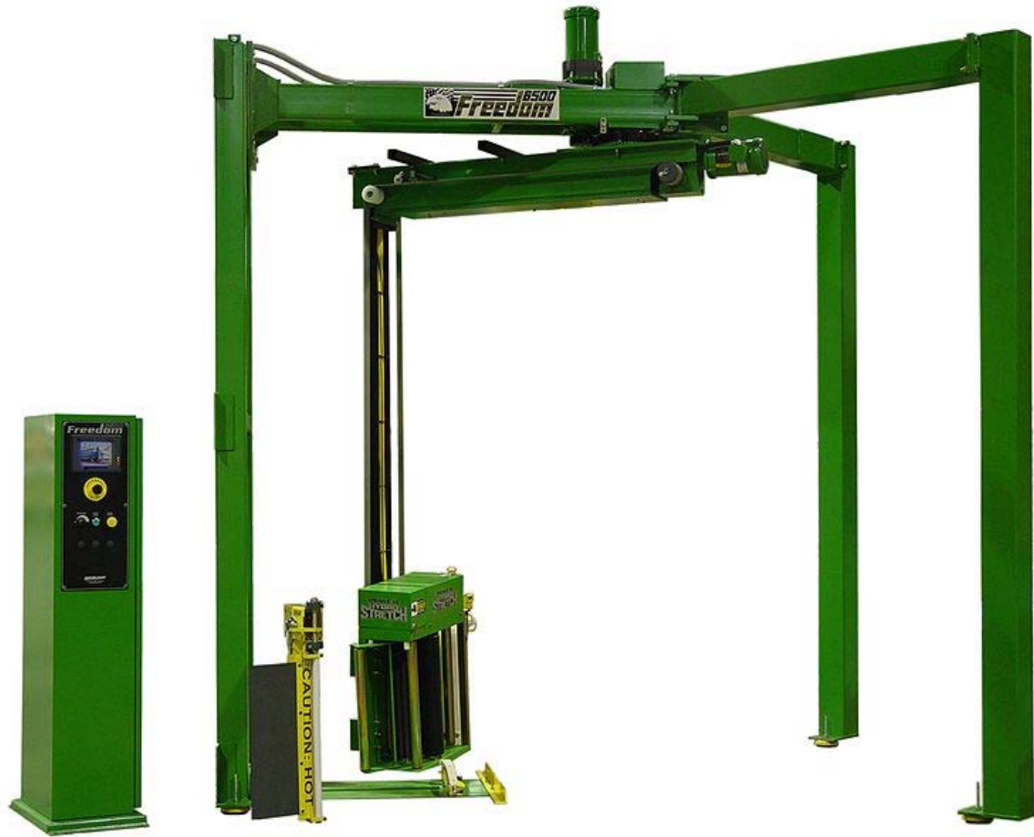
A semi-automatic Rotary Arm Stretch Wrapper
