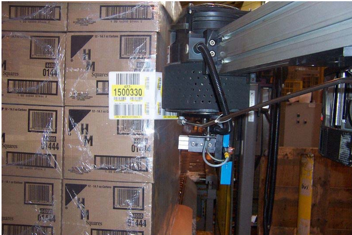
"Print & Apply" corner wrap UCC (GS1-128) label application to a pallet load
