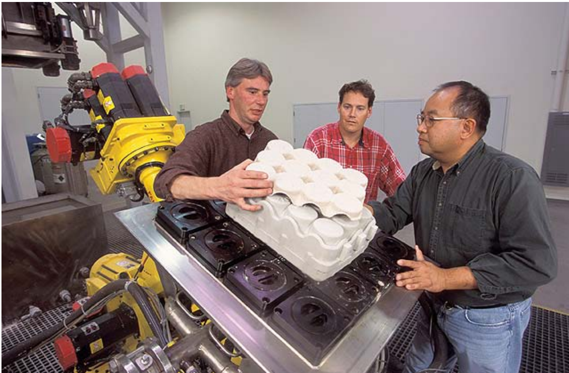
Equipment used for making molded pulp components and molding packaging from straw
