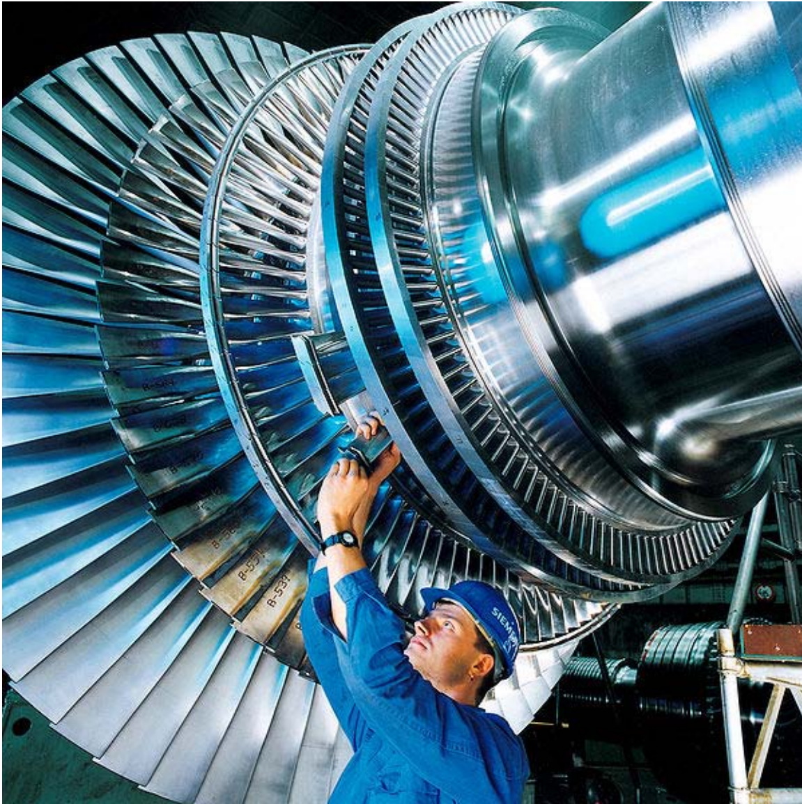
Rotor of a modern steam turbine, used in power station.
