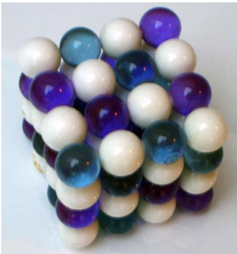
Fig. 2. Sodium chloride (NaCl) lattice, showing close-packed spheres representing a face-centered cubic AB lattice similar to that of NaCl and most other alkali halides. In this
