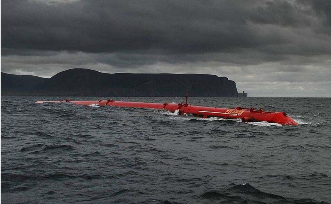
A Pelamis wave device under test at the European Marine Energy Centre (EMEC), Orkney, Scotland.
