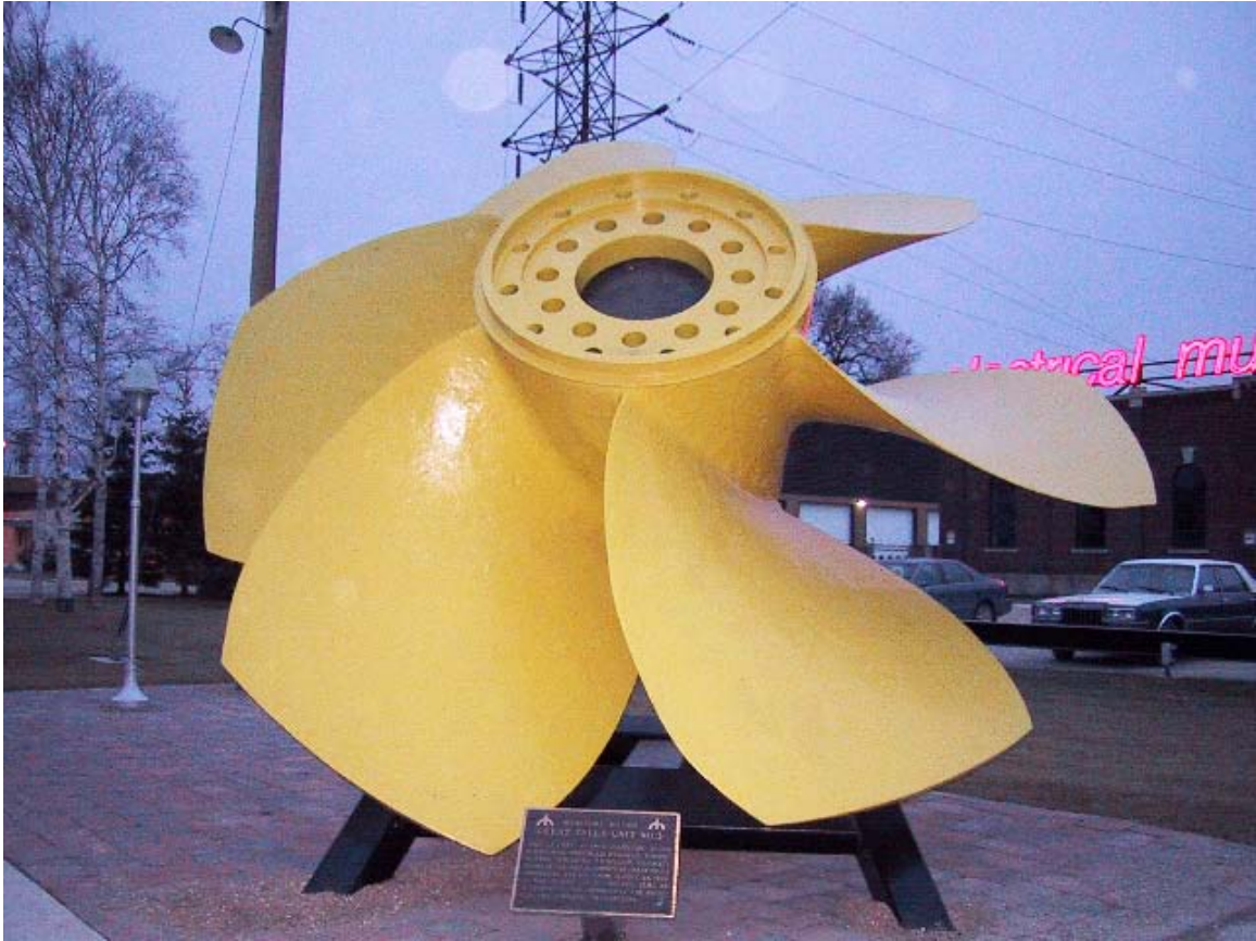
A propeller-type runner rated 28,000 hp (21 MW)
