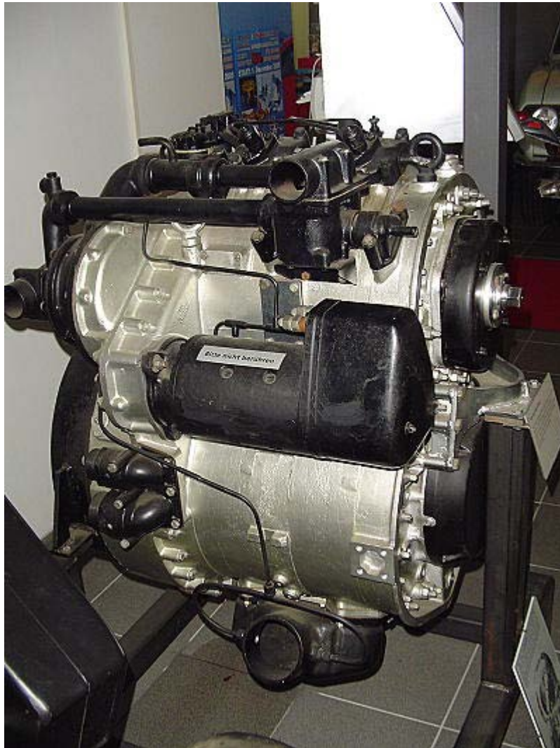
Rolls Royce R6 two stage Wankel Diesel engine
