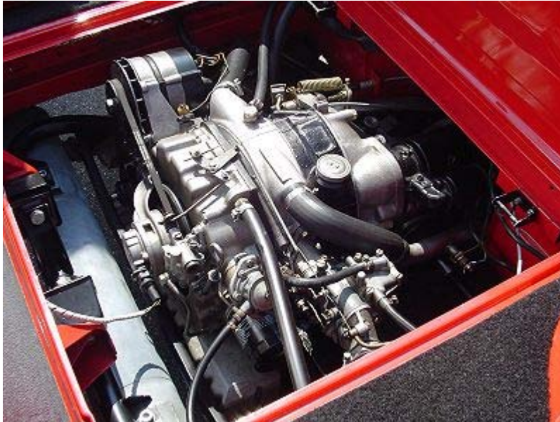
NSU Wankel Spider, the first line of cars sold with a rotor Wankel engine
