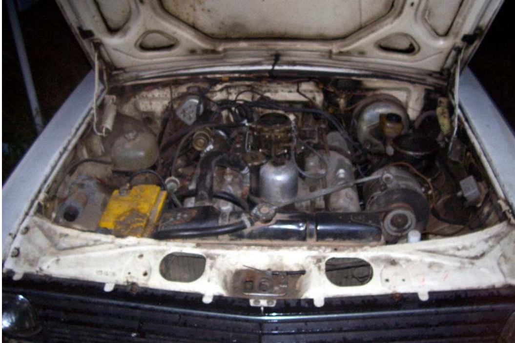
GAZ-24-34 Volga with ZMZ-503 V8 engine, 1992-built car.
