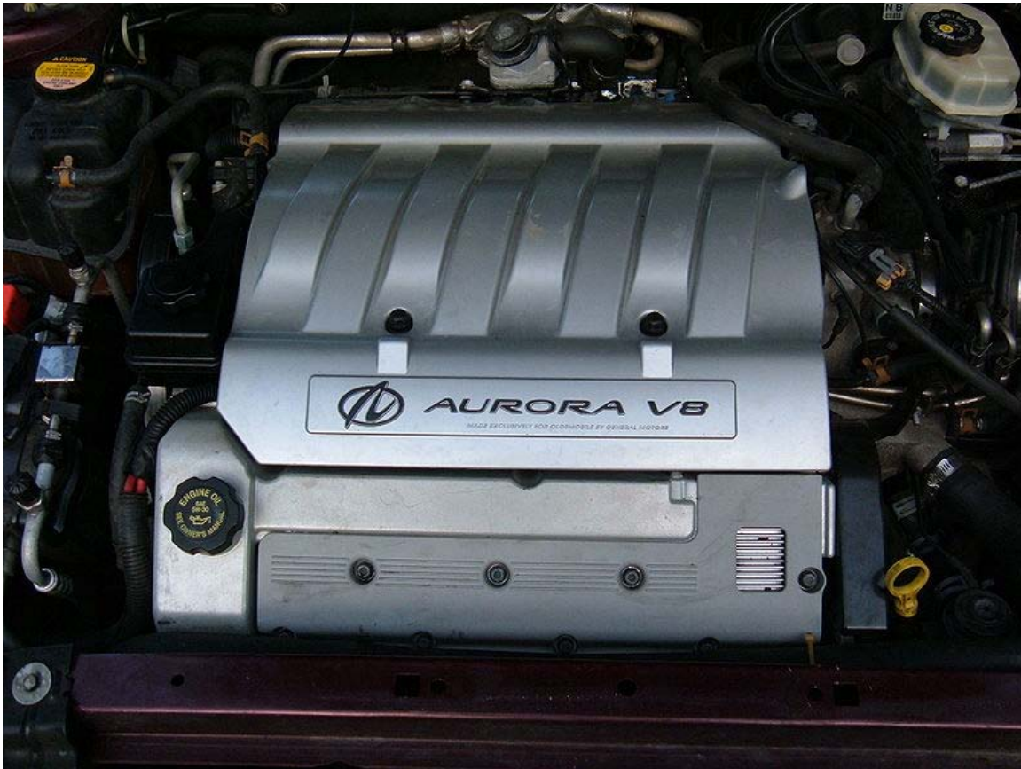
A 4.0 L (244 cu in) V8 engine from an Oldsmobile Aurora
