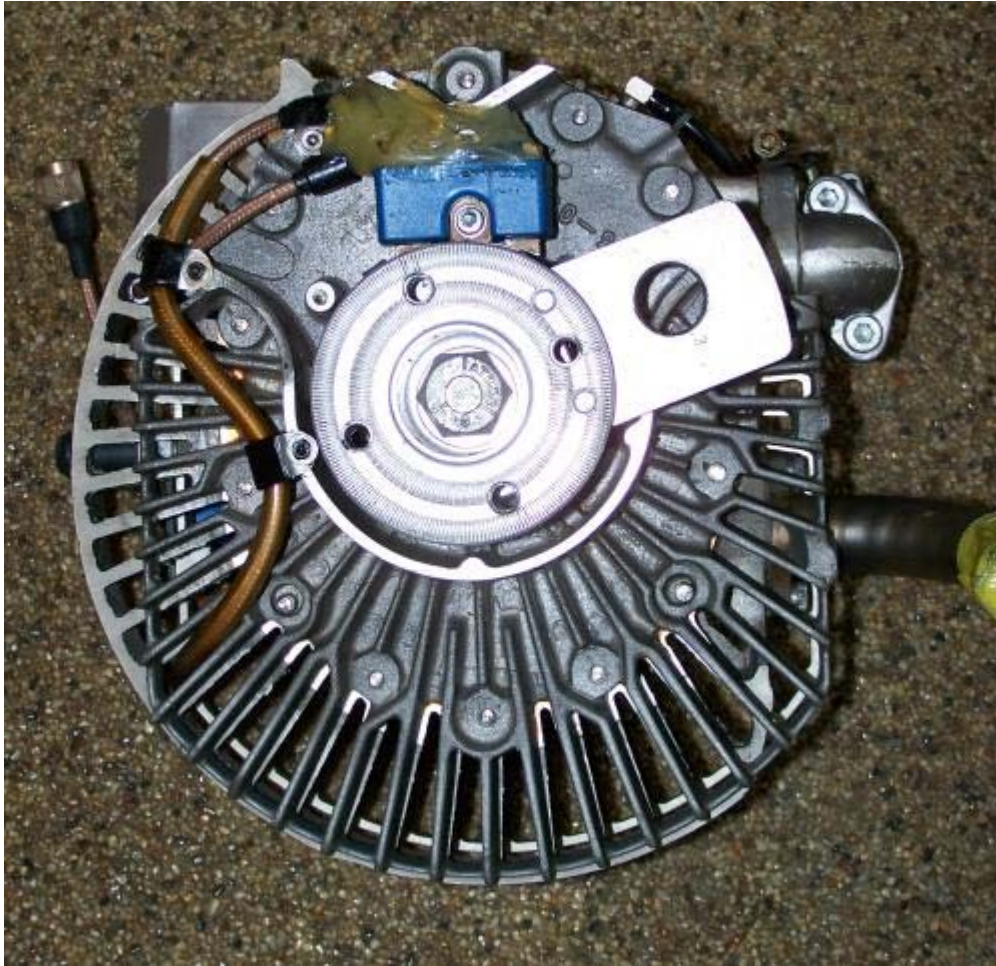
UEL UAV-741 Wankel engine for a UAV
