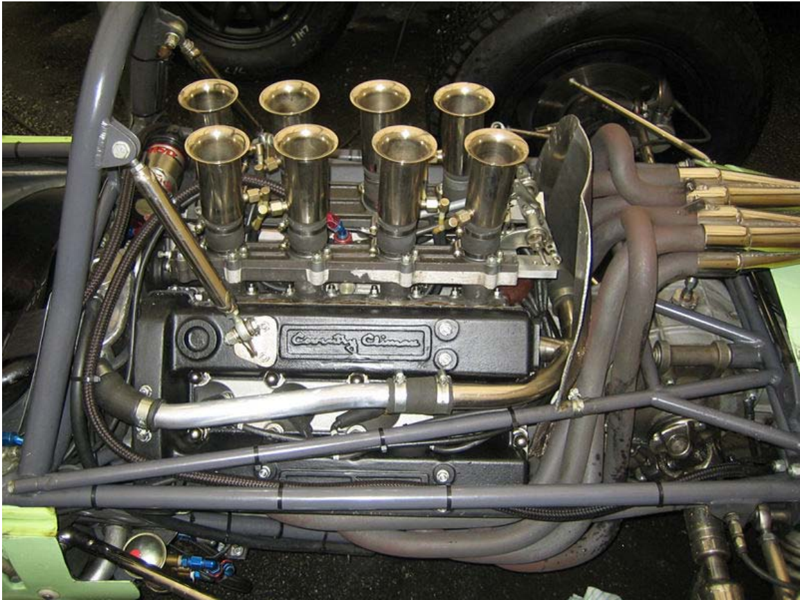
1962 Coventry Climax FWMV 1500cc V8 Formula 1 engine in a Lotus 24
