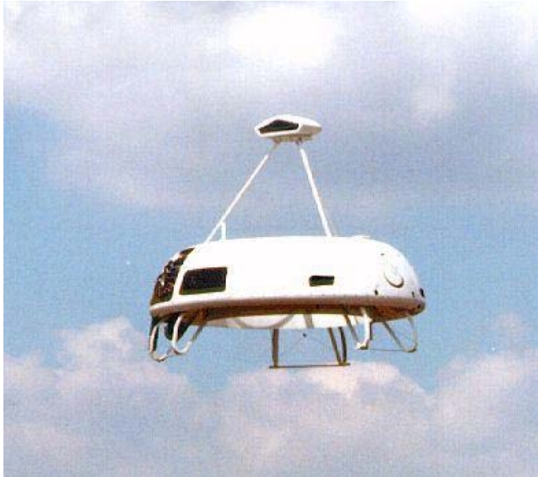
Sikorsky Cypher UAV powered with a UEL AR801 Wankel engine
