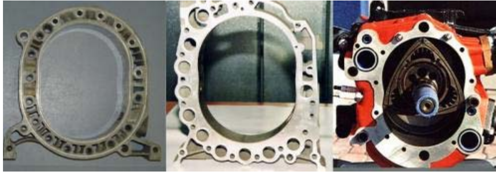
Left Mazda old L10A Camber axial cooling, middle Audi NSU EA871 axial water cooling only hot bow, right Diamond Engines Wankel radial cooling only in the hot bow
