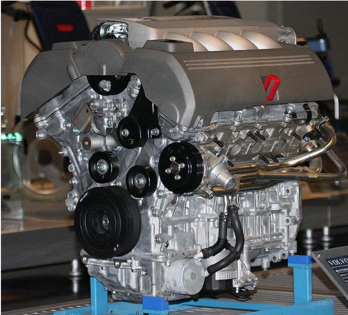
2005 Volvo (Yamaha) V8 engine for Volvo XC90. V8 4,414cc
