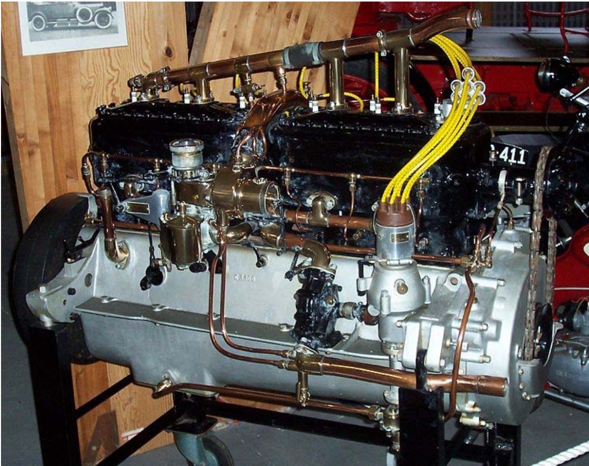
Rolls-Royce 40/50hp Silver Ghost 7,400cc side valve six cylinder engine
