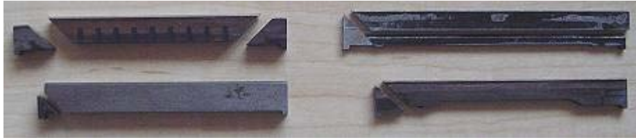
Apex seals, left NSU Ro80 Serie and Research and right Mazda 12A and 13B
