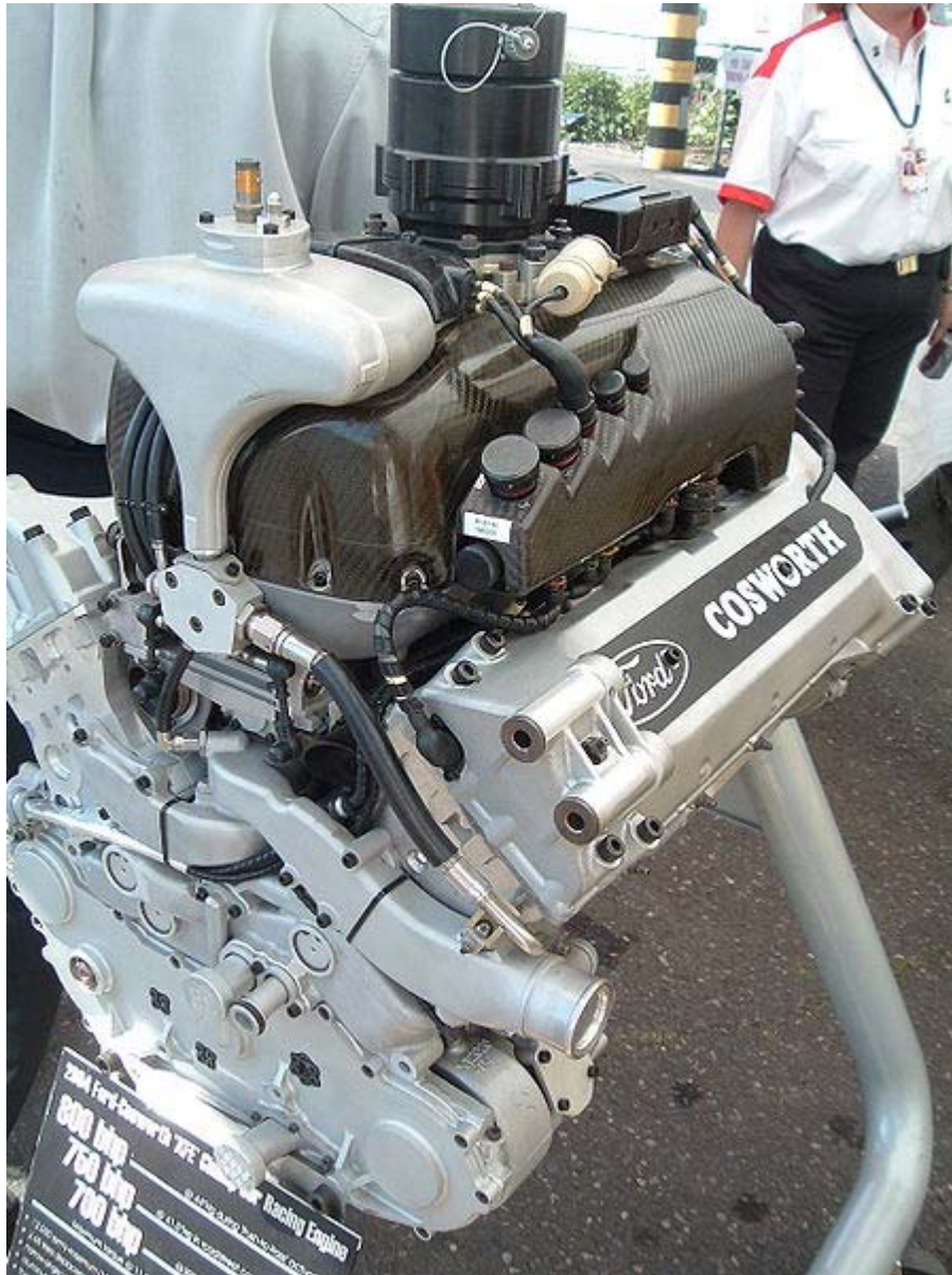
A 2004 Cosworth Champ Car World Series V-8 engine, capable of generating over 800 horsepower from just 161 cu./in
