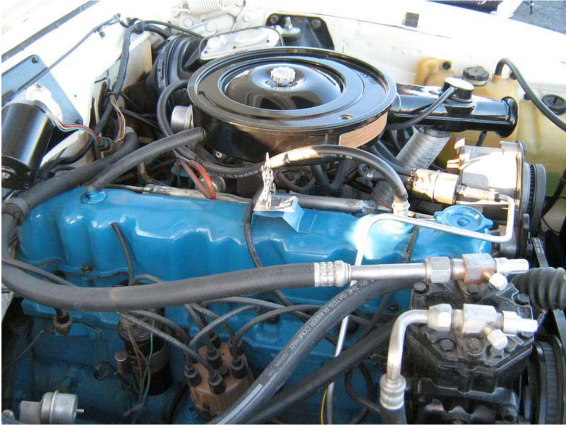
Carbureted 1977 AMC 258 cu in (4.2 L)
