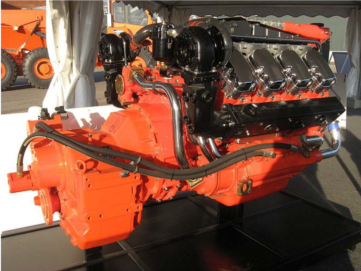
Scania V8, 16 litre marine engine with reverse.
