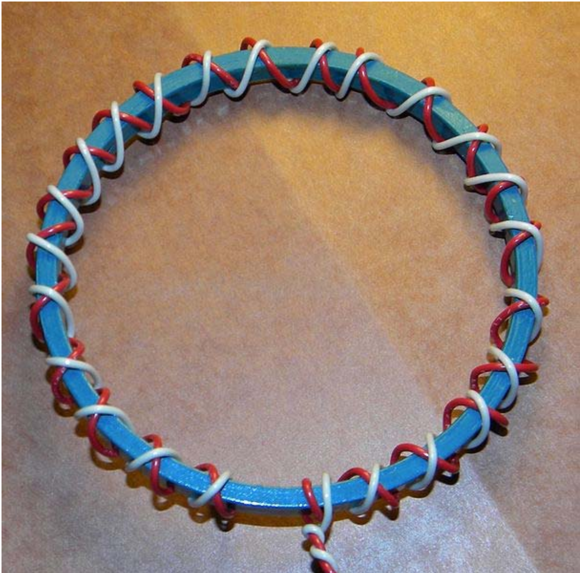
Fig. 5. Circumferential current countered with a return winding.
