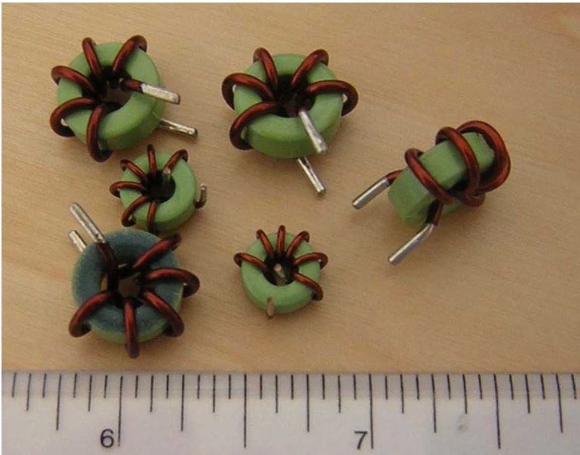
Several small toroidal inductors. The major scale is in inches.
