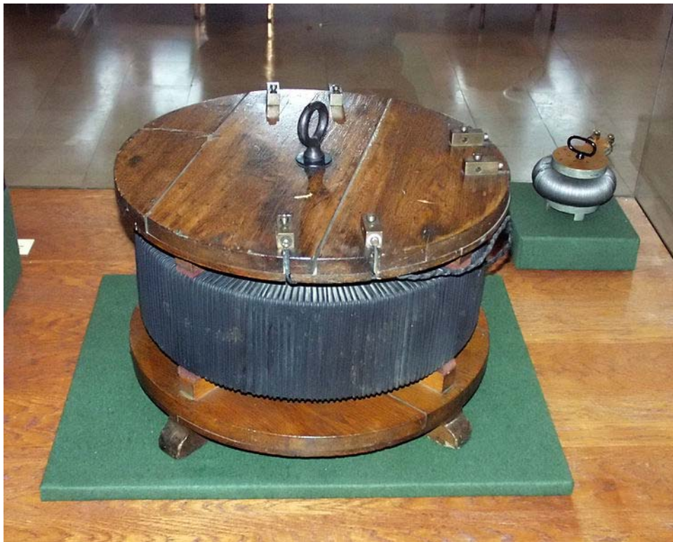
Prototypes of the world's first high-efficiency transformers. They were built by the Z.B.D. team on 16th September 1884.
