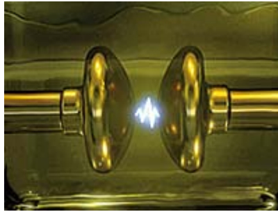
Voltage breakdown during transformer oil testing
