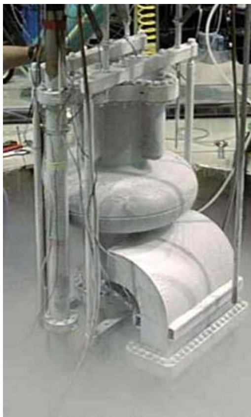
Photograph of the Cornell storage ring 500 MHz SRF cavity being lifted out of a cryogenic test dewar while still cold.
