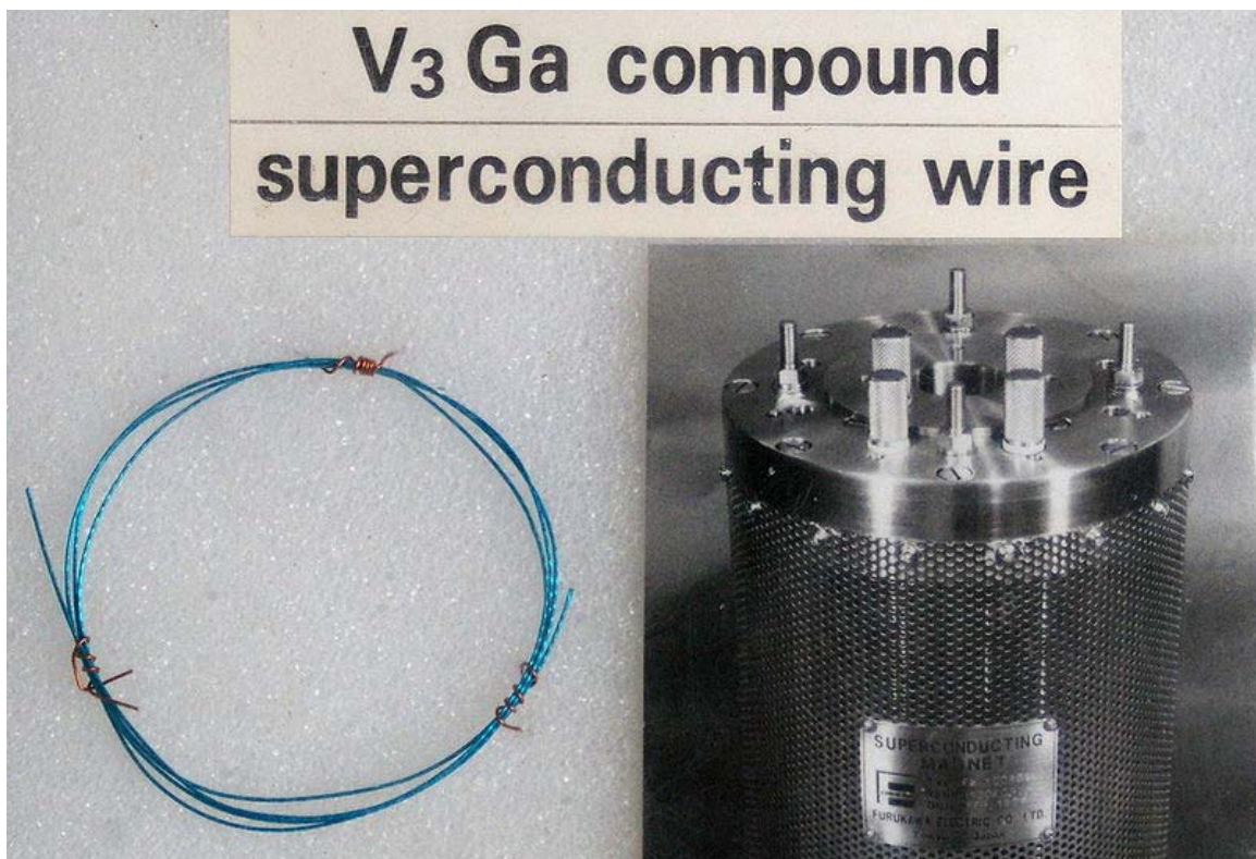
An example of a wire ( V_3Ga alloy) used in a superconducting magnet.
