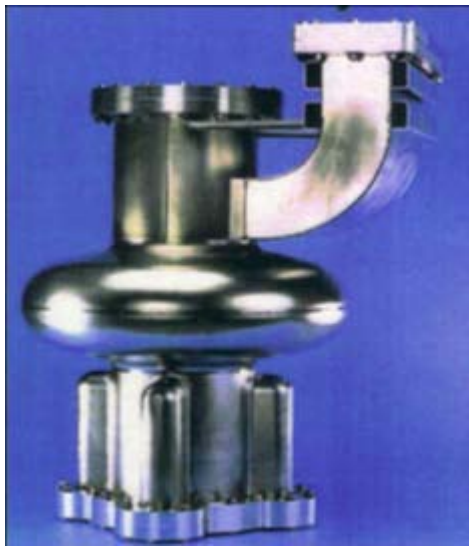
The Cornell storage ring 500 MHz SRF cavity.
