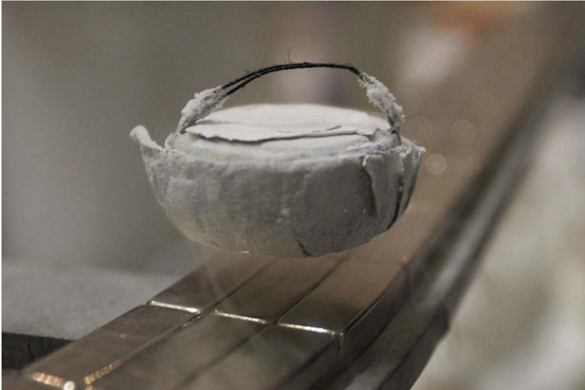
A high-temperature superconductor levitating above a magnet
