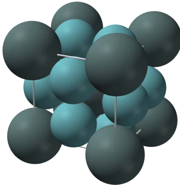
Unity cell of the A15 phases of Nb 3 Sn
