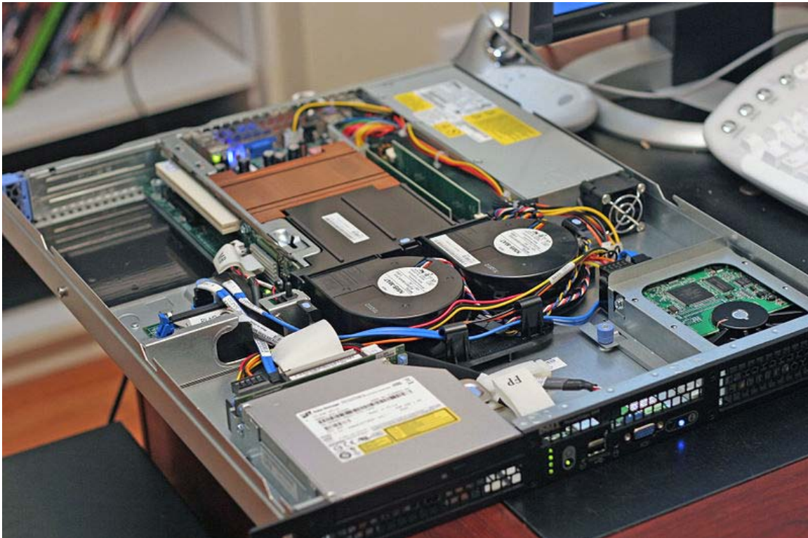
The inside and front of a Dell PowerEdge Web server
