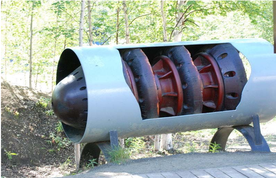
A pig on display in a section of cutaway pipe, from the Alaska Pipeline
