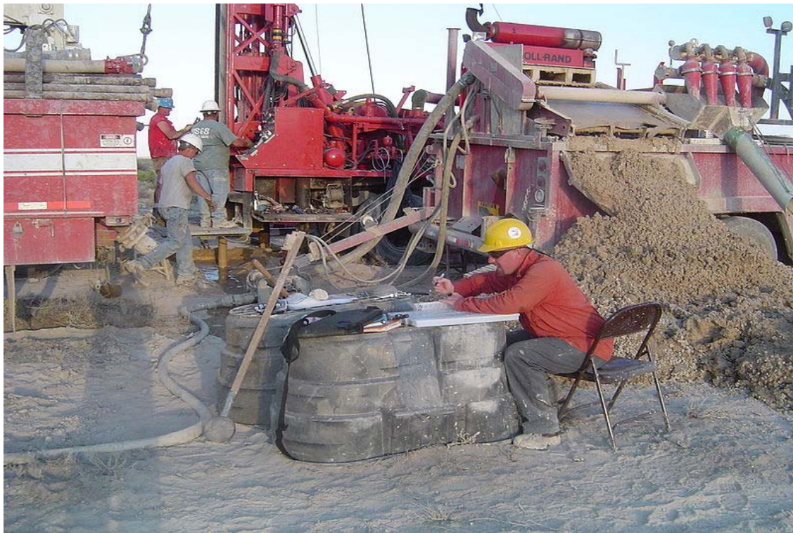
Mud log in process, a common way to study the lithology when drilling oil wells.
