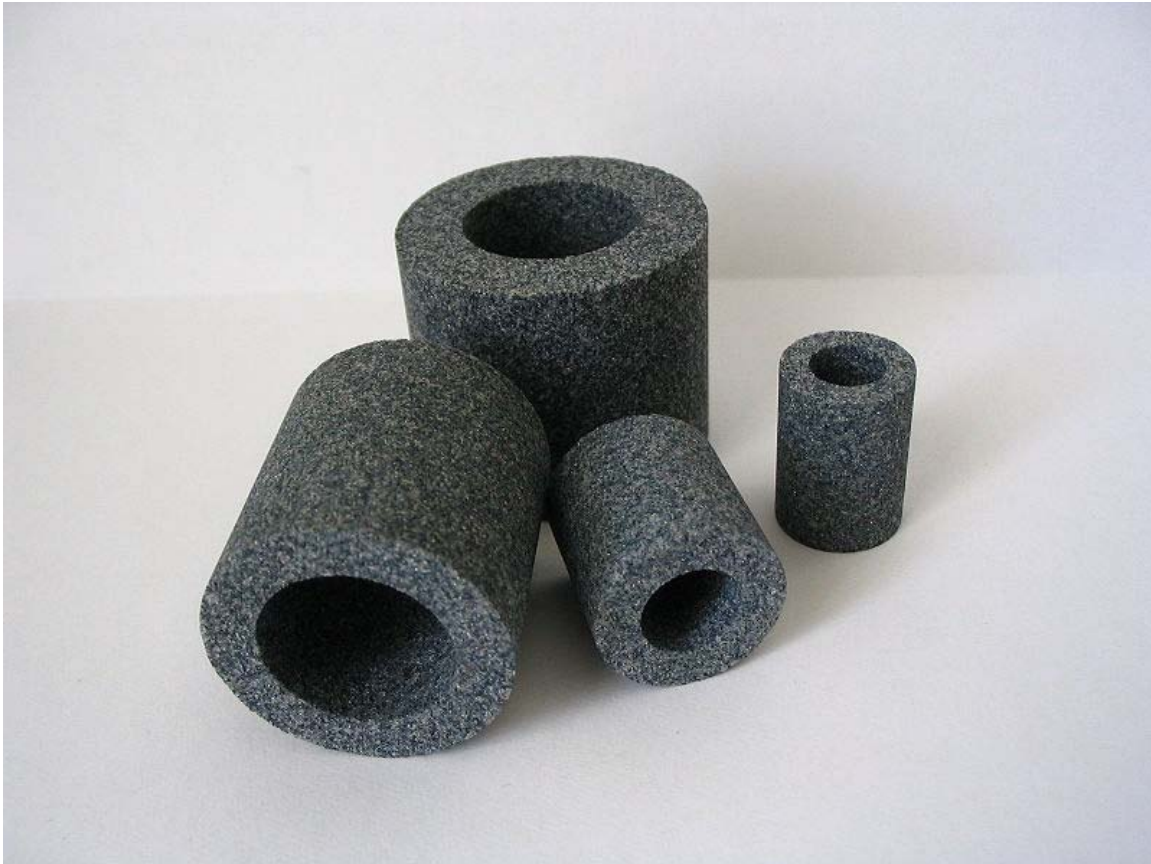
Assorted grinding wheels as examples of bonded abrasives.
