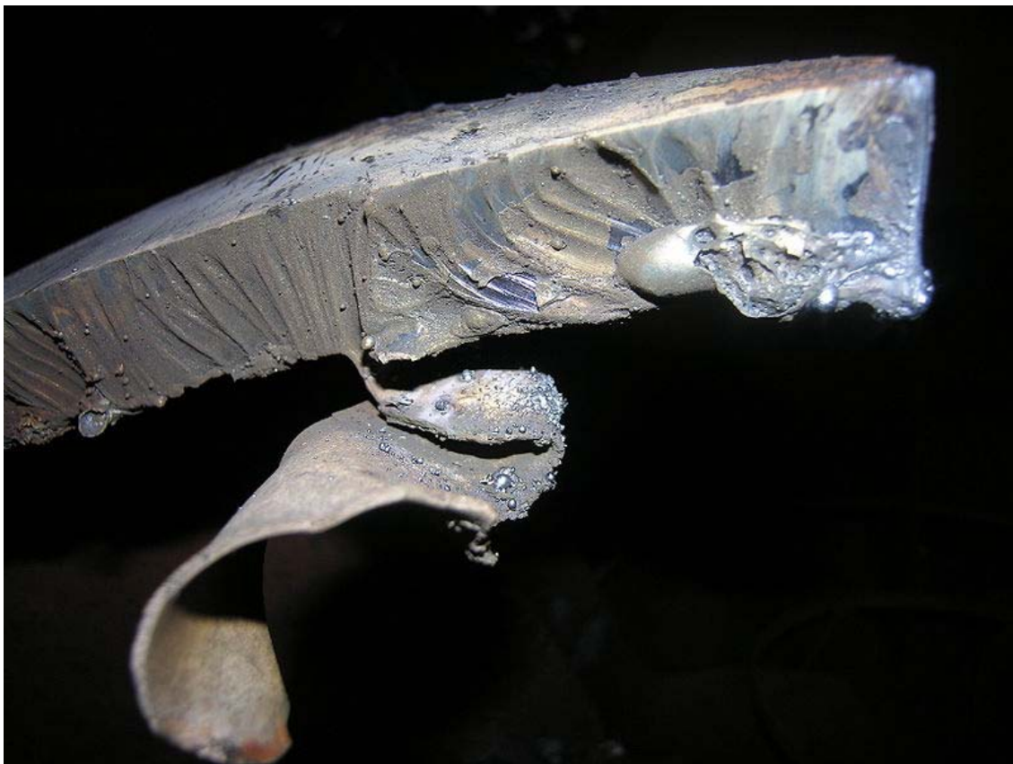
Side of metal, cut by oxygen - propane cutting torch
