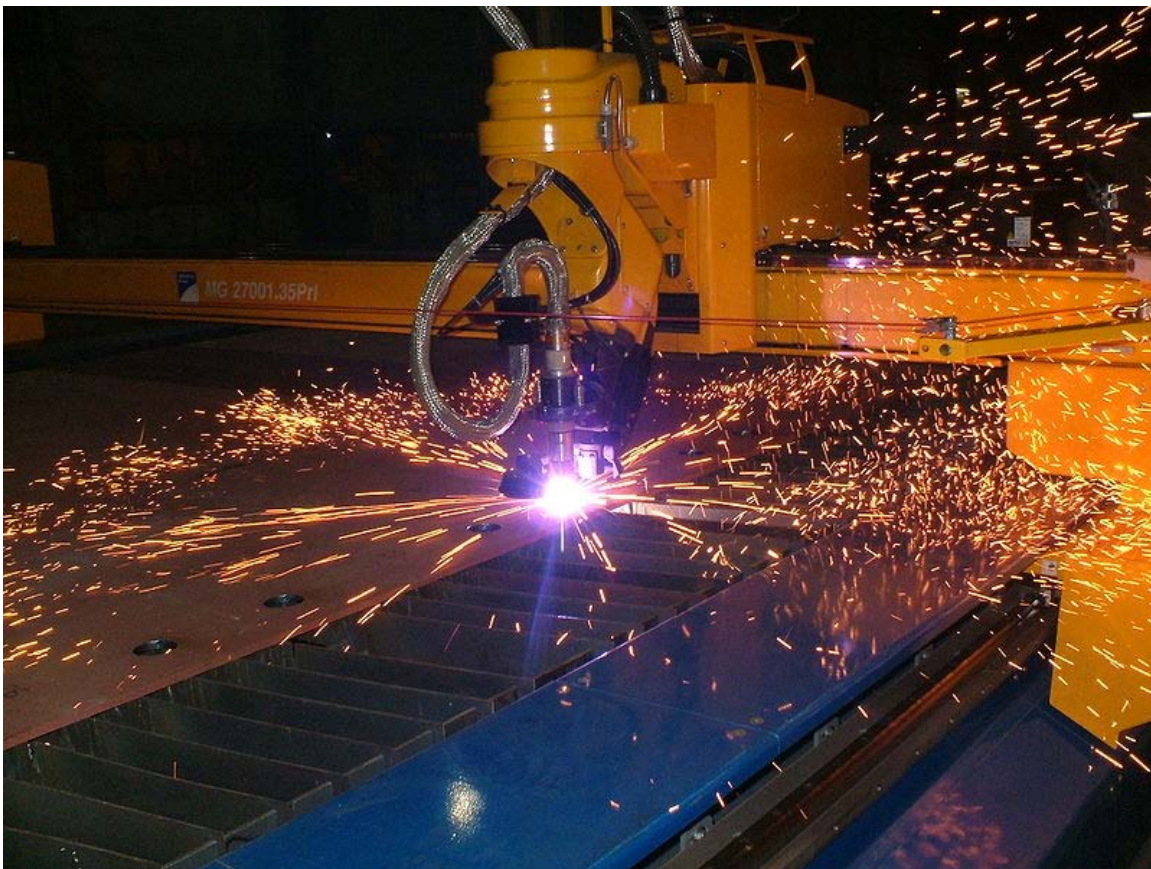
A CNC plasma cutting machining
