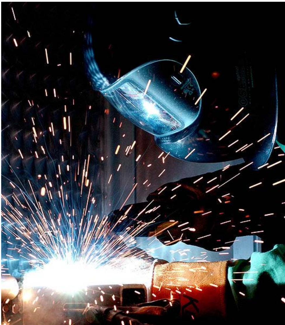
Gas metal arc welding
