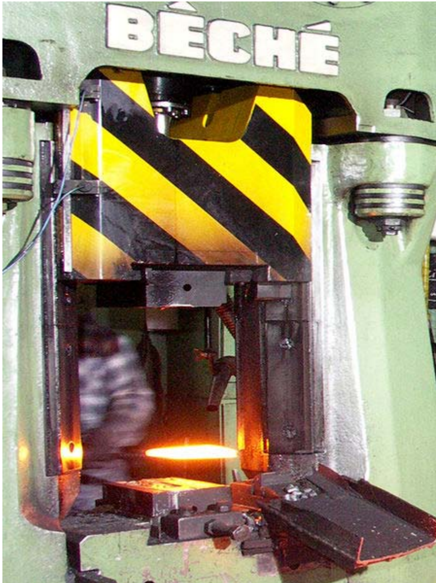
A red-hot metal workpiece is inserted into a forging press.
