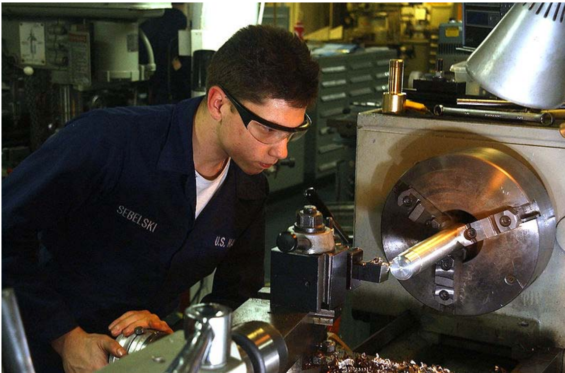
Machining a bar of metal on a lathe.
