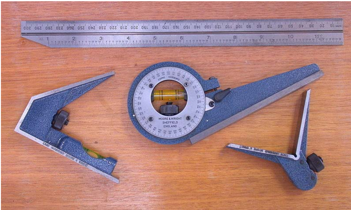
A combination square used for transferring designs.
