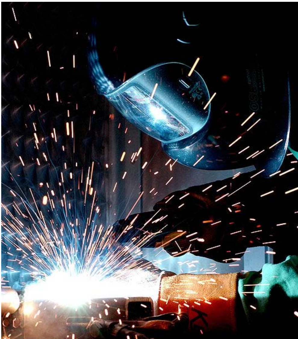
Gas metal arc welding
