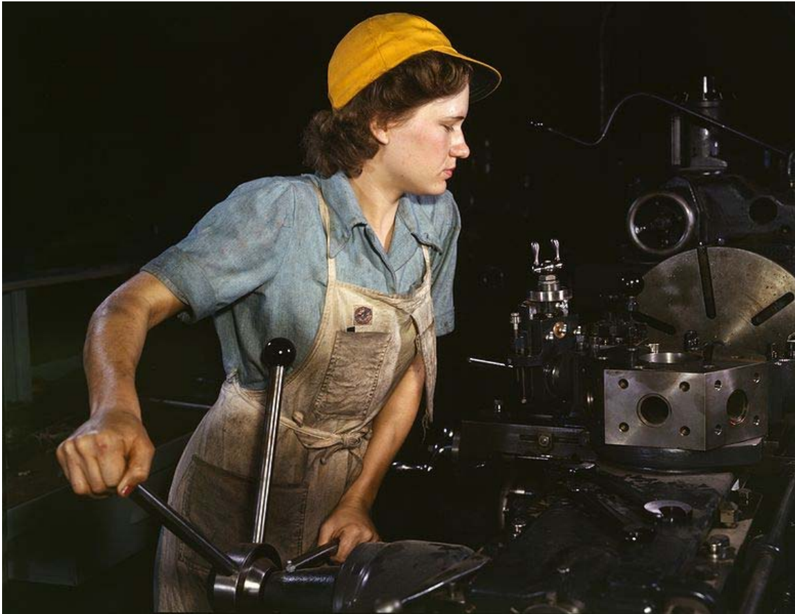
A turret lathe operator machining parts for transport planes at the Consolidated Aircraft Corporation plant, Fort Worth, Texas, USA in the 1940s.
