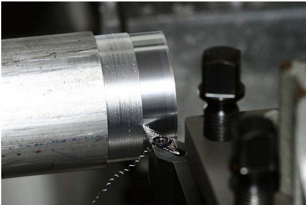
A lathe cutting material from a workpiece.
