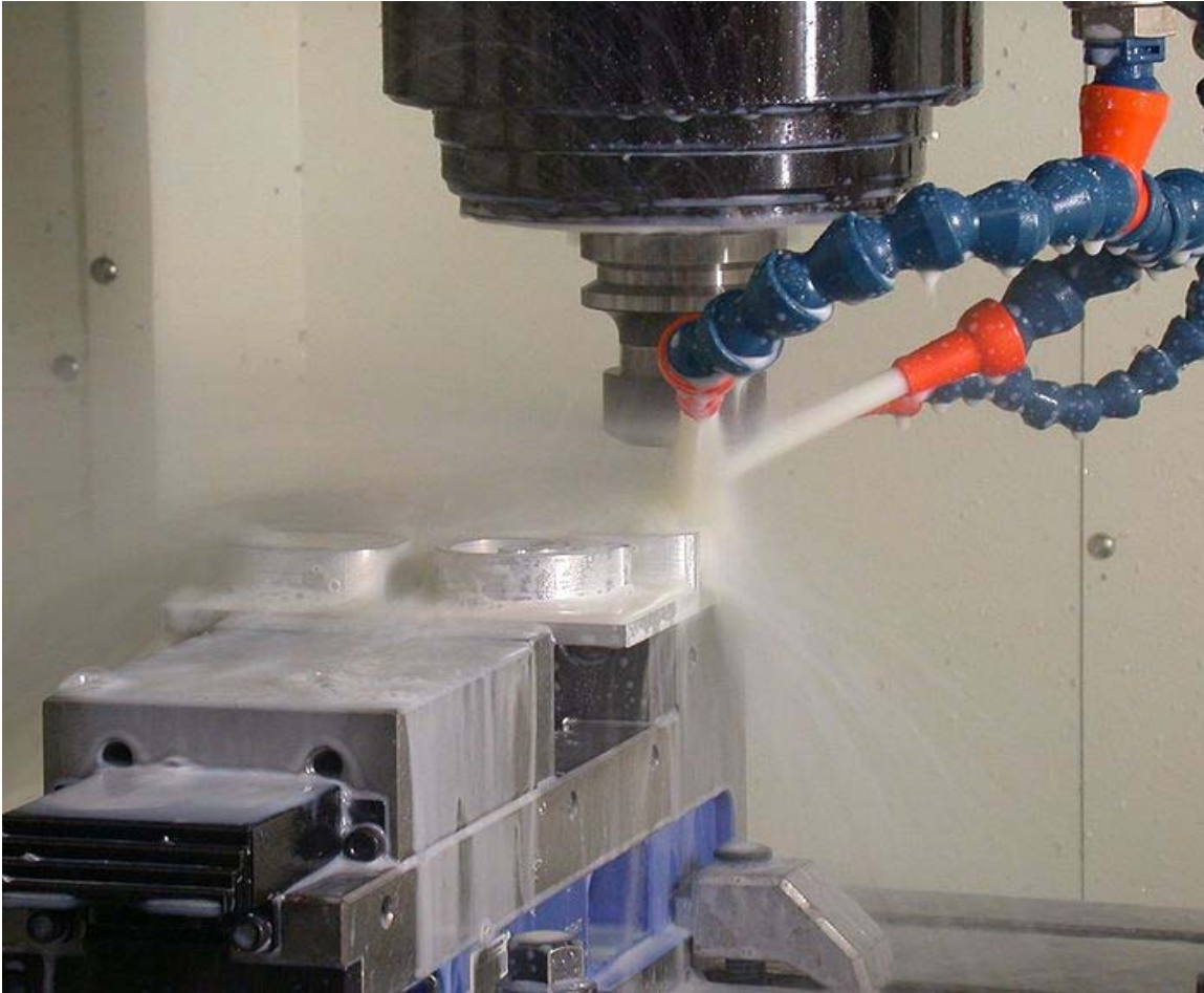
A milling machine in operation, including coolant hoses.
