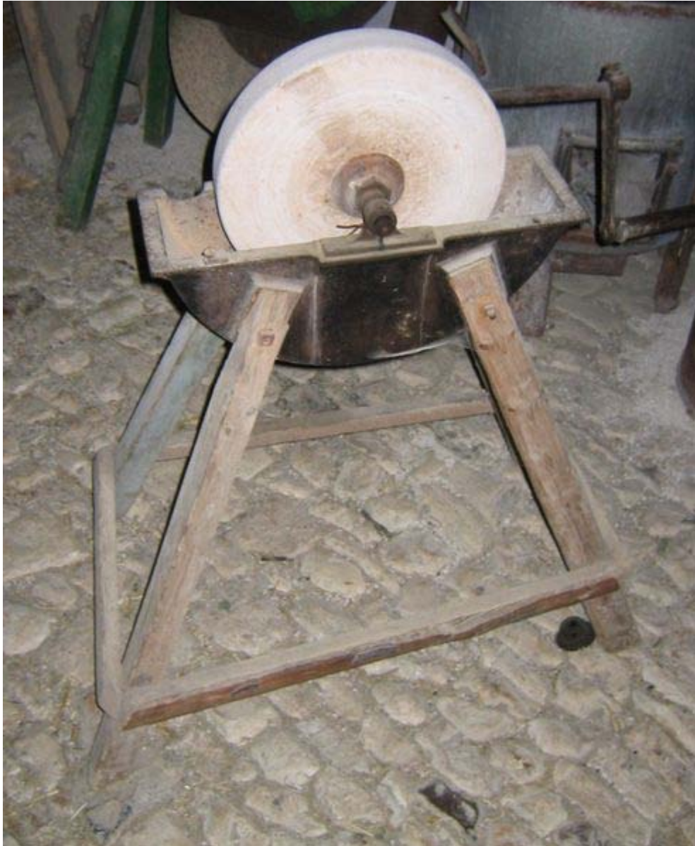
A grinding wheel with a reservoir to hold water as a lubricant and coolant.
