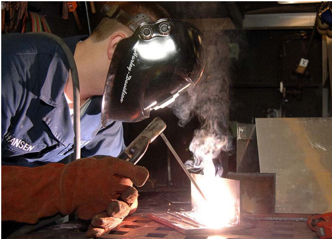
Shielded metal arc welding
