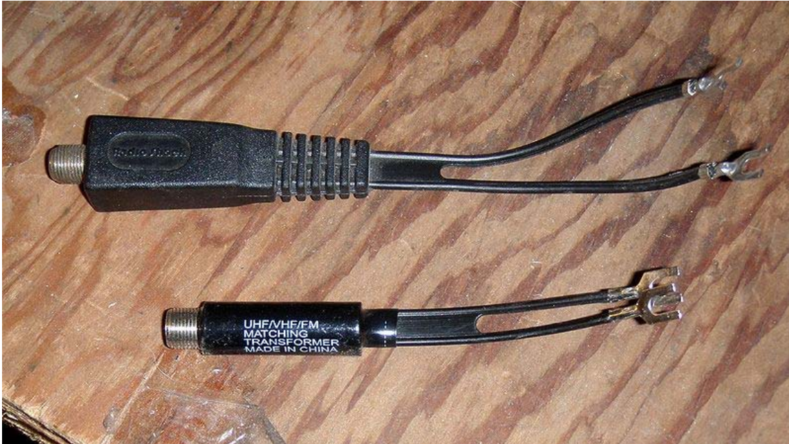
2 balun matching transformers
