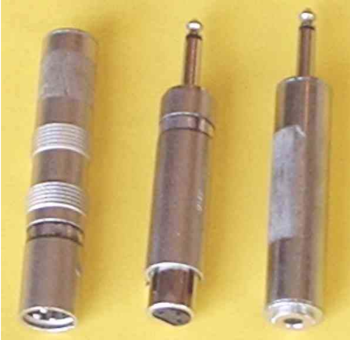
Three audio baluns (transformers).
