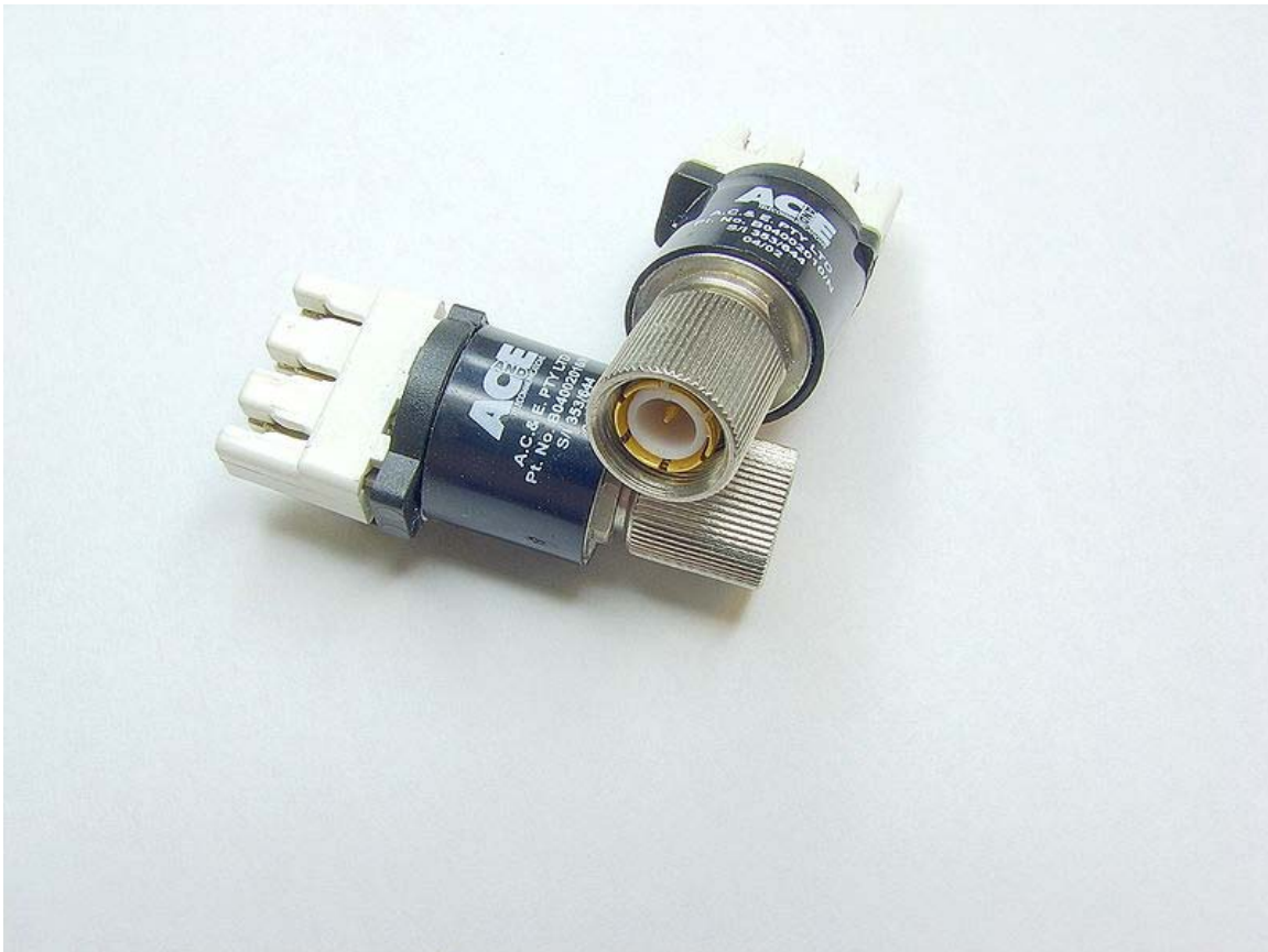
Pair of AC&E 120 Ohm twisted pair (Krone IDC) to 75 Ohm coaxial cable balun transformers. Actual length is about 3cm.
