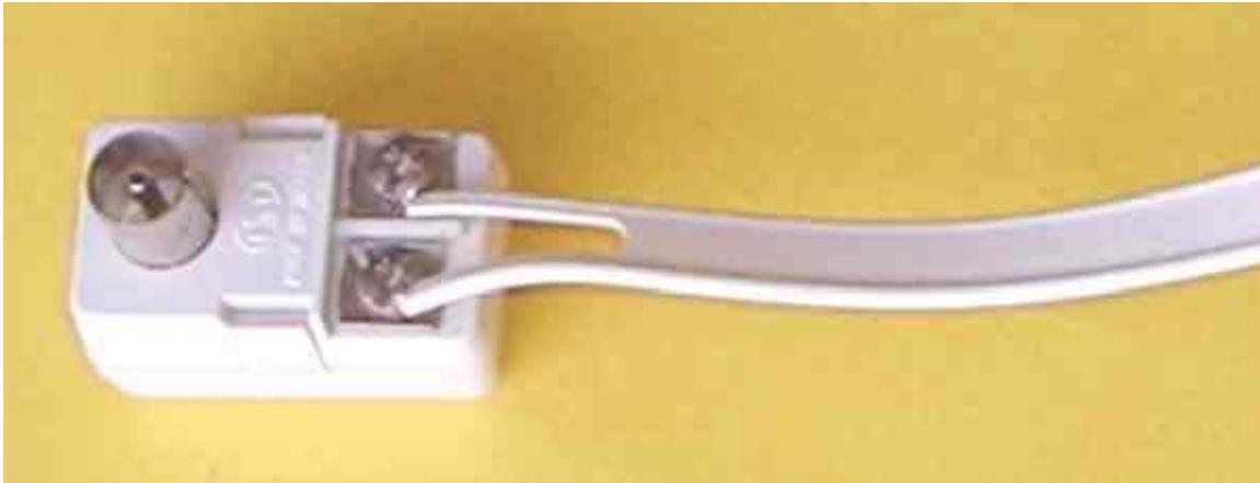
A 75-to-300 ohm balun built into the antenna plug.
