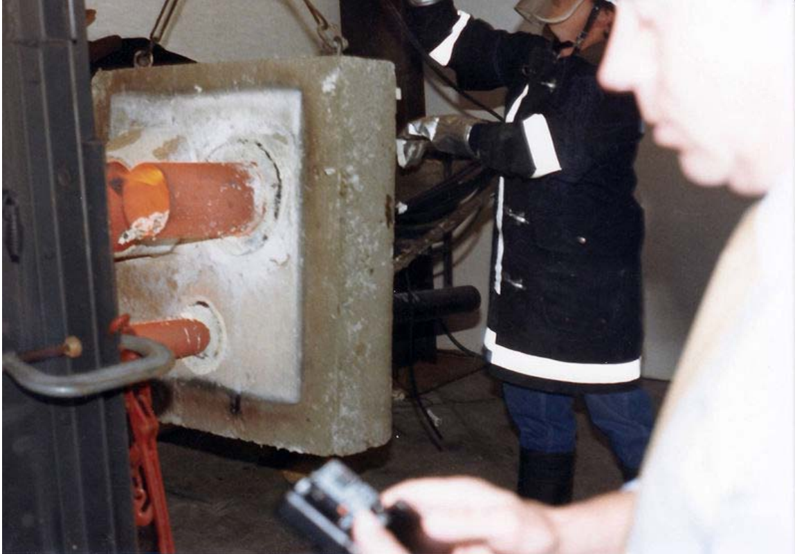
Heat exposure as part of a fire test for firestop products
