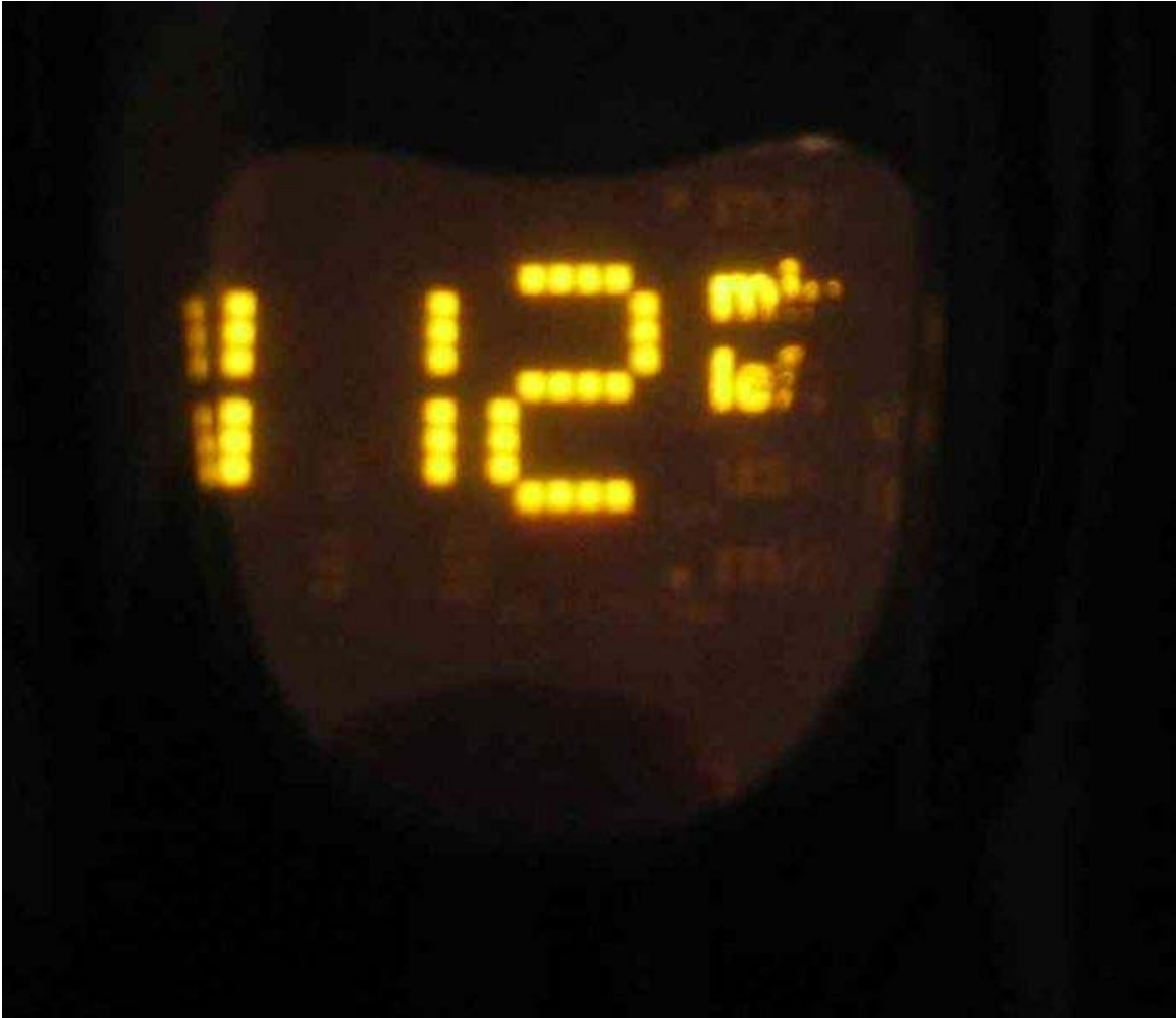
LEP display showing partial failure
