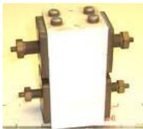
Voltage-controlled switch, a molecular electronic device from 1974. From Smithsonian Chip collection
