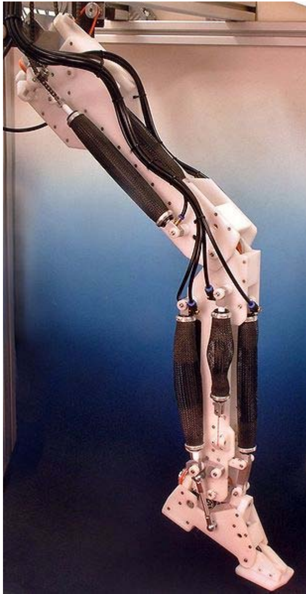
A robotic leg powered by Air Muscles
