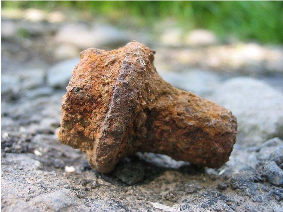
A rusted (and dirt-encrusted) bolt; note the surface pitting and gradual shape-deformation, caused by severe oxidation
