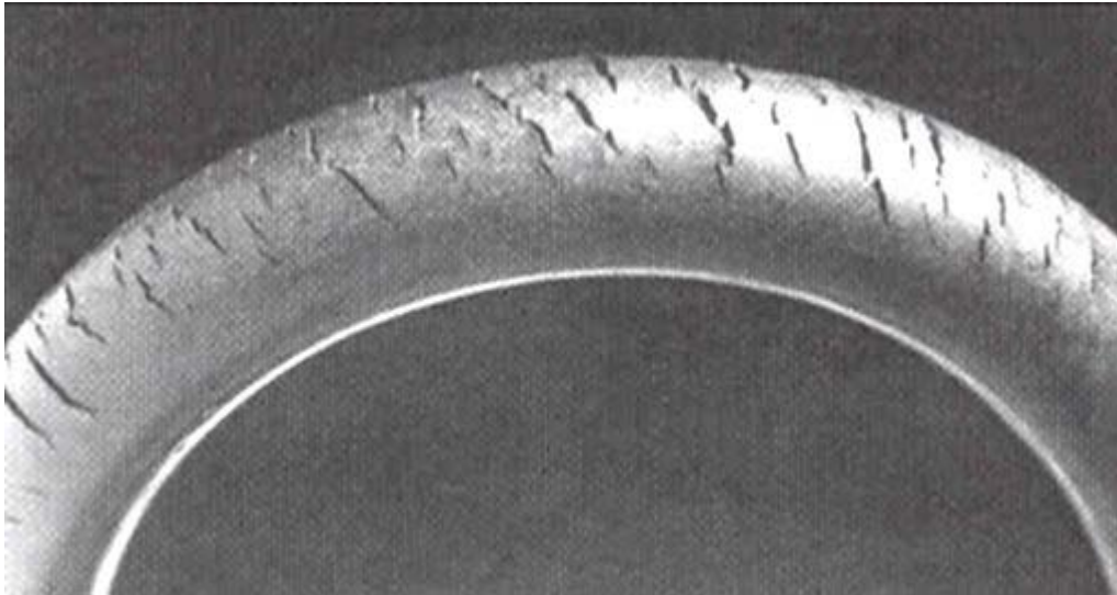
Ozone cracking in Natural rubber tubing
