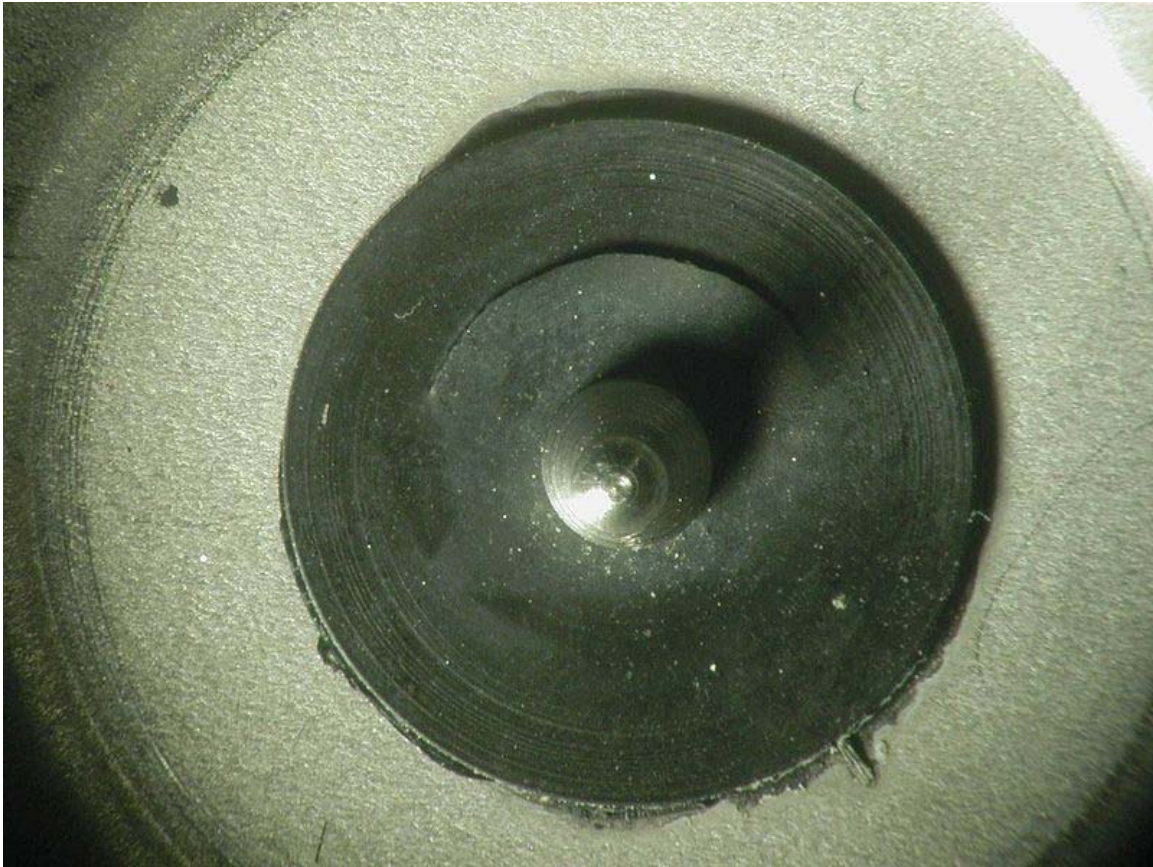
Macro photograph of ozone cracking in NBR (Nitrile Butadiene Rubber) diaphragm seal
