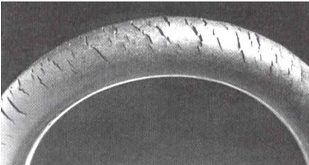
Ozone cracking in natural rubber tubing
