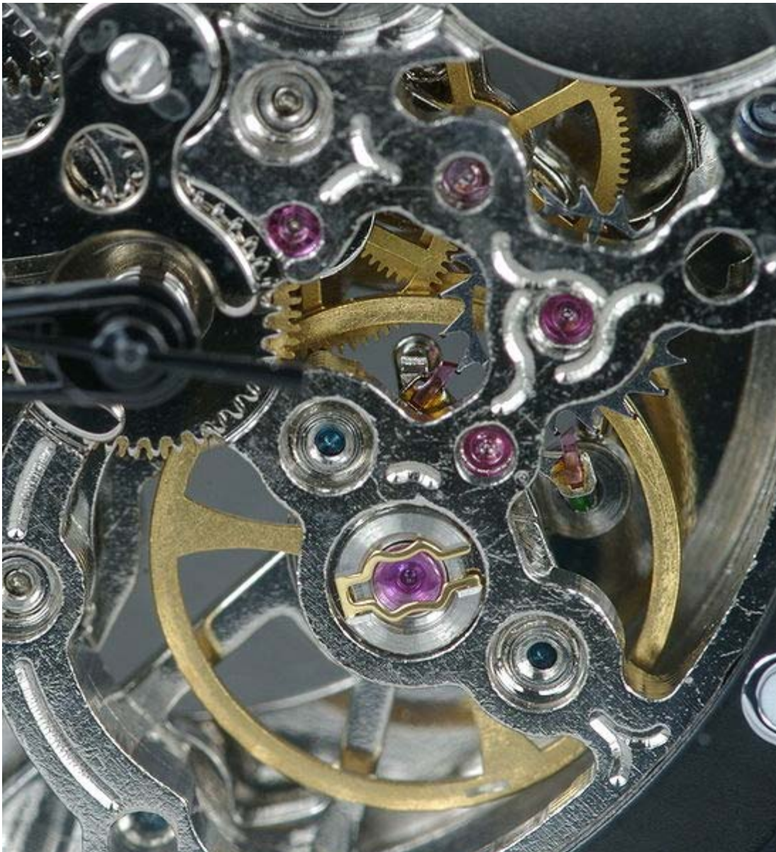
Ruby jewel bearings used for a balance wheel in a mechanical watch movement.
