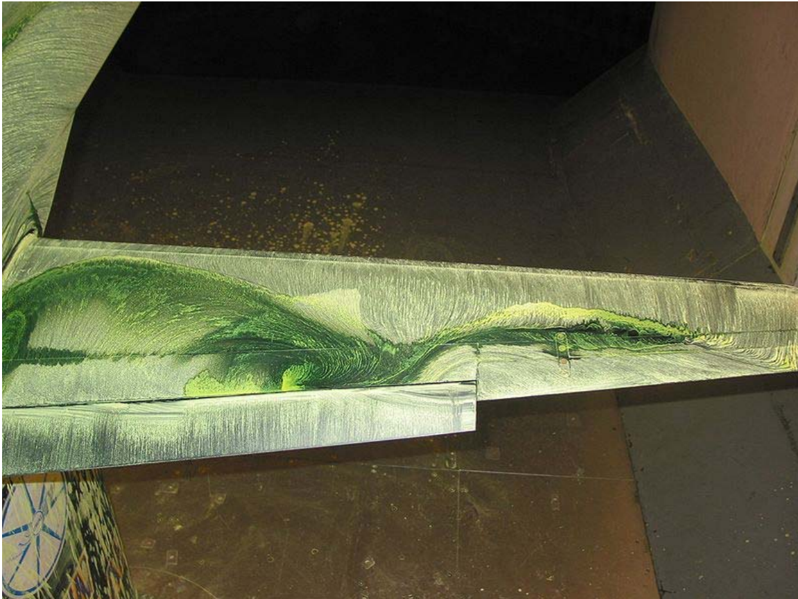
China clay on a wing in the Kirsten Wind Tunnel showing reverse and span-wise flow.
