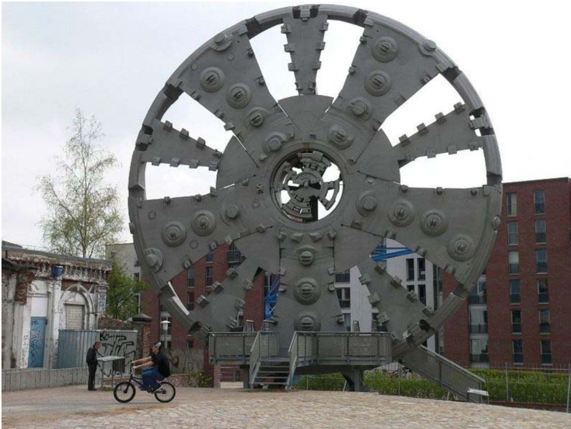
Cutting shield used for the New Elbe Tunnel.
