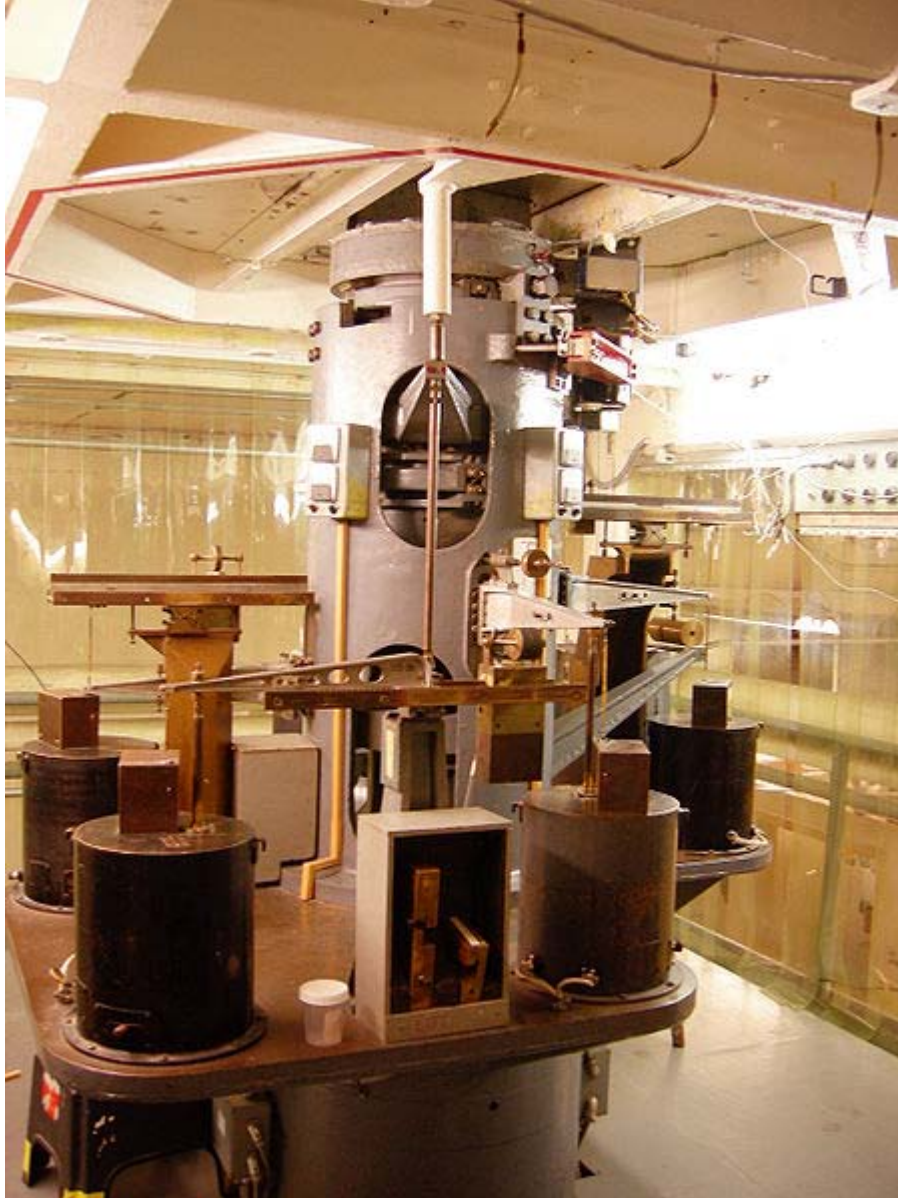
Six-element external balance below the Kirsten Wind Tunnel
