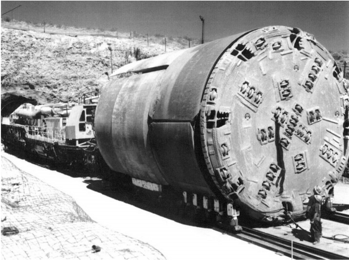
A tunnel boring machine that was used at Yucca Mountain, Nevada, United States
