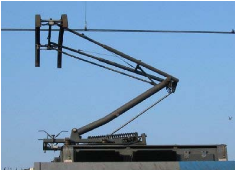
A modern pantograph. The device shown is technically a half-pantograph.
