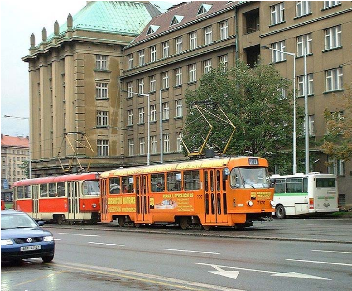
Symmetrical, diamond 0073haped pantographs on trams in Prague.
