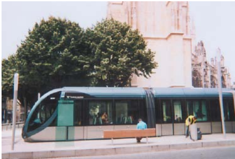
Bordeaux trams run without overhead wires
