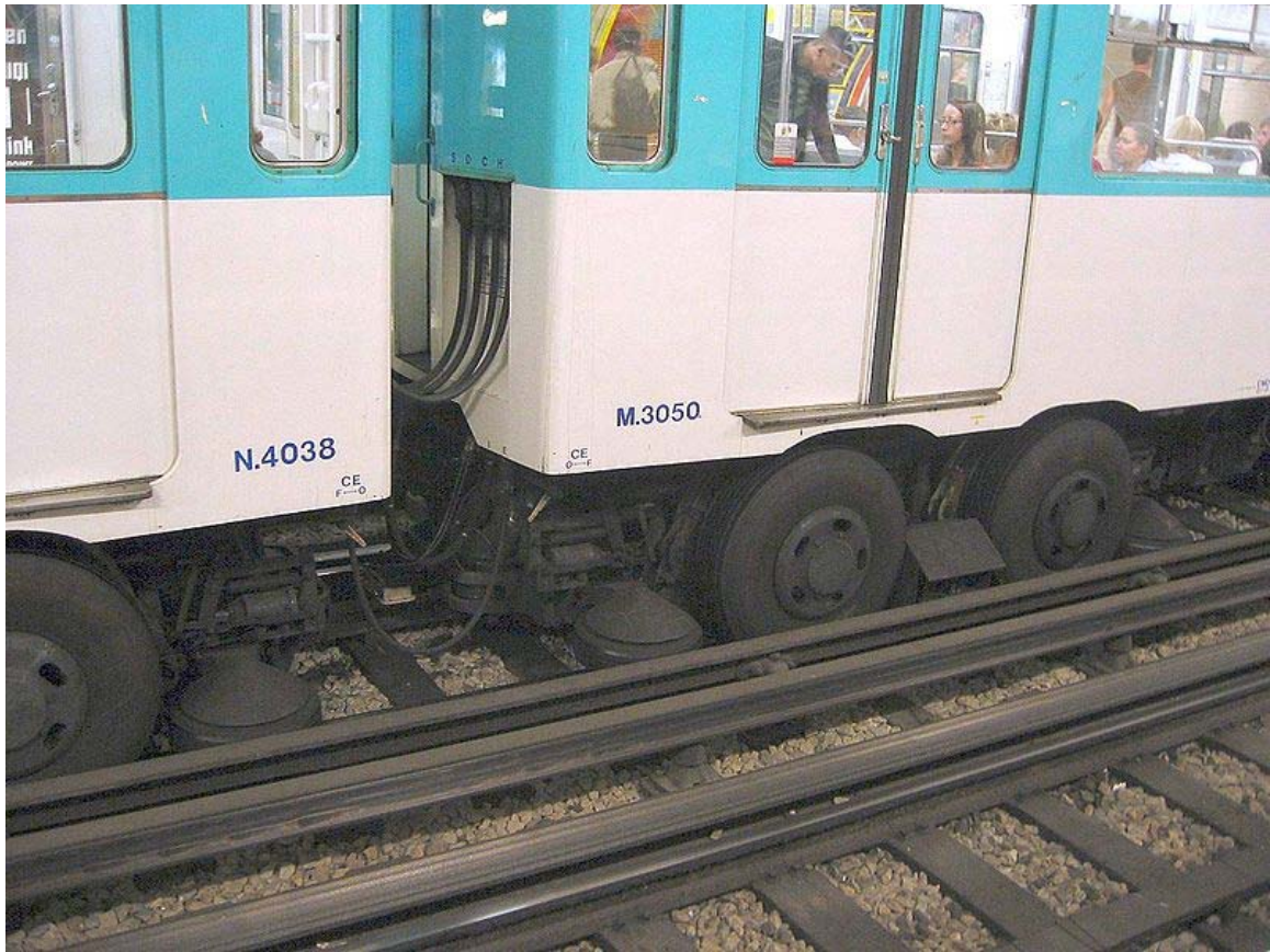
Paris Metro. The guiding rails of the rubber-tyred lines are also current conductors. The current collector is between the pair of rubber wheels.
