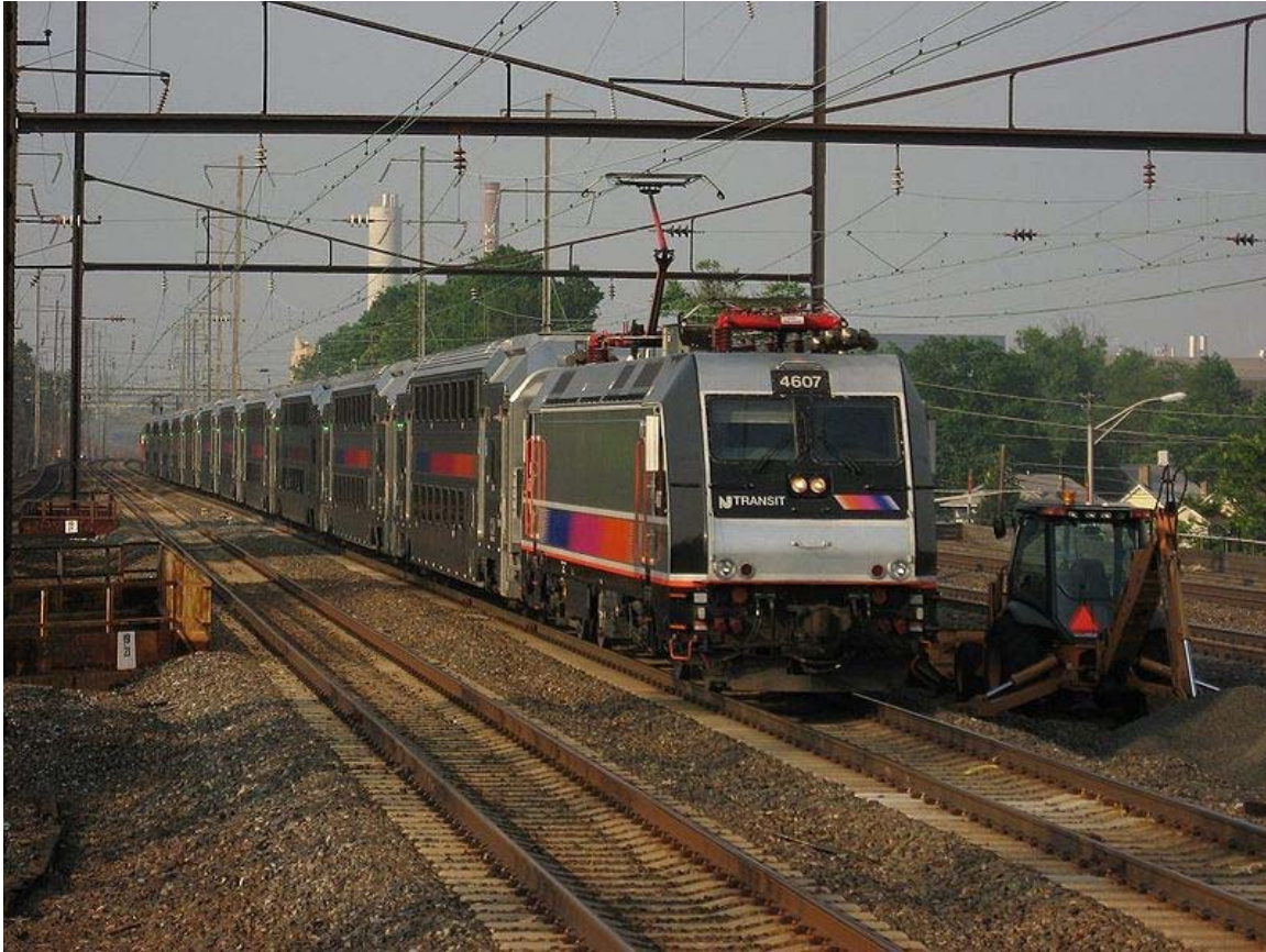
New Jersey Transit ALP-46 AC locomotive based on the DBAG Class 101
