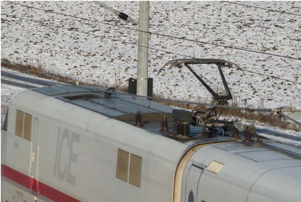
High-performance pantograph for measurements on the ICE S
