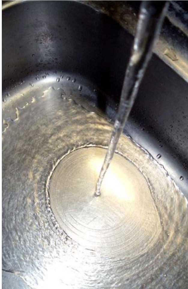
Figure 2: A common example of a hydraulic jump is the roughly circular stationary wave that forms around the central stream of water. The jump is at the transition between the point where the circle appears still and where the turbulence is visible.
