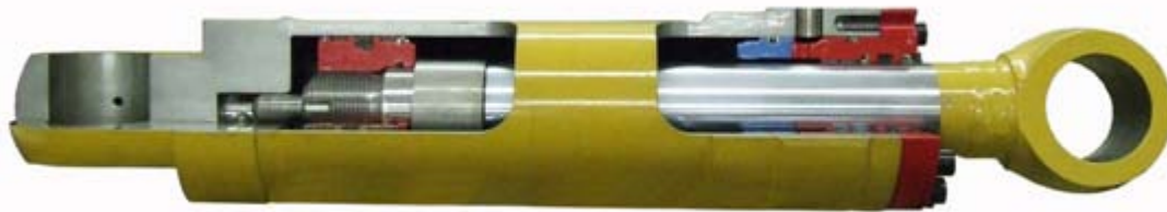
A Cut Away of a Welded Body Hydraulic Cylinder showing the internal components
