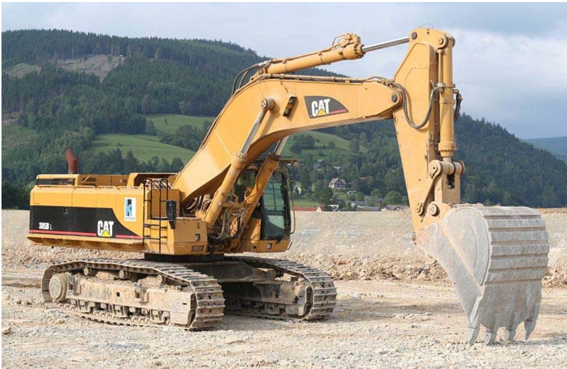
An excavator; main hydraulics: Boom cylinders, swingdrive, cooler fan and trackdrive
