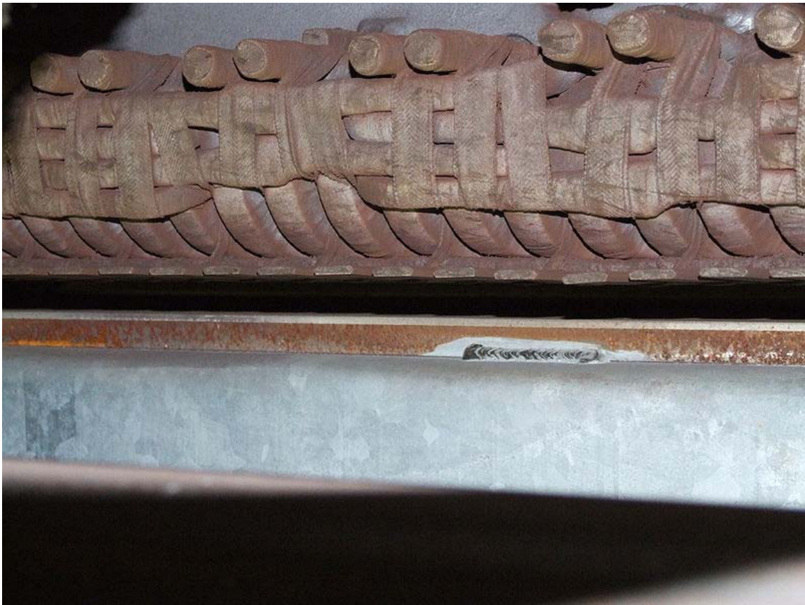
A linear motor for trains running Toei Oedo line
