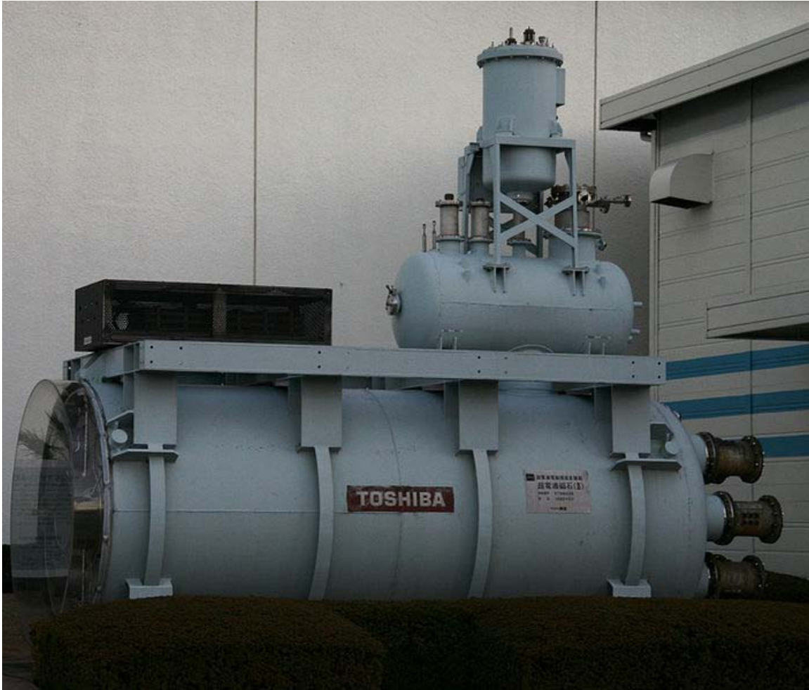
A MHD thruster from the boat, at the Ship Science Museum in Tokyo.
