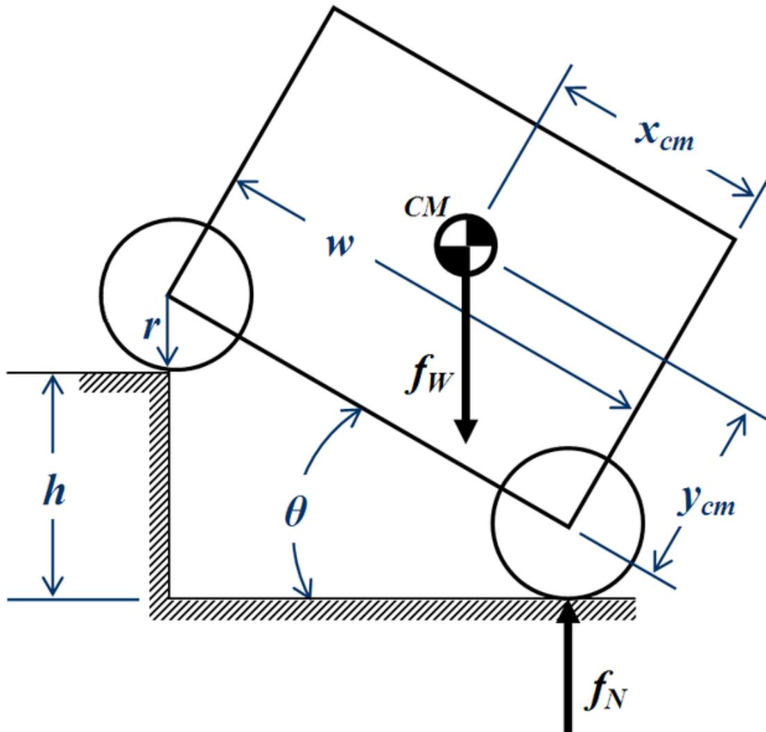
Static stability of a wheeled vehicle
