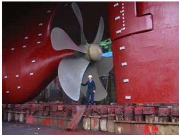
Propeller on a modern mid-sized merchant vessel
