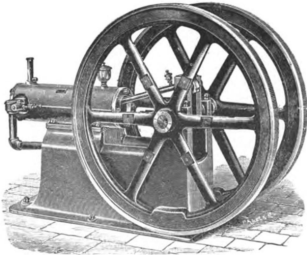
1898 illustration of a White and Middleton stationary engine; note the large twin flywheels
