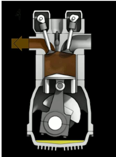
the four stages of the 4-stroke combustion engine cycle:
