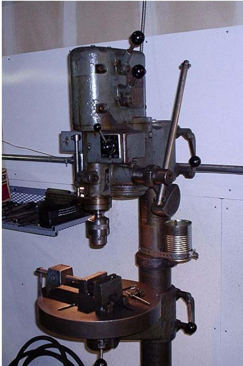
Geared head drill press. Shift levers on the head and a two speed motor control immediately in front of the quill handle select one of eight possible speeds
