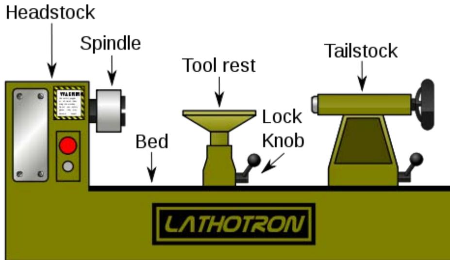
Parts of a wood lathe
