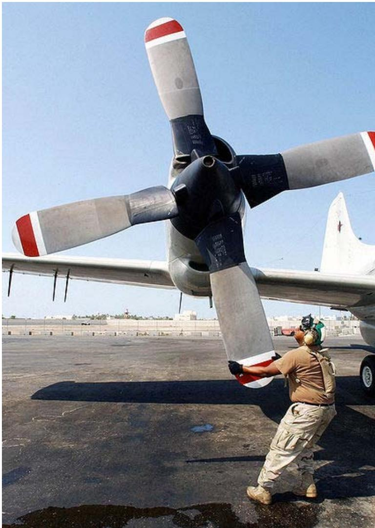
Rotating the Hamilton Standard 54H60 propeller on a US Navy EP-3E Orion's number four engine as part of pre-flight checks
