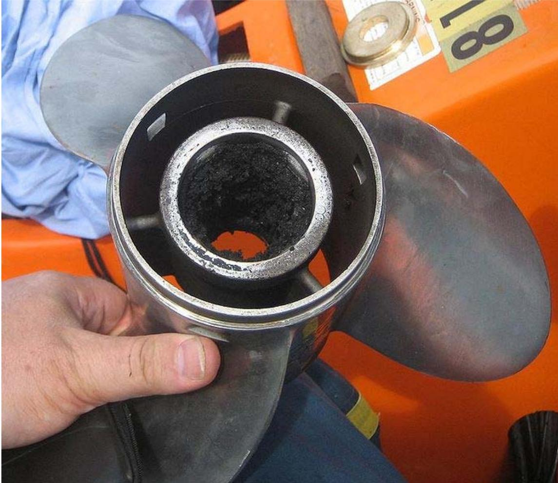
A failed rubber bushing in an outboard's propeller
