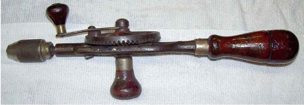
An old hand drill or "eggbeater" drill. The hollow wooden handle, with screw-on cap, is used to store drill bits
