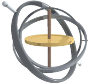
A gyroscope in operation with freedom in all three axes. The rotor will maintain its spin axis direction regardless of the orientation of the outer frame.
