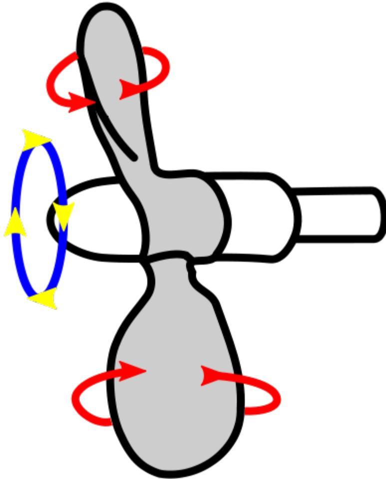
A controllable pitch propeller
