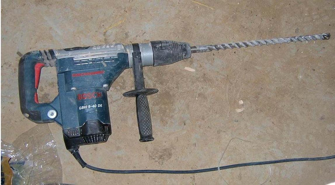
A rotary hammer drill used in construction
