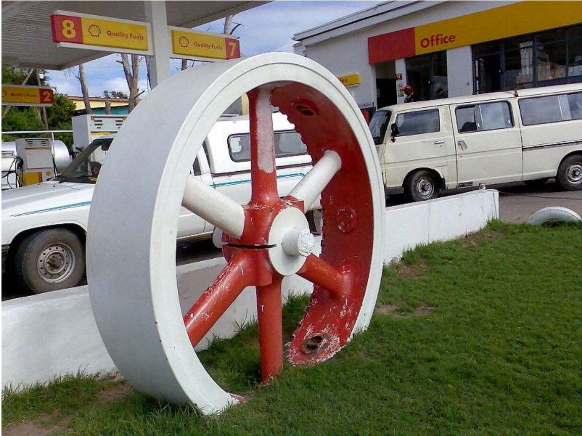
Flywheel from stationary engine. Note the castellated rim which was used to rotate the engine to the correct starting position by means of a lever
