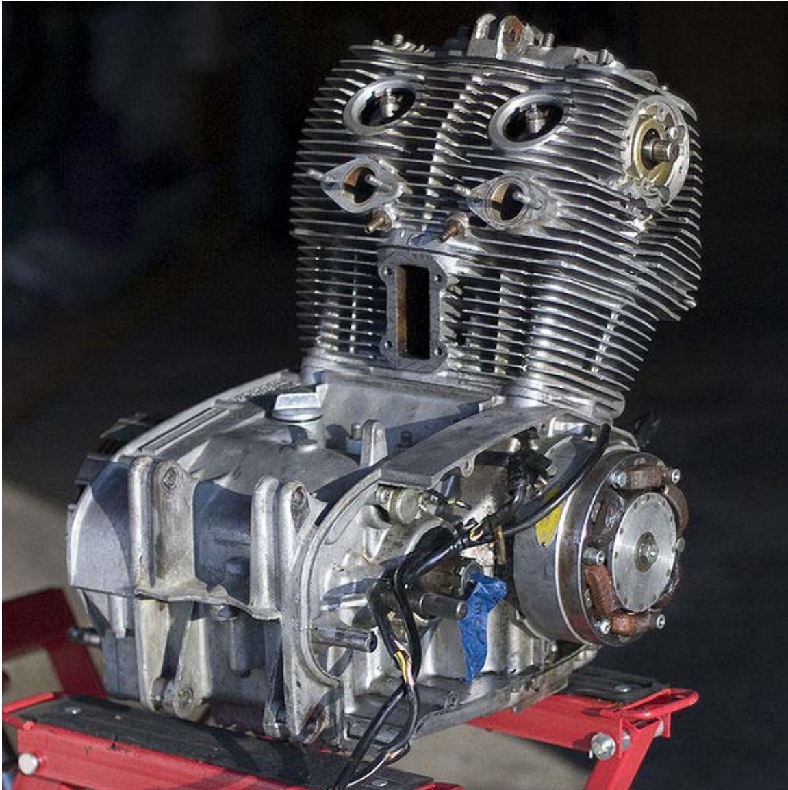
1962 Honda CB77 Superhawk 305 cc (18.6 cu in) twin engine.
