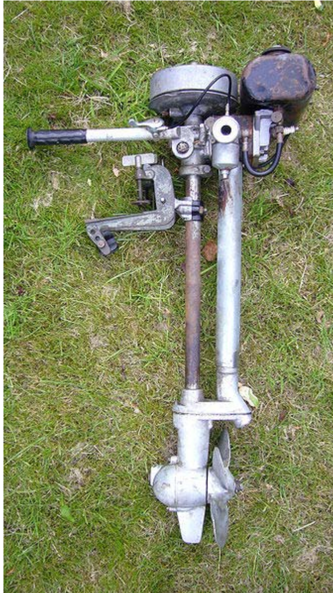
Lateral view of a two-stroke Forty series British Seagull outboard engine. The serial number dates it to 1954/1955
