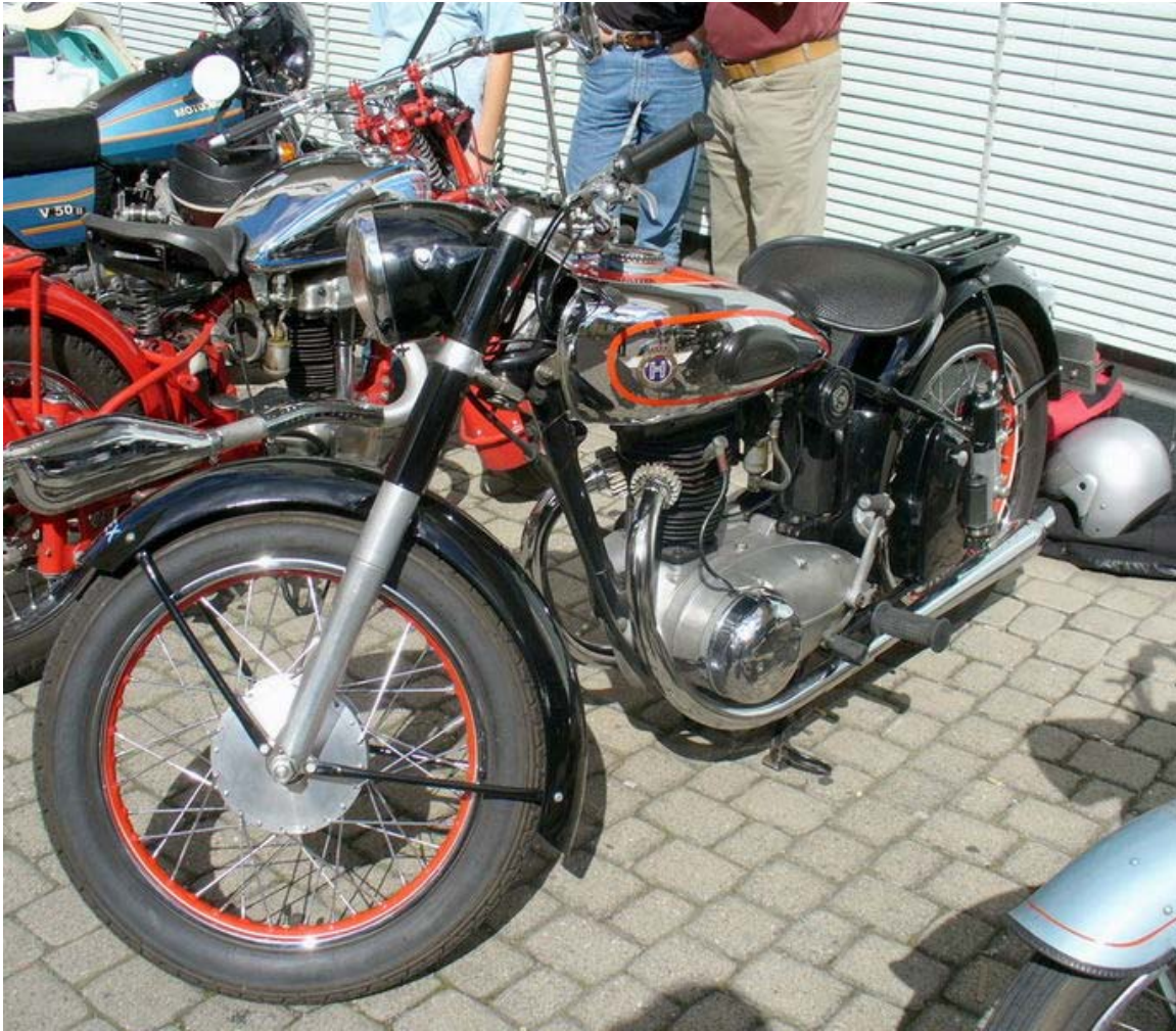
Motorbike Horex "Regina" with one-cylinder-four-stroke-engine
