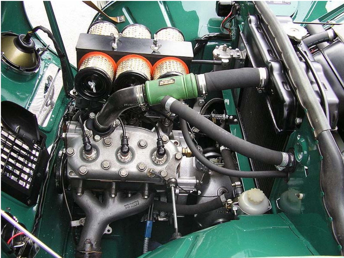
A tuned version of a Saab inline-three cylinder two-stroke engine
