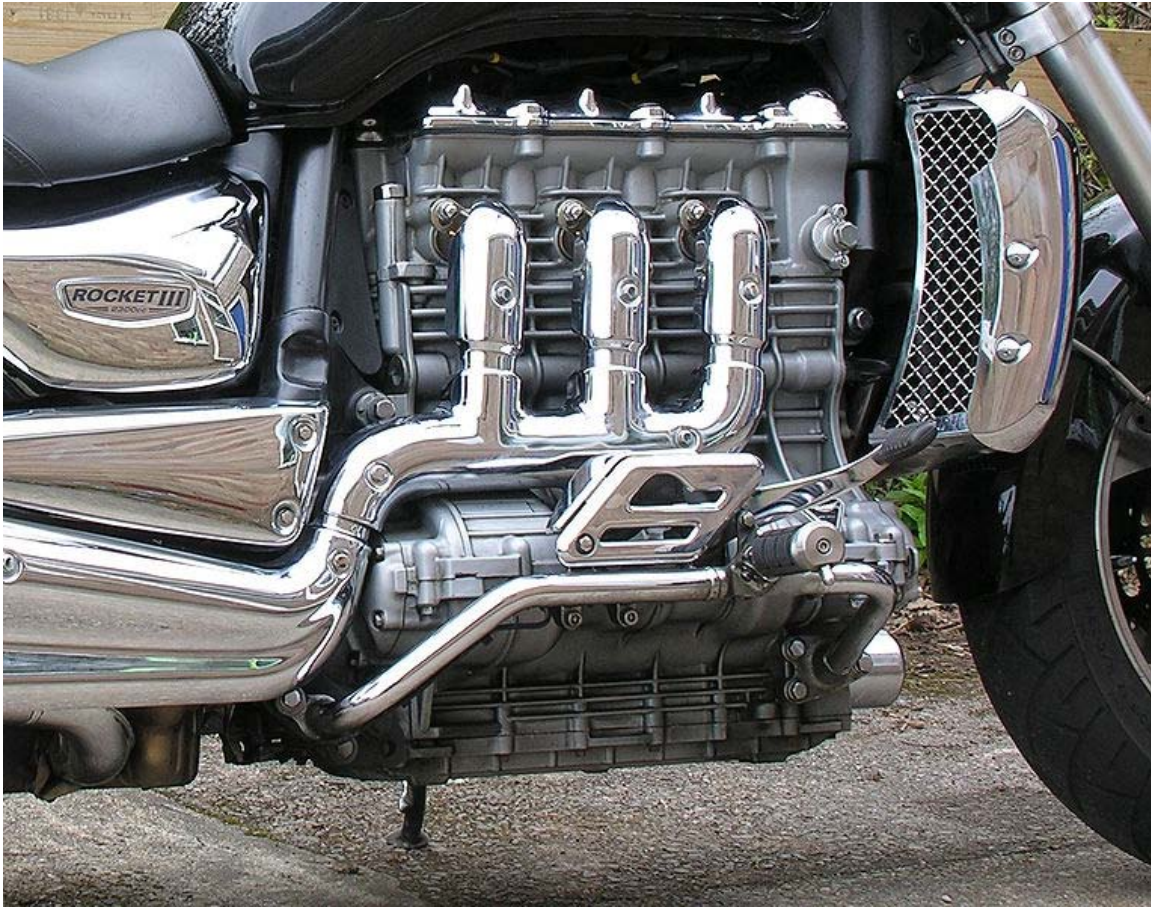
Triumph Rocket III has a 2.3 L straight-three engine
