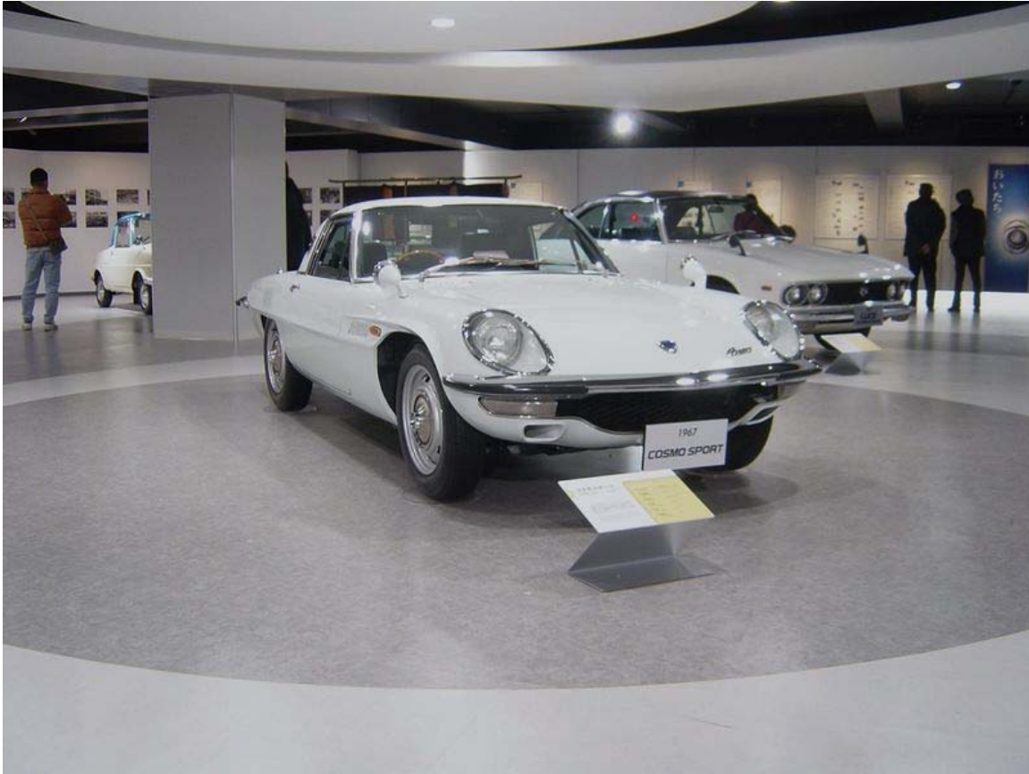
Mazda Cosmo , the first series two rotor Wankel engine sports car
