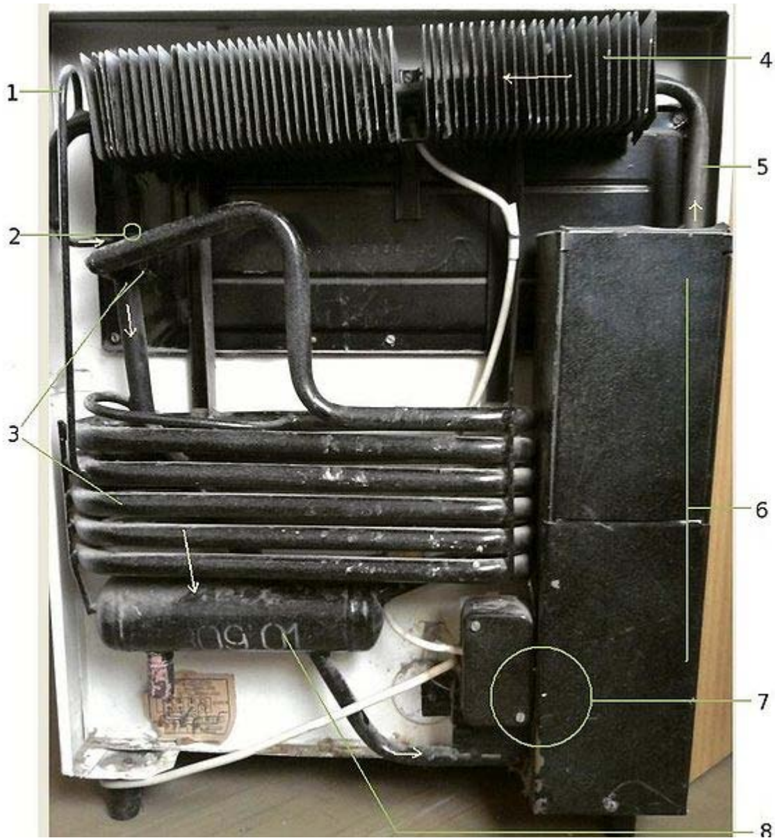
Labeled photo of a domestic absorption refrigerator.
