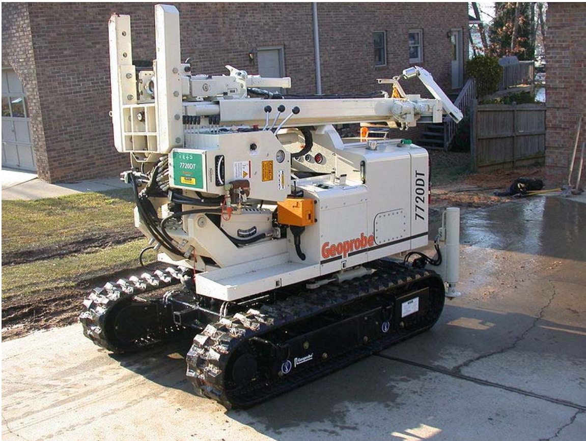
Typical drill rig for DX installation, length 8 ft
