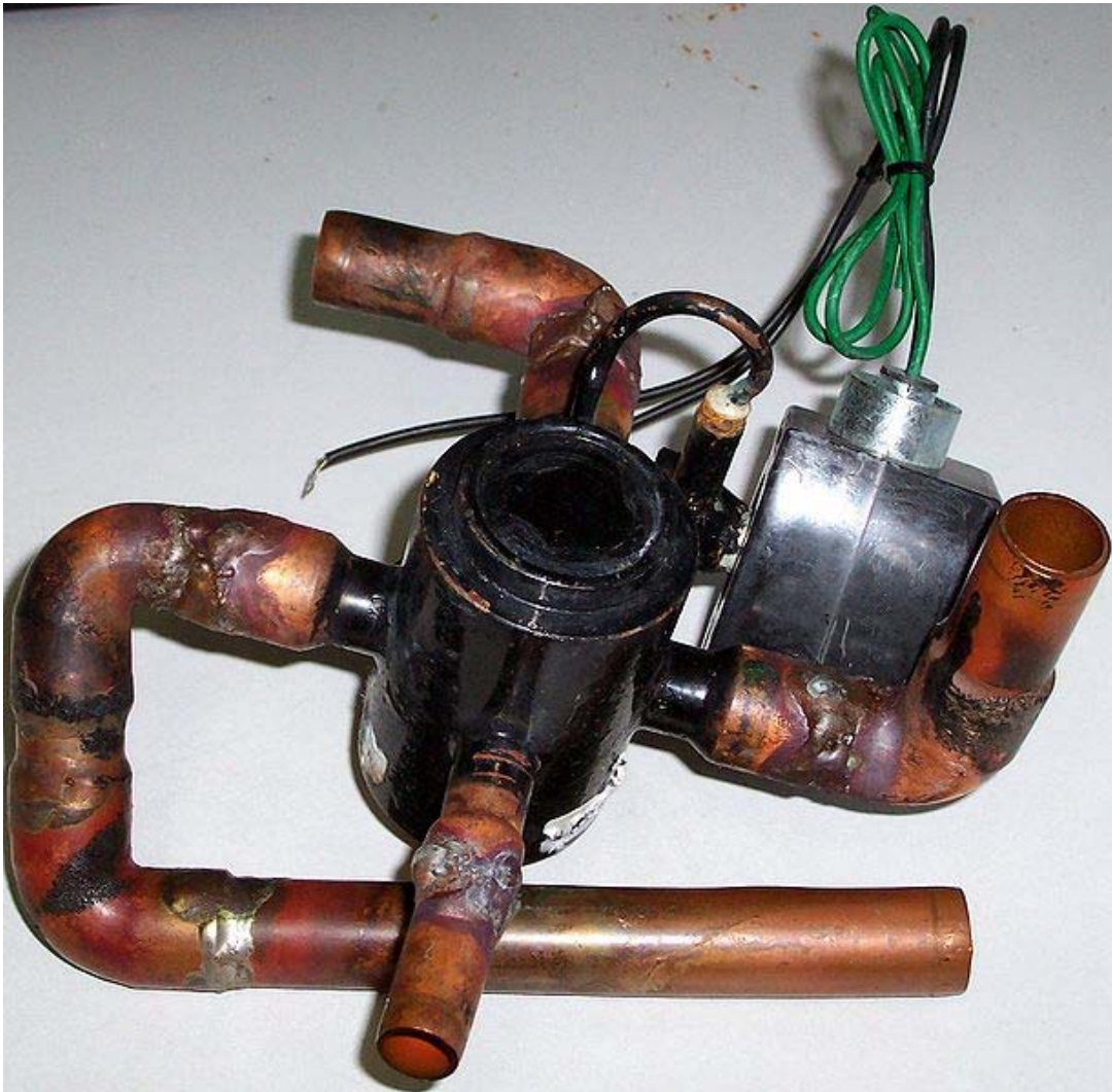
A reversing valve removed from an HVAC heat pump for replacement.
