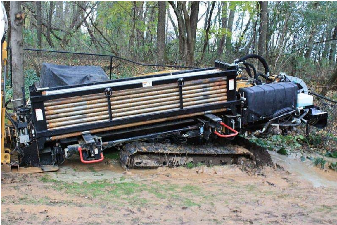
Geothermal drill machine.
