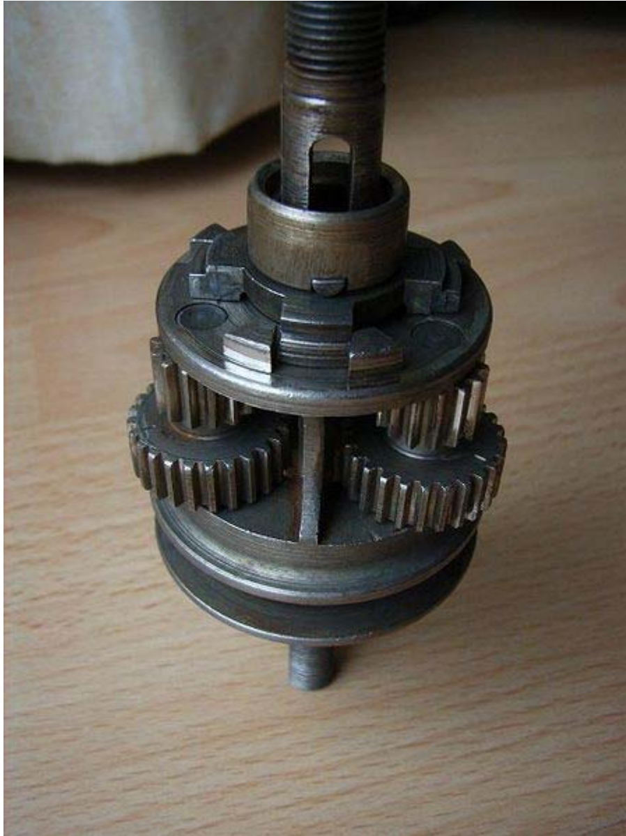
Compound planets of a Sturmey-Archer AM bicycle hub (gear ring removed)
