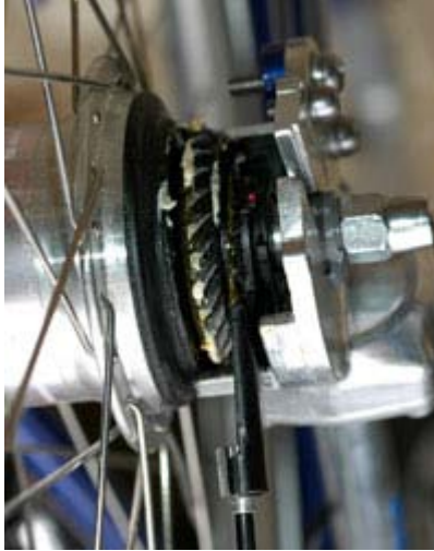
Bevel ring gear on the rear wheel of a shaft-driven bicycle
