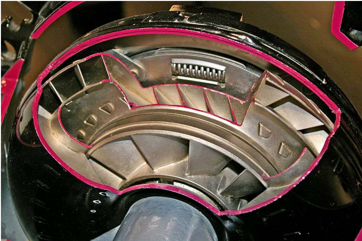
A cut-away model of a torque converter
