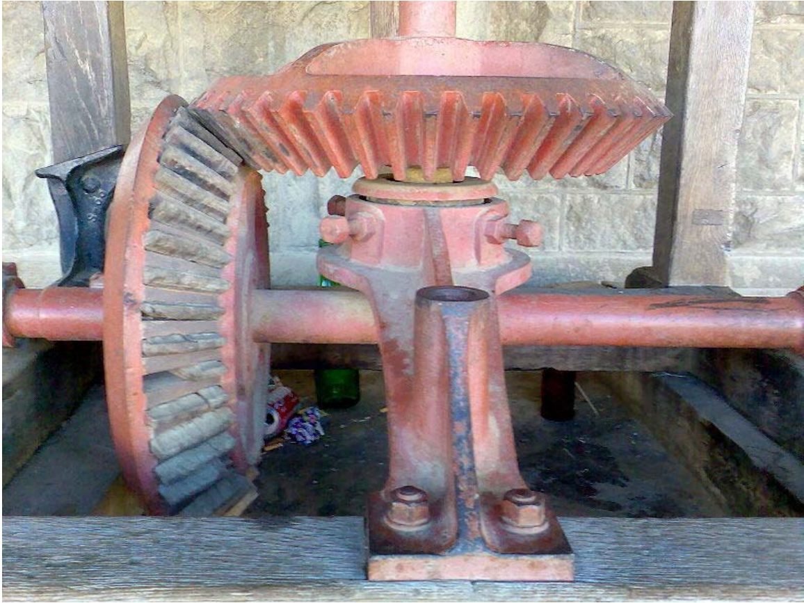
Bevel gears on grain mill at Dordrecht. Note wooden teeth inserts on one of the gears.
