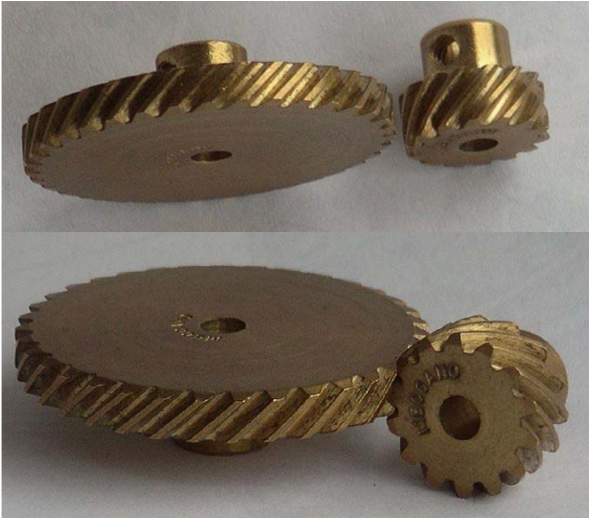
Helical gears Top: parallel configuration Bottom: crossed configuration
