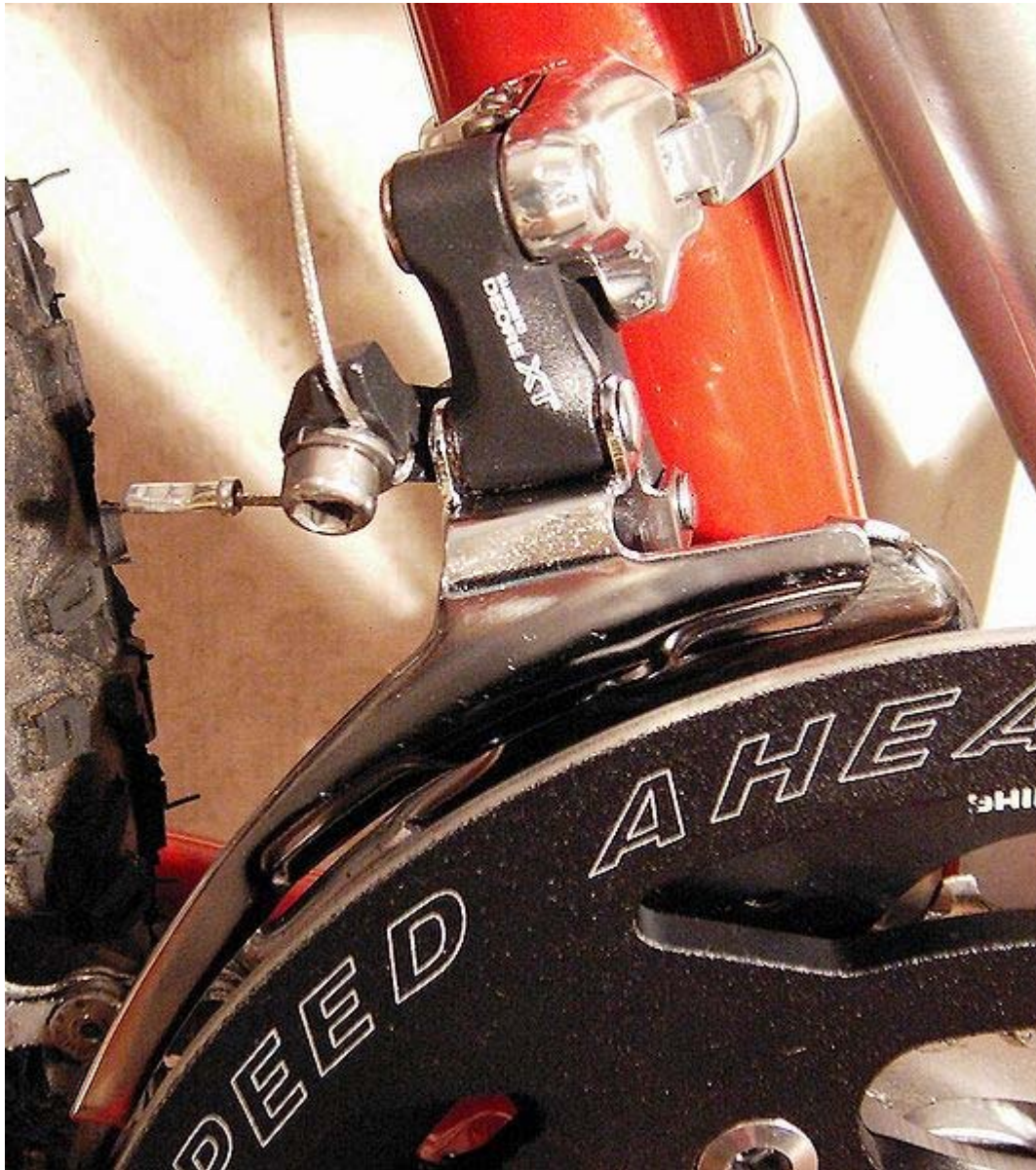
Shimano XT front derailleur (top pull, bottom swing, triple cage) on a mountain bike
