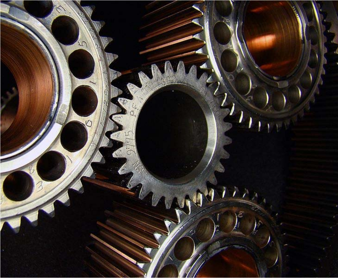
Reduction gears on Pratt & Whitney Canada PT6 gas turbine engine.
