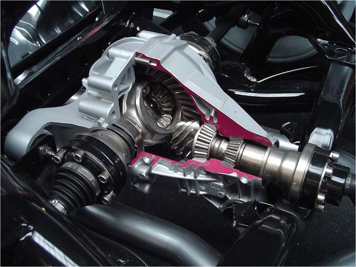
Hypoid gear in a differential
