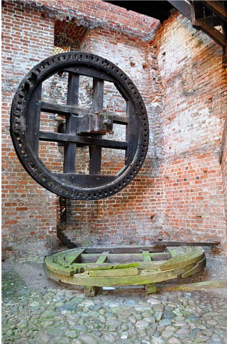
Wooden gears of a historic windmill
