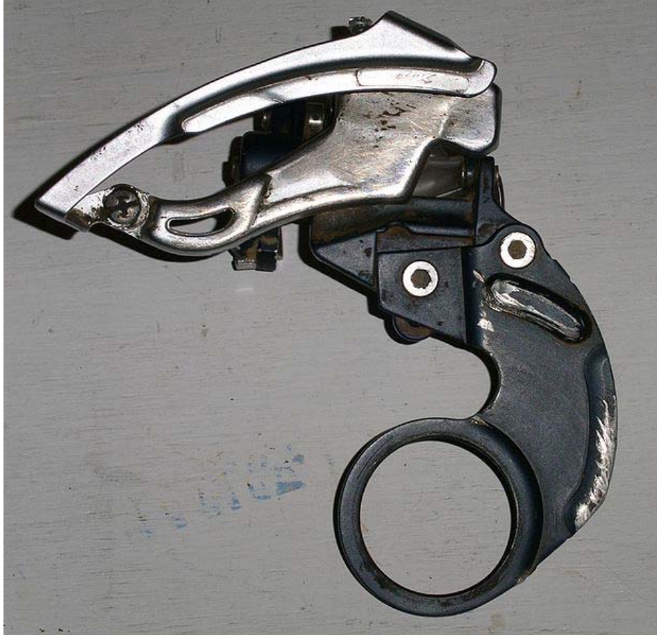
Shimano E-type front derailleur (top pull, top swing, triple cage)
