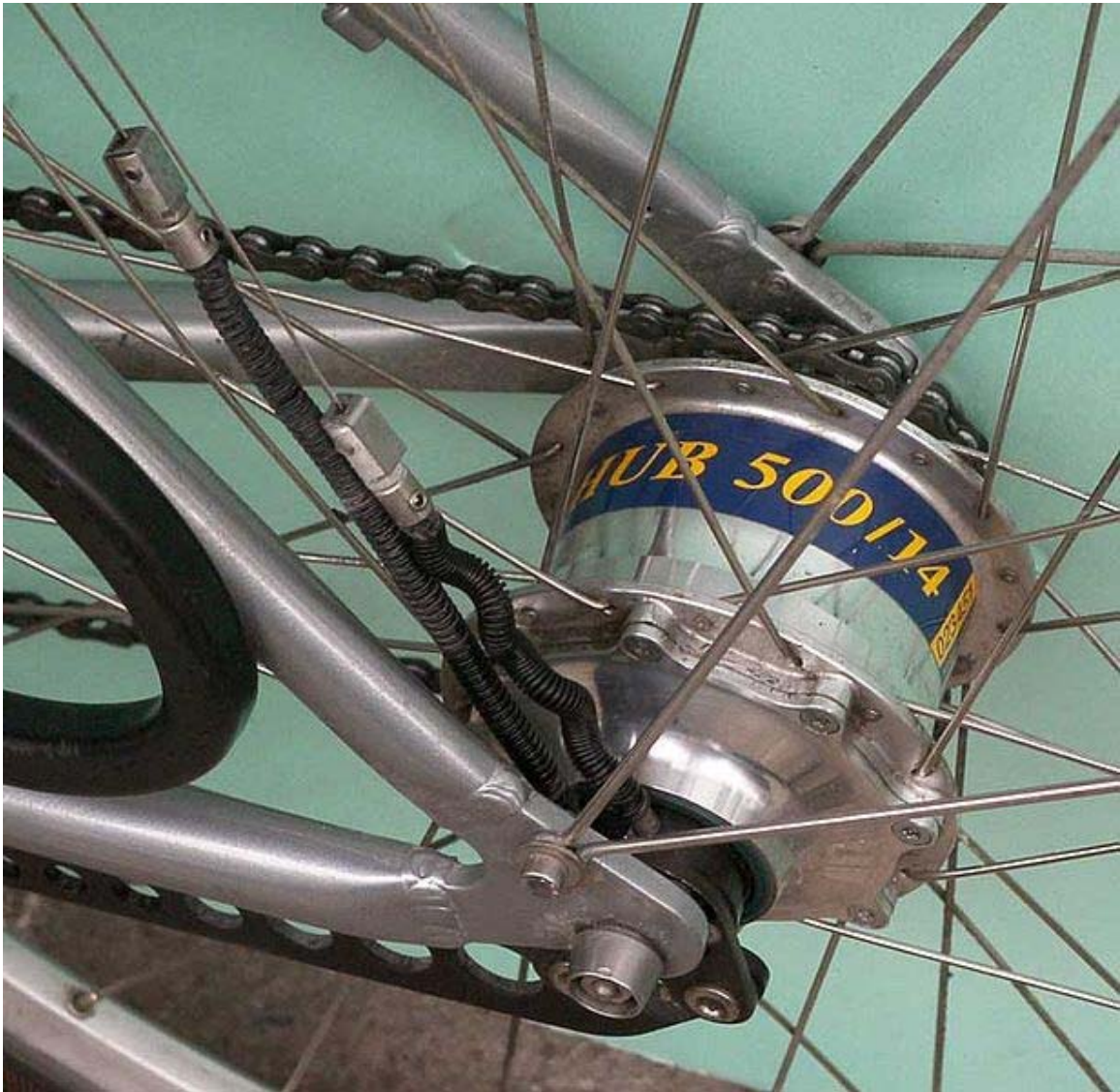
Rohloff 14 speed internally-geared rear hub
