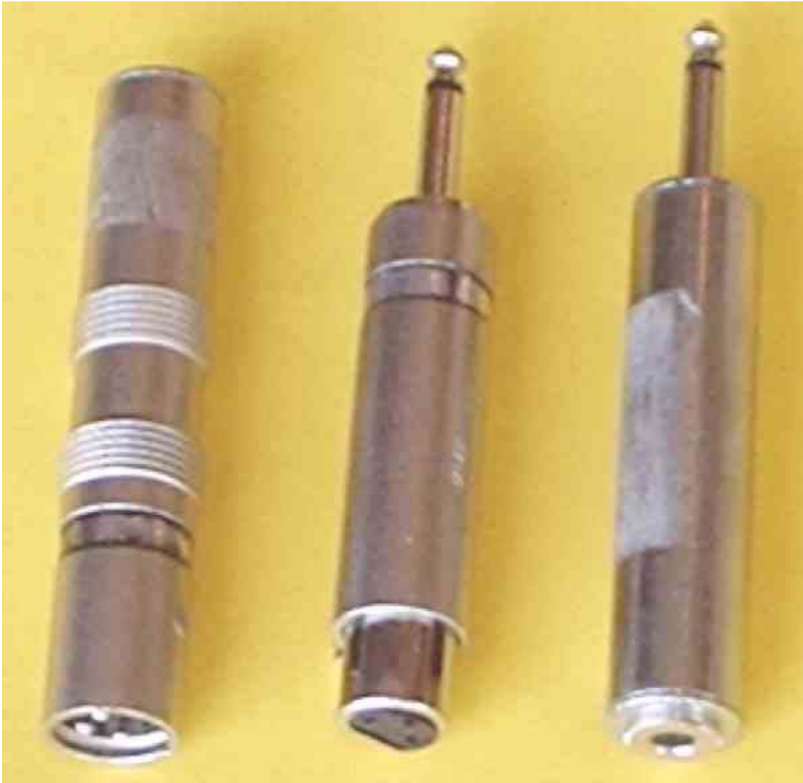
Three audio baluns (transformers).
