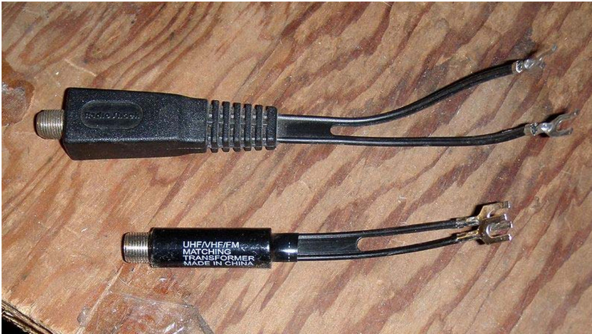
2 balun matching transformers
