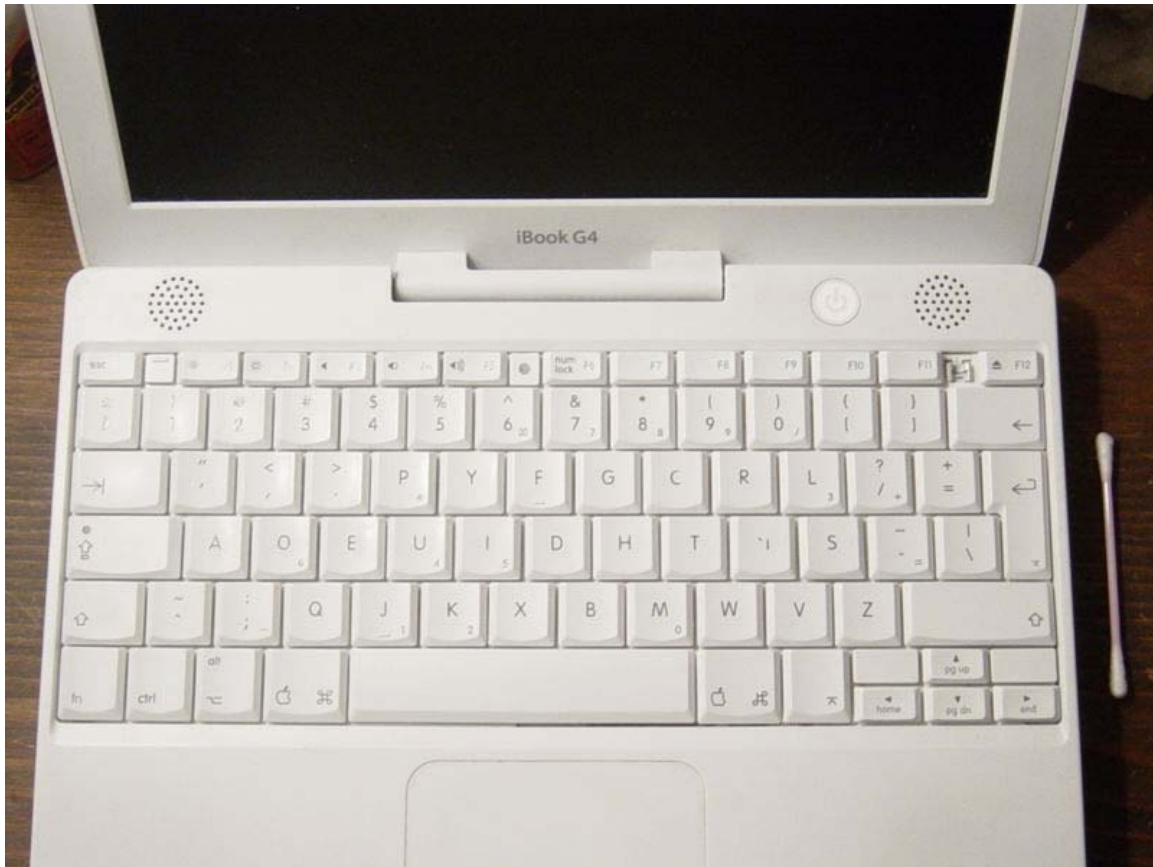
iBook with alpha and punctuation keys manually rearranged to the Dvorak layout
