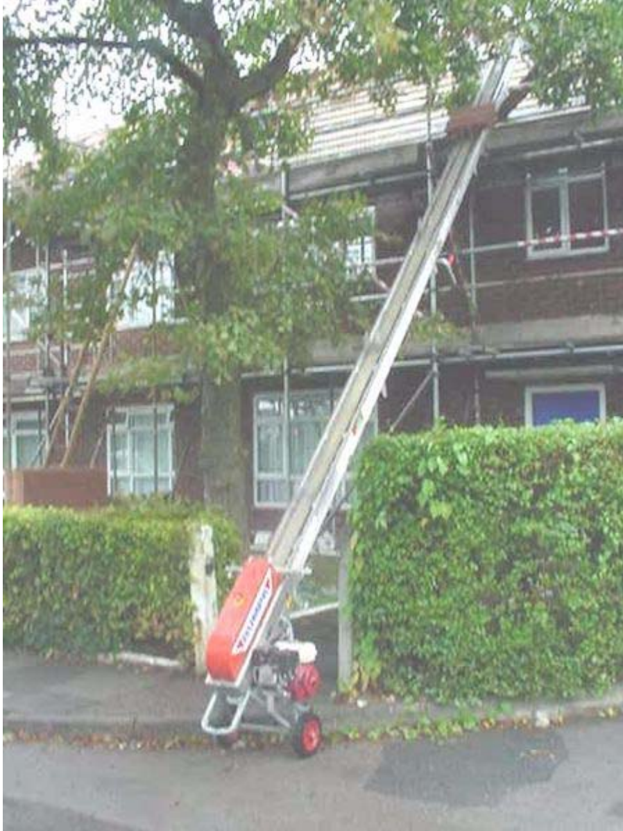
Builder's hoist, with small petrol engine
