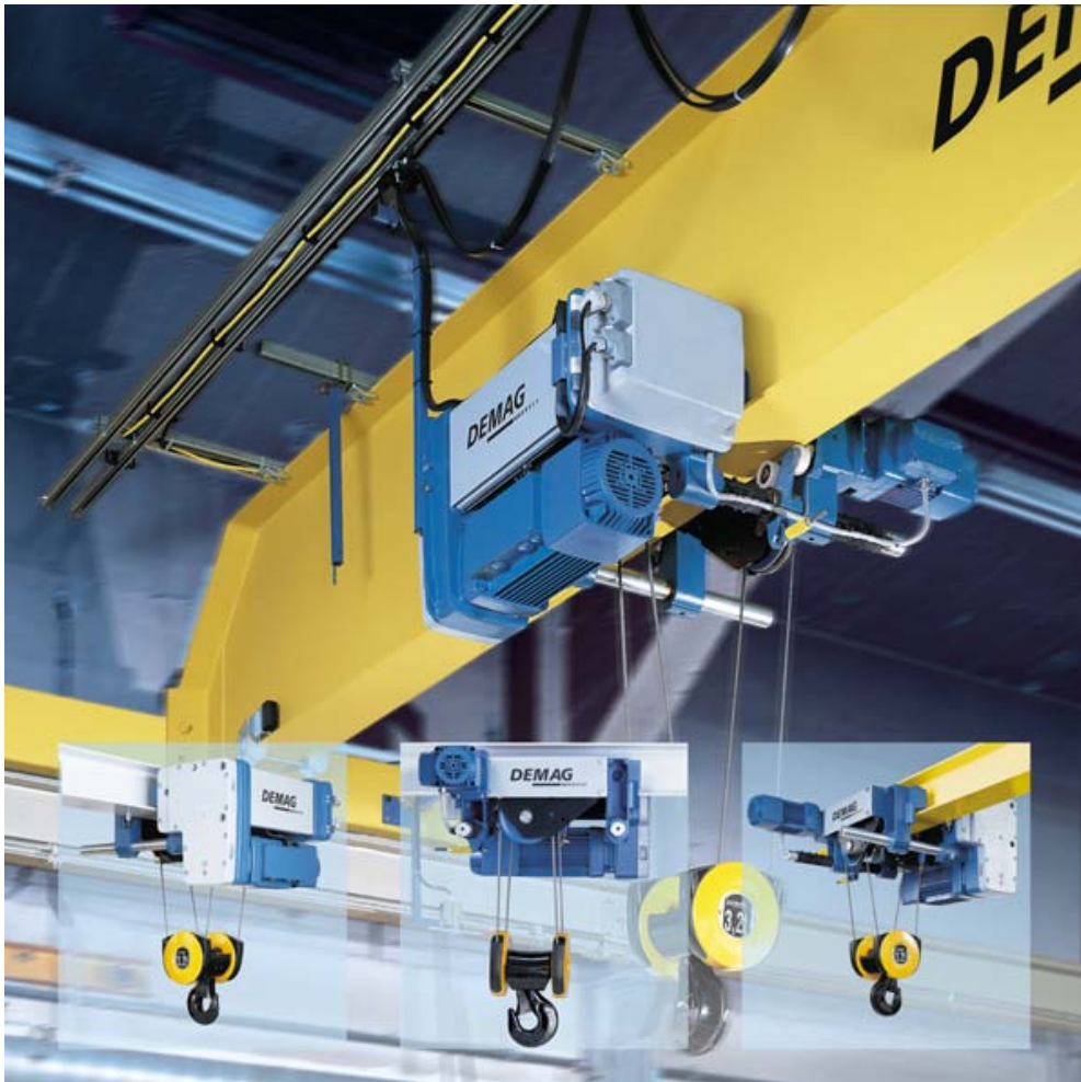
Overhead crane with a Wire Rope hoist (device) in blue suspended from bridge crane girder
