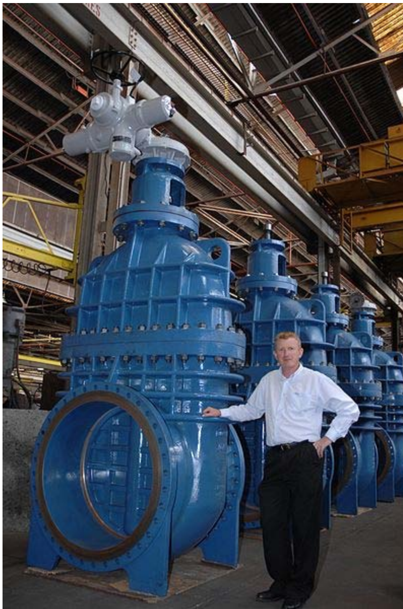
Electric multi-turn actuator on a gate valve
