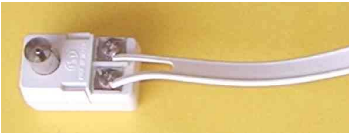
A 300-to-75-ohm balun, showing twin-lead on the right hand side
