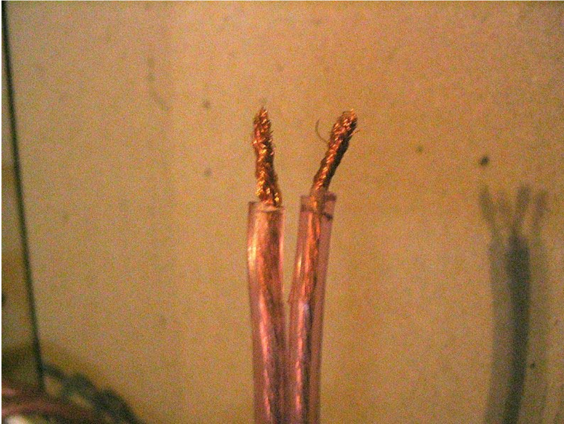
stripped speaker wires
