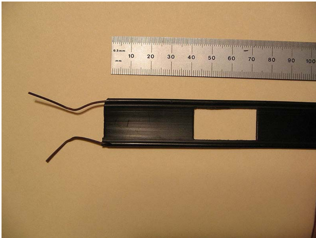
450 Ohm "Ladder line"
