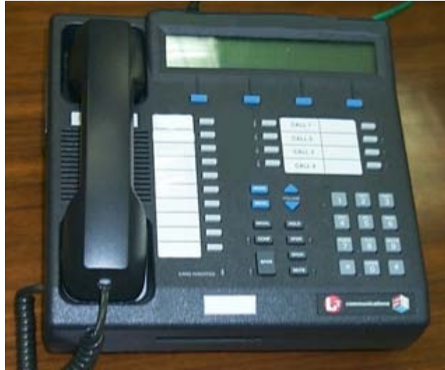
A Secure Terminal Equipment desk set. Note slot in front for Fortezza PC Card.
