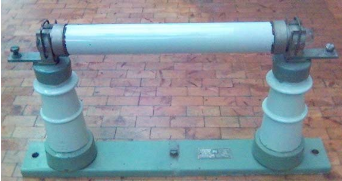
Older medium-voltage fuse for a 20 kV network
