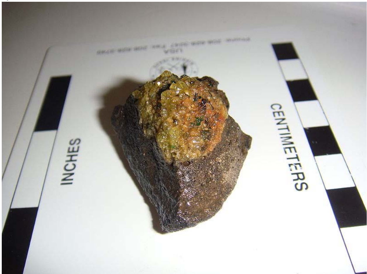
Olivine weathering to iddingsite within a mantle xenolith
