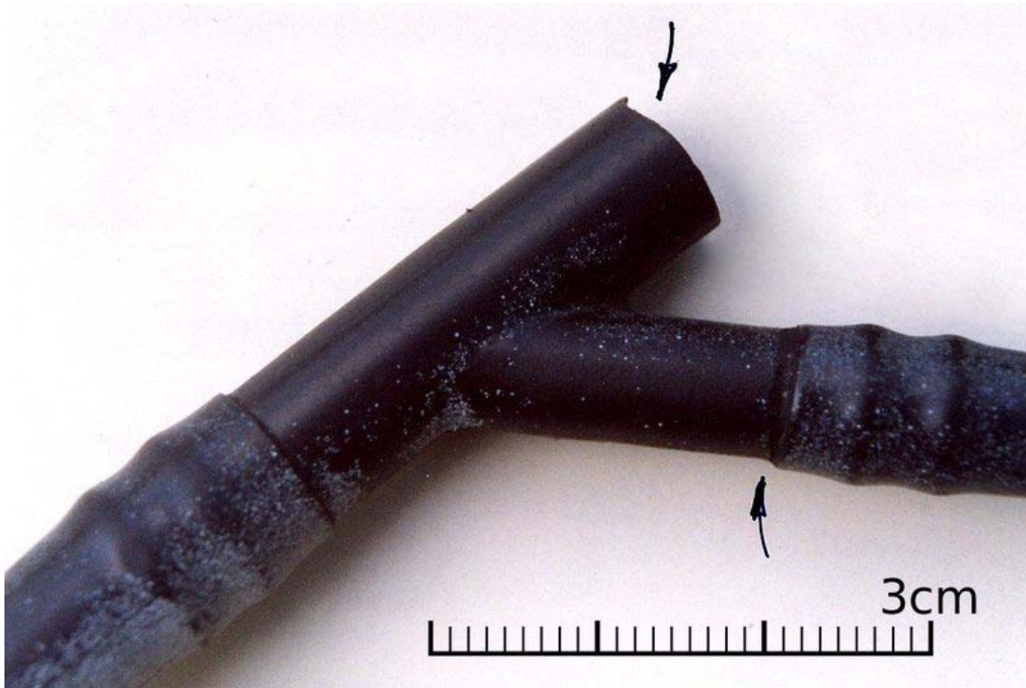
Close-up of broken fuel pipe from road traffic accident
