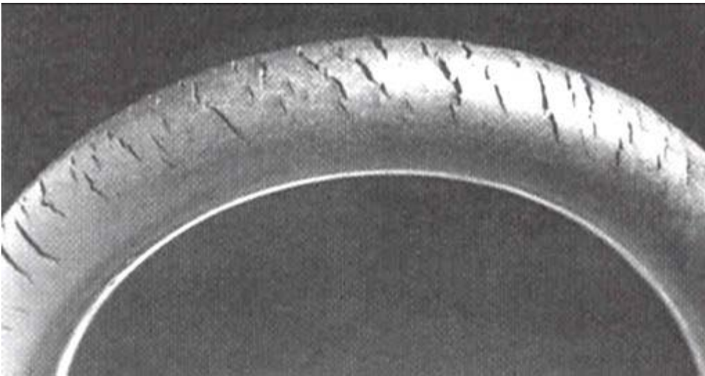
Ozone cracking in natural rubber tubing
