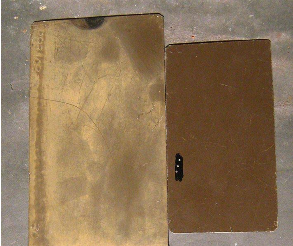
Figure 1.1: Weathered and unweathered samples of painted steel. Note the colour change.
