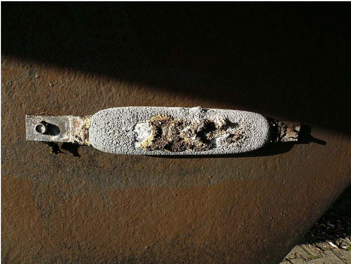
Sacrificial anode in the hull of a ship.
