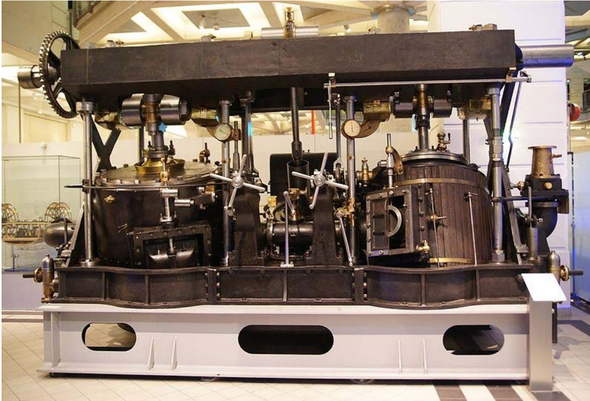
Oscillating engine built in 1853 by J. & A. Blyth of London for the Austrian paddle steamer Orsova
