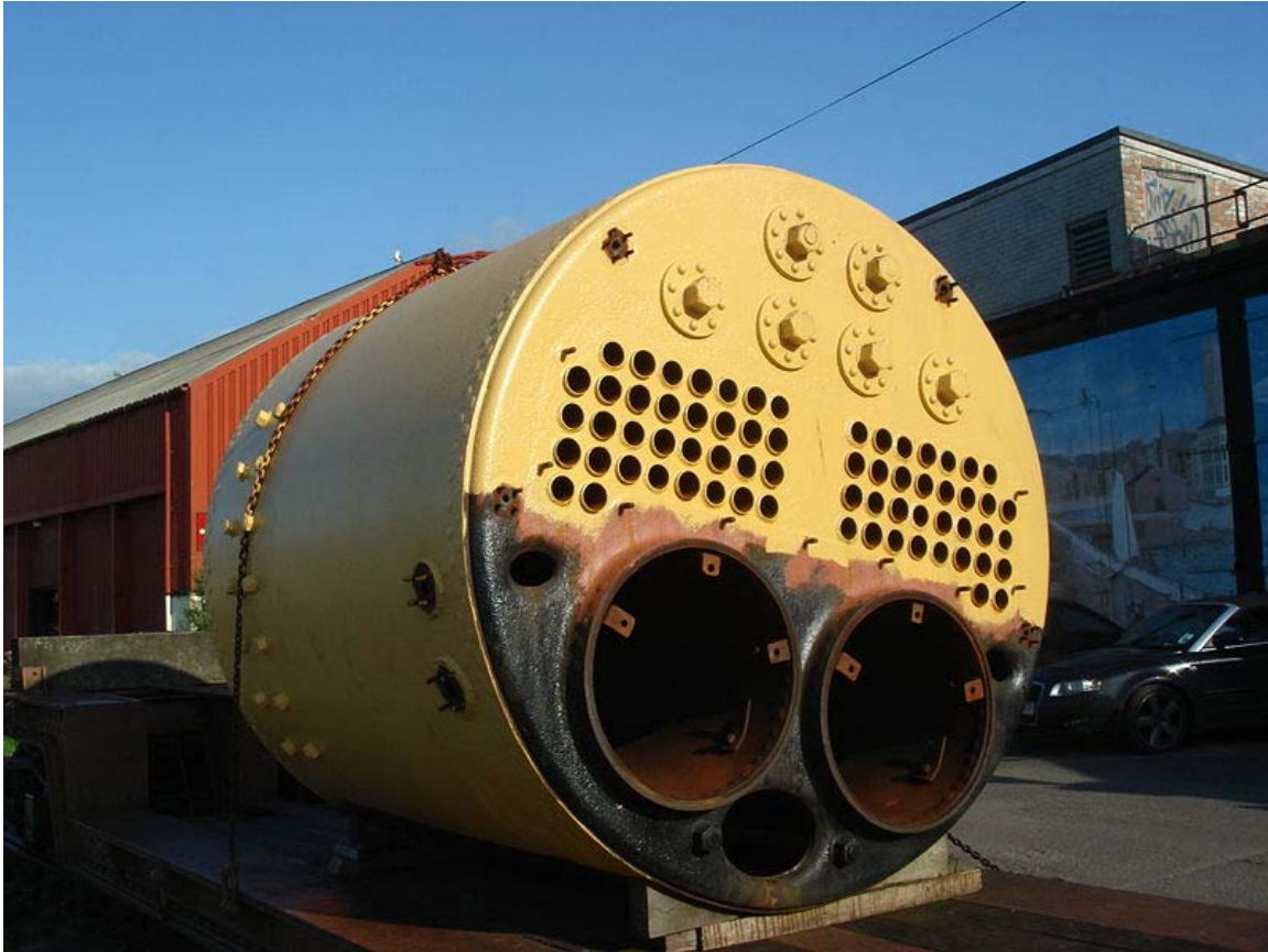
Boiler removed from steam tug Mayflower
