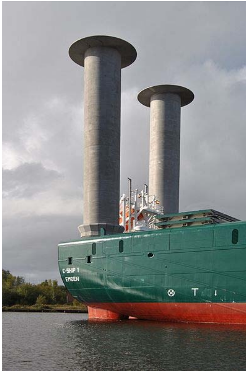
Two Flettner rotors of the E-Ship 1
