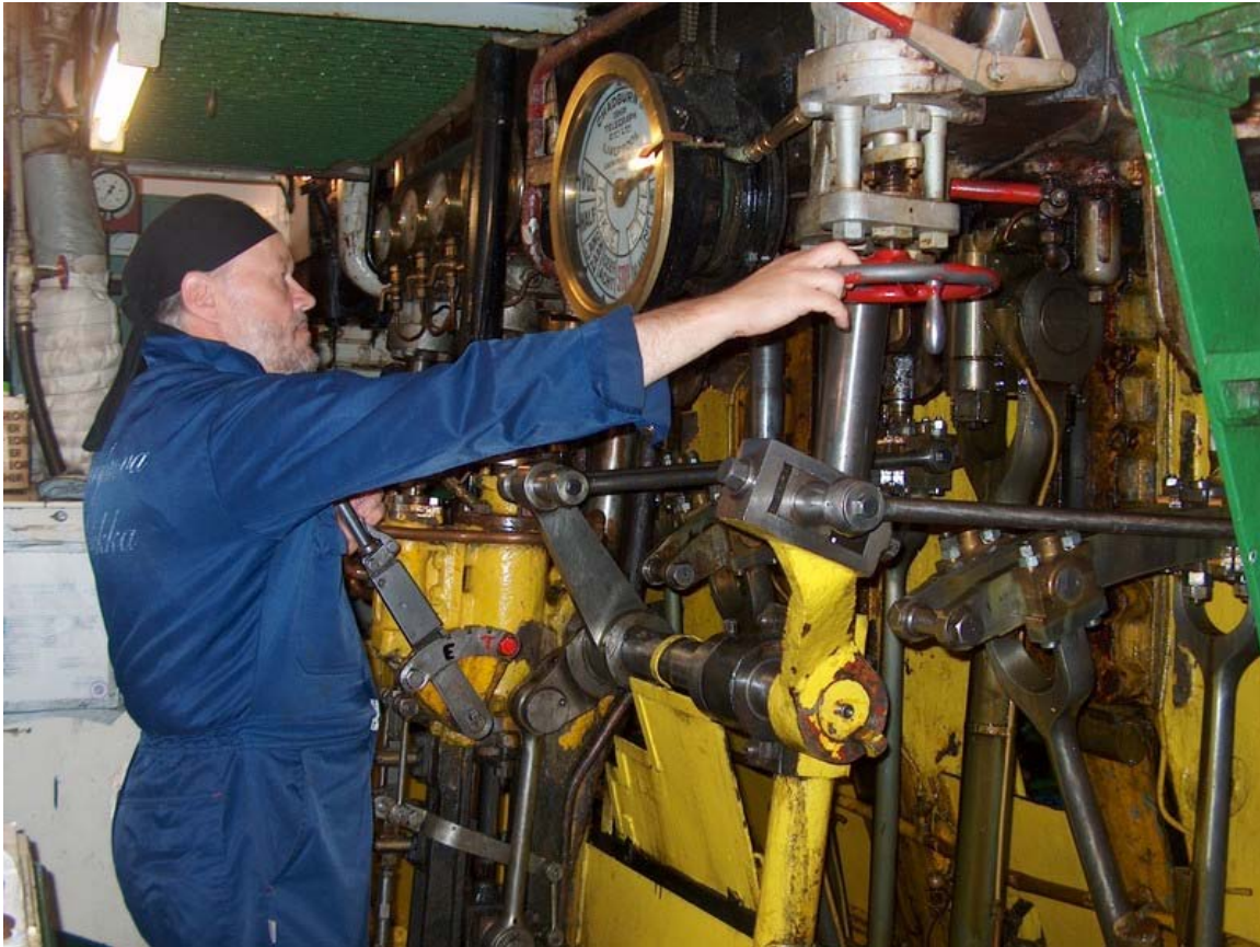
SS Ukkopekka uses a triple expansion steam engine
