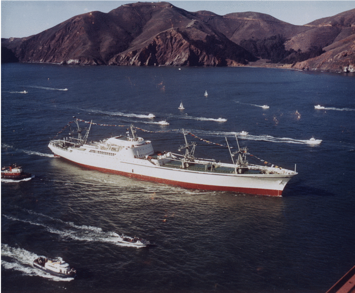
The NS Savannah was the first nuclear-powered cargo-passenger ship
