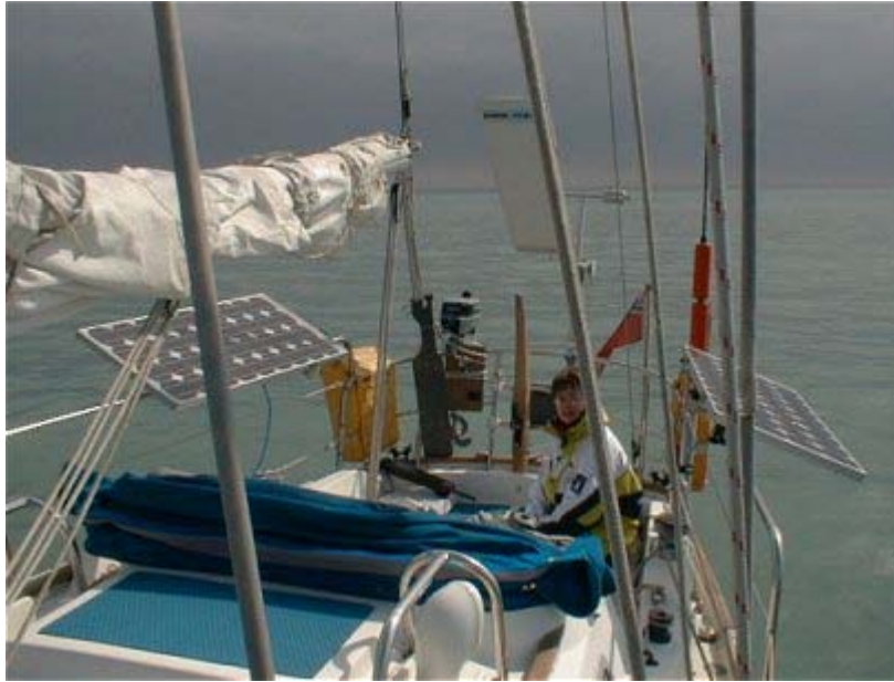
Solar panels deployed on a small yacht at sea
