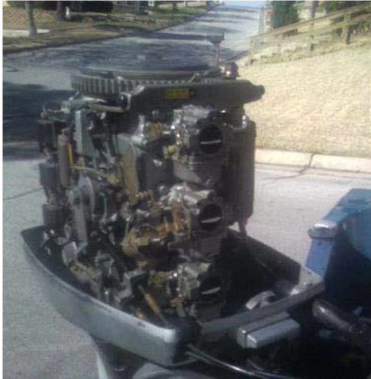
1979 Evinrude 70 HP outboard, cowling and air silencer removed, exposing its shift/throttle/spark advance linkages, flywheel, and three carburetors
