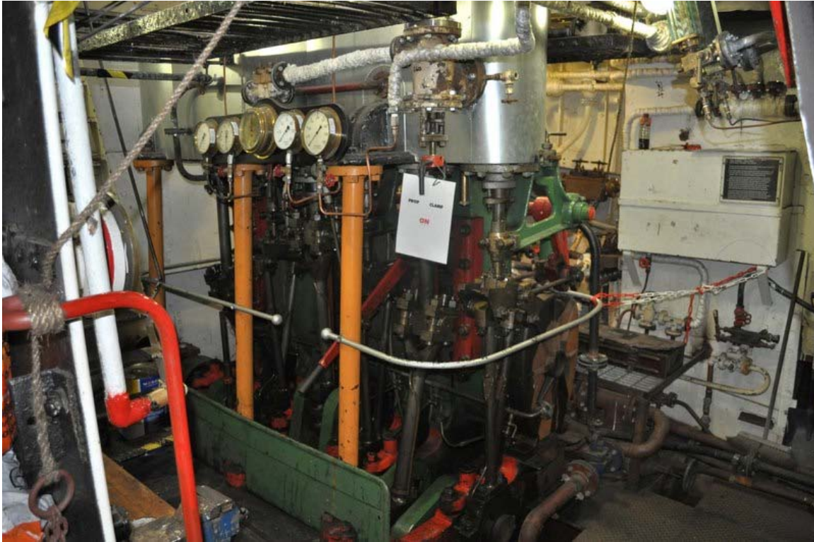
A triple expansion engine on the Lydia Eva (steam drifter)
