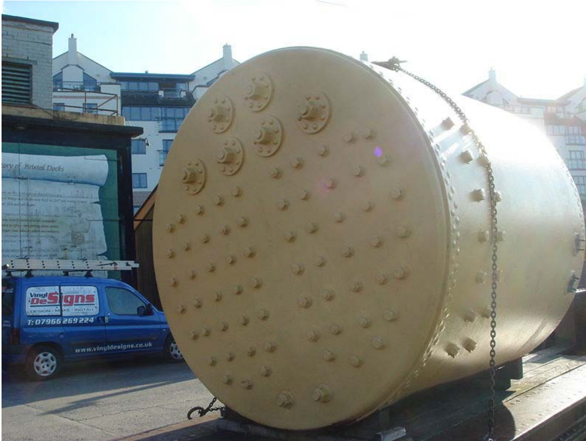
Rear face of the boiler, showing the stays supporting the combustion chambers
