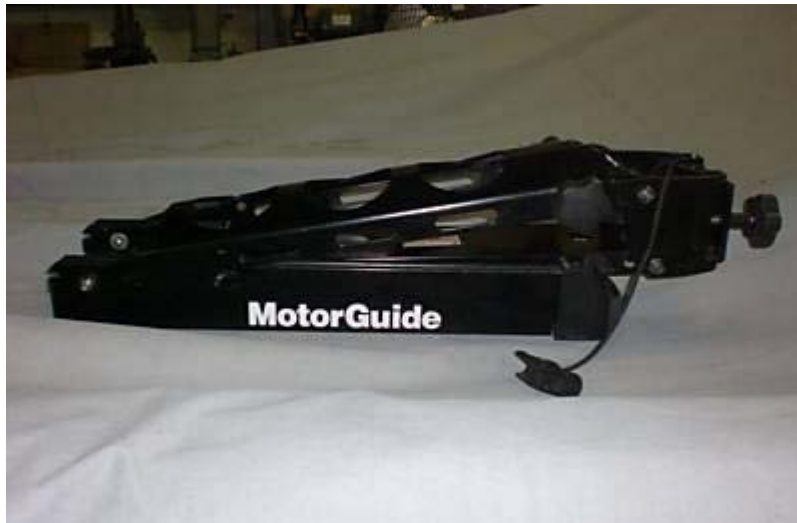
Foot controlled trolling motor mount in the deployed position.
