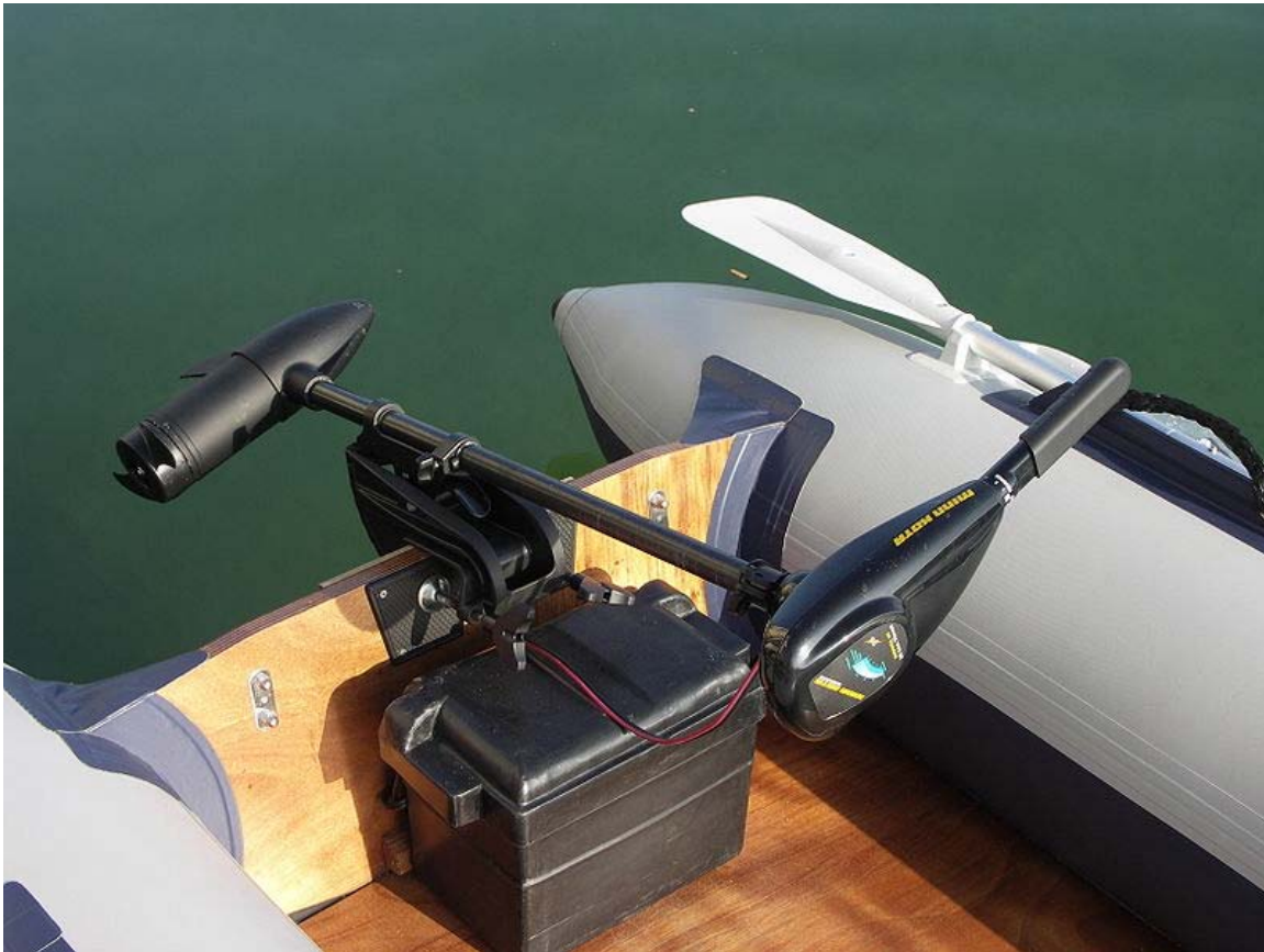
A 12 volt electric trolling motor mounted on a 8 foot inflatable boat
