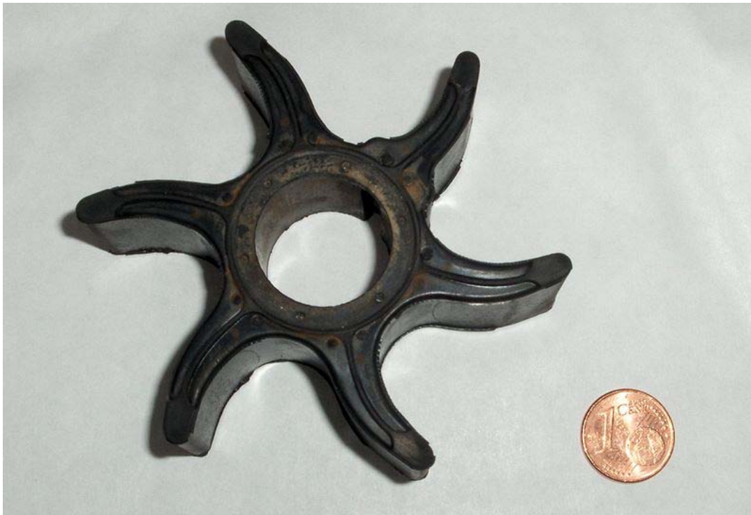
Rotor of the impeller pump (cooling system) of an outboard motor
