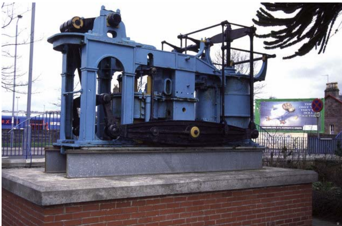
Early Napier side-lever engine from PS Leven , on display at Dumbarton, Scotland
