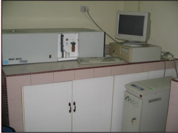
Use of emission spectrometer to analyse ^{15}\text{N} isotope in plant and soil samples
