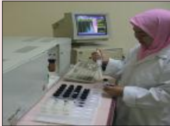
Use of emission spectrometer to analyse ^{15}\text{N} isotope in plant and soil samples
