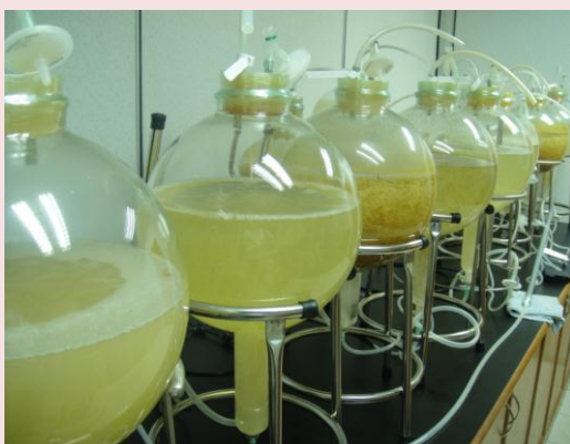
Seed-cultures in 20-litre bioreactors
