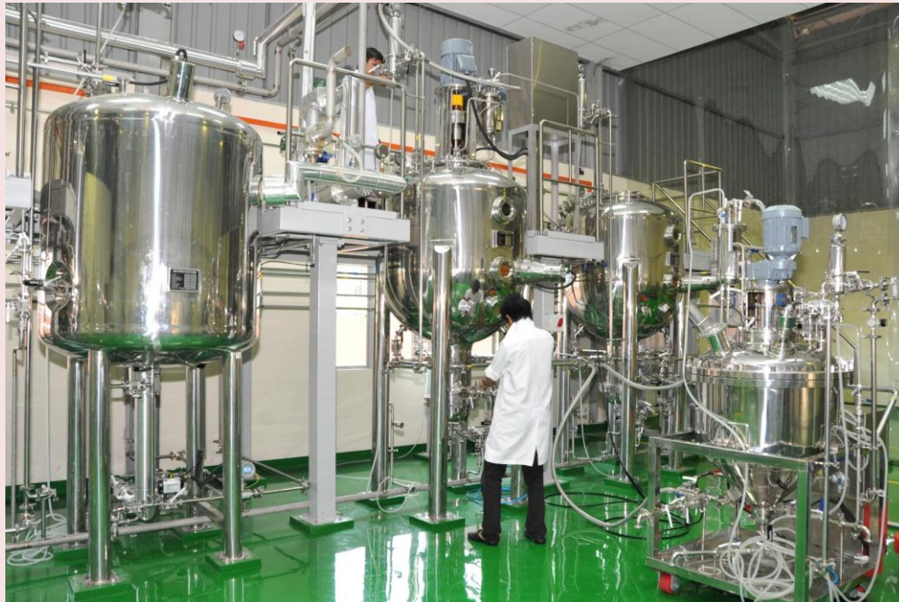
Pilot Plant of 1 ton Advanced Bioreactor System
